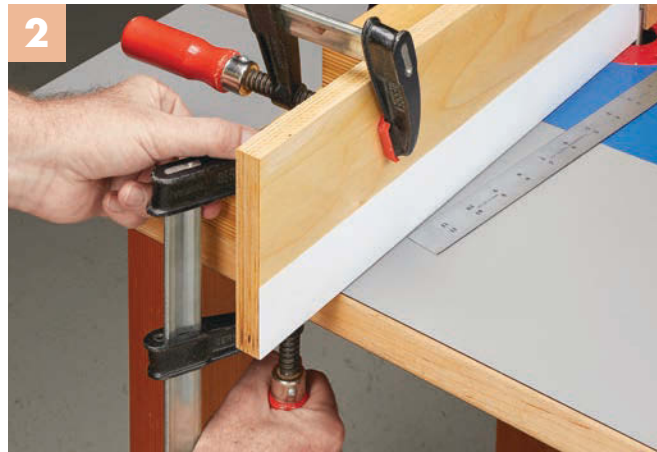
▲ After positioning the left side of the fence, carefully clamp the router fence to the table. It's a good idea to do a test cut to make sure it's not removing too much material at one time.
