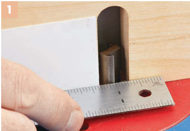
▲ With the right end of the router table fence clamped to the table, use a straightedge to swing the left side of the fence into position. The router bit should just touch the edge of the rule.
