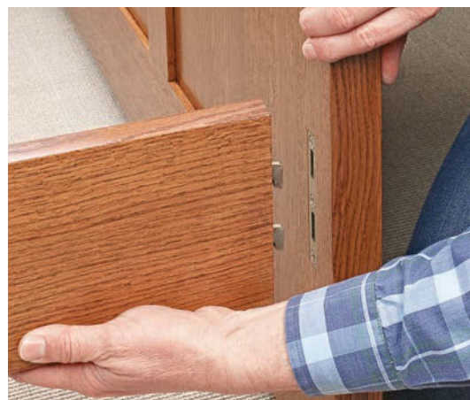
▲ Hidden fasteners are used to hold the rails to the legs. Shop Notes on page 64 has the details.
