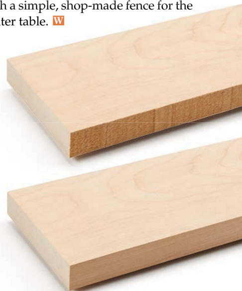
▲ Before jointing, the stock is rough (above). A couple passes using the auxiliary fence on the router table cleans it up (below).
