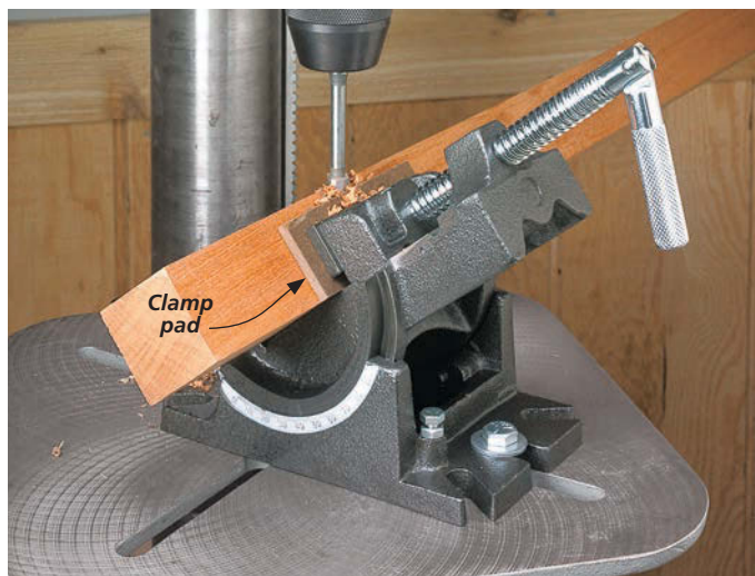
▲ An angle drill press vise provides a convenient way to drill accurate angled holes without having to go through the hassle of tilting the table of your drill press.
