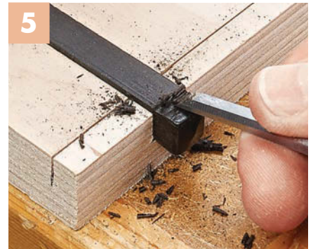
▲ Reposition the stick to slightly back-bevel each plug before cutting them free. The bevels help the plug fit tightly in the hole.
