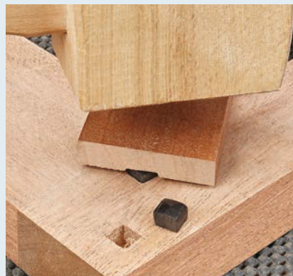
▲ A scrap of wood with a shallow groove cut near the end acts as a gauge for inserting the plugs to the proper depth.
