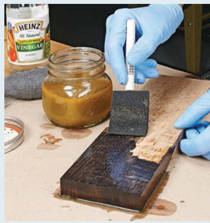
▲ Steel wool is dissolved in vinegar and brushed onto the still damp wood. The chemical reaction begins immediately.
