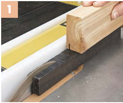
▲ Rip \frac{3}{8} "-square "sticks" of ebony to size at the table saw. Use a push block to keep your hands well away from the blade.
