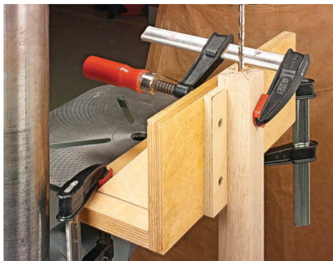
▲ A simple plywood right angle support can be clamped to your drill press table so that it just overhangs the edge. It's invaluable when drilling a hole in the end of a long workpiece.
