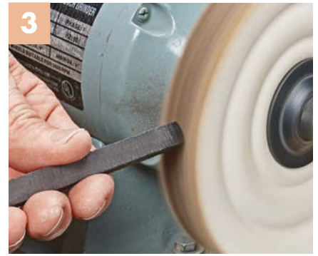
▲ When you're done crowning the end of several sticks, polish the ends on a buffing wheel to give them a burnished look.
