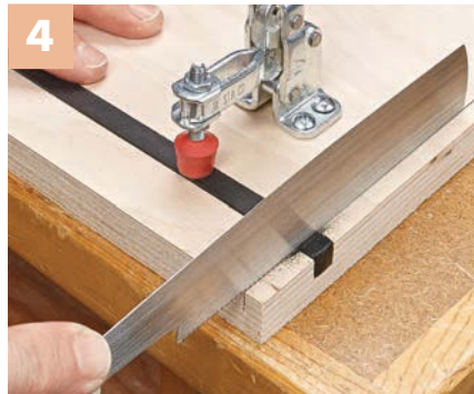
▲ Make a shallow kerf cut on all four sides of each stick. This plywood jig and clamp holds the sticks in place.
