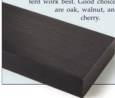
▲ A solution of 1 tsp. tannin powder and 1 cup warm water is brushed on and allowed to partially dry.
