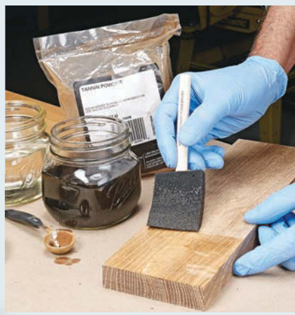
▲ A solution of 1 tsp. tannin powder and 1 cup warm water is brushed on and allowed to partially dry.
