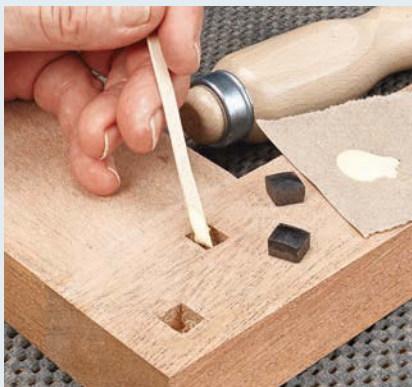
▲ Use a small applicator to apply a dab of glue in the square hole. Don't overdo it as the excess is tough to clean up.
