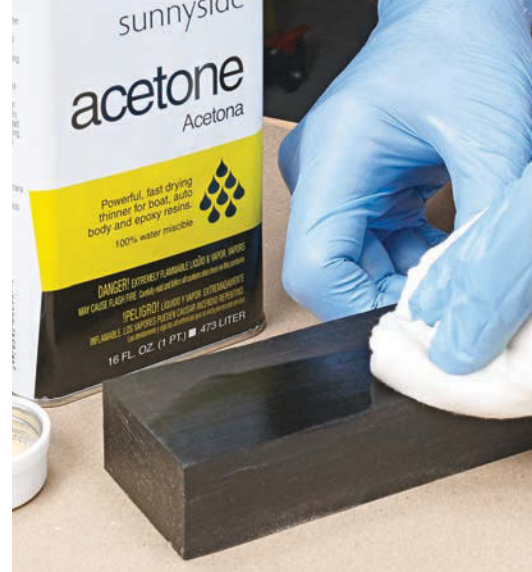
▲ Wiping ebony down with acetone or denatured alcohol prior to gluing will ensure a good bond.
