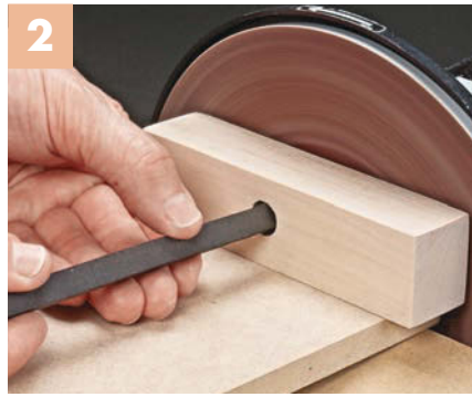
▲ After building this sanding jig (Shop Notes, page 64), crown the ends of the ebony sticks by rotating them in the hole.
