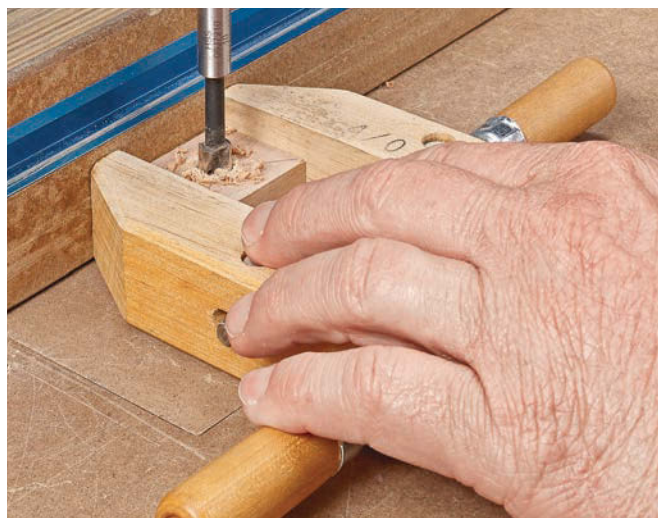
▲ When it comes to drilling holes in small workpieces, a wood handscrew makes a handy holding device. The wide, square jaws of the handscrew also register against the fence and table.
