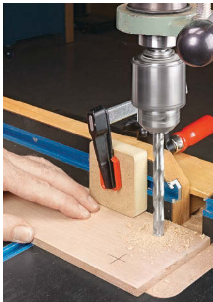
▲ By clamping a block to the fence above a workpiece, you can prevent a thin workpiece from climbing the bit.
