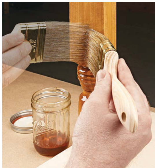
▲ An approach that works well for vertical surfaces is called cross-brushing. First, you brush back and forth across the grain, working from the bottom up (left photo). Now complete the coat by "tipping off" the surface vertically from the bottom to the top (right photo).
