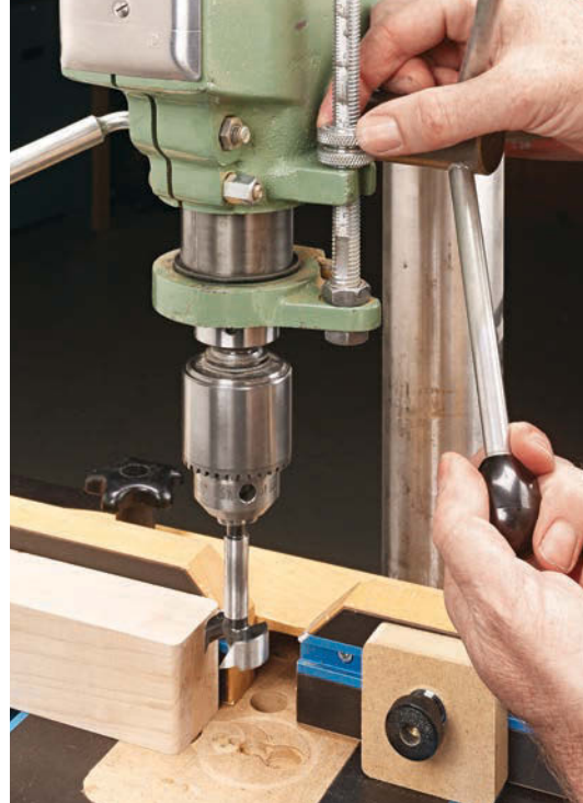
▲ All it takes is a few seconds to set the depth stop on the drill press to create consistent, accurate holes.
