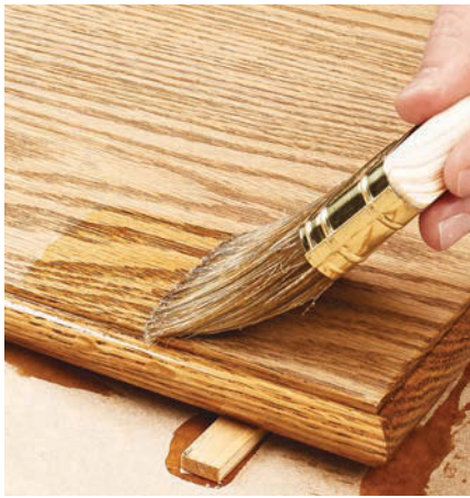
▲ By starting slightly off the edge of a panel and back-brushing carefully toward it, you can avoid runs and drips.
