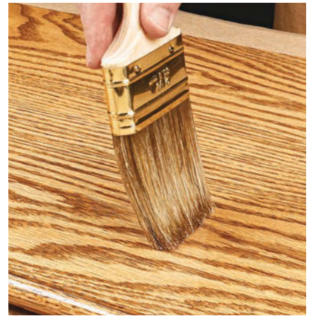
▲ After finishing the entire panel, hold the brush almost vertically in order to "tip off" the surface and make it smooth.
