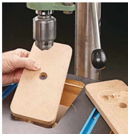
▲ Replace the insert regularly to ensure adequate workpiece support for drilling tearout-free holes every time.
