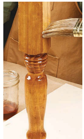
▲ An approach that works well for vertical surfaces is called cross-brushing. First, you brush back and forth across the grain, working from the bottom up (left photo). Now complete the coat by "tipping off" the surface vertically from the bottom to the top (right photo).
