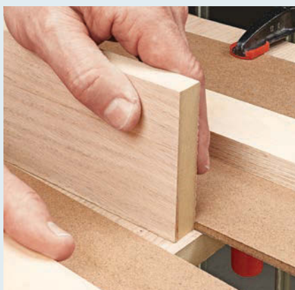
▲ Next, use a scrap of the material that will go into the dado to position the second guide. Then clamp that guide in place.
