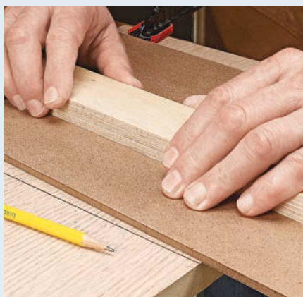
▲ After laying out one edge of the dado using a pencil, clamp the first straightedge guide tightly against the layout line.
