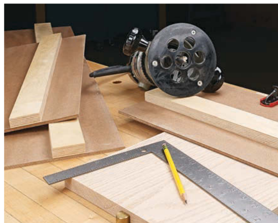
▲ I like to make several guides, such as the 28" and 54" ones shown, for various cutting and routing operations.
