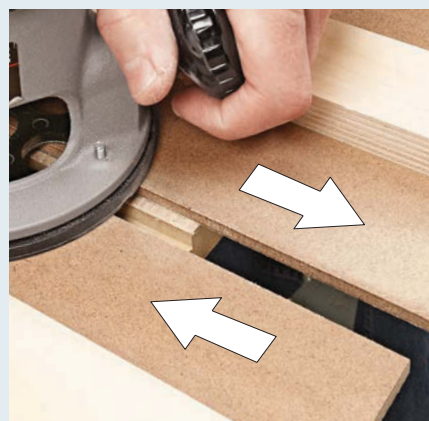
▲ Complete the custom-size dado by routing against the fence of one guide (shown) and back down the other guide.
