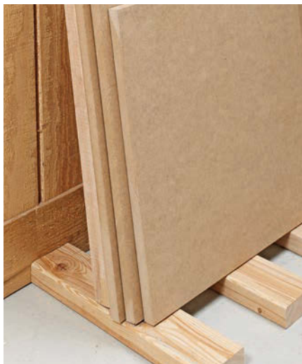
▲ Raising sheets off the floor prevents moisture from wicking up. To keep panels flat, support them against thick boards.
