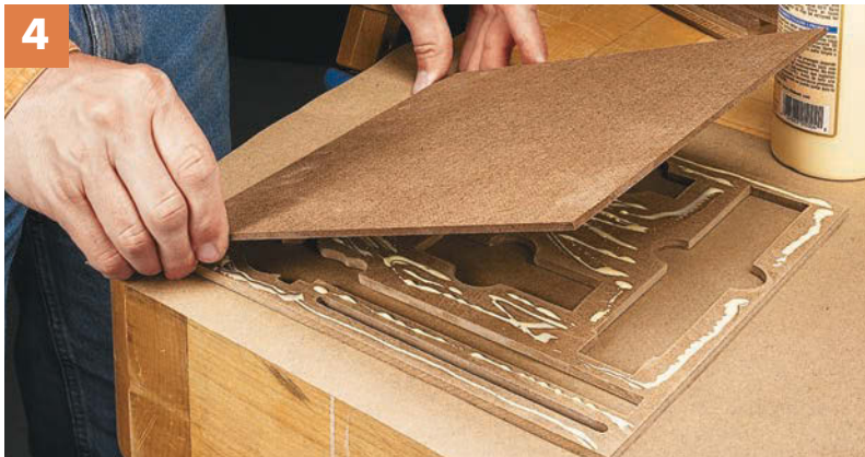
▲ A separate hardboard base forms the bottom of the insert. You can simply cut it to match the size of the insert top and then glue it in place. Apply glue sparingly to reduce the amount that squeezes out into the tool pockets.
