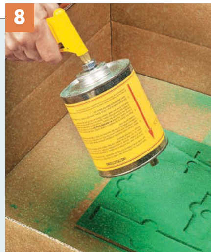
Spray the Flocking Heavily. Place the insert in a cardboard box to contain the overspray of flocking material.
