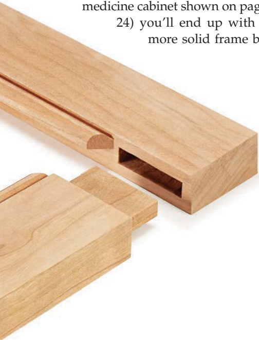
1 Route the Profile. With the router bit bearing flush with the face of the fence, pass the stiles and rails across.
