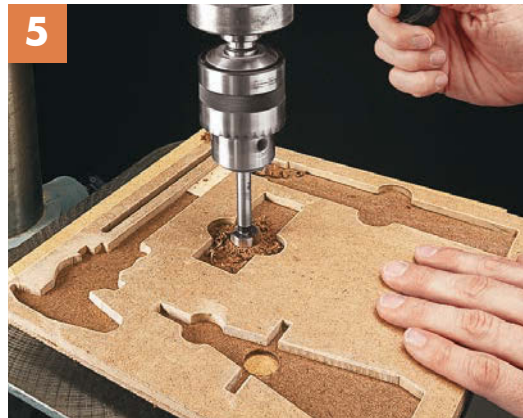
▲ Depending on the shape of your tools, you may need to drill relief holes in the base to provide clearance for parts that extend below the body.
