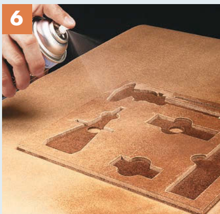
Seal the Insert. A couple of coats of spray lacquer or shellac create a smooth surface for the adhesive.
