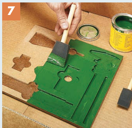
Apply Adhesive. A foam brush allows you to apply adhesive to the surface, as well as the nooks and crannies.
