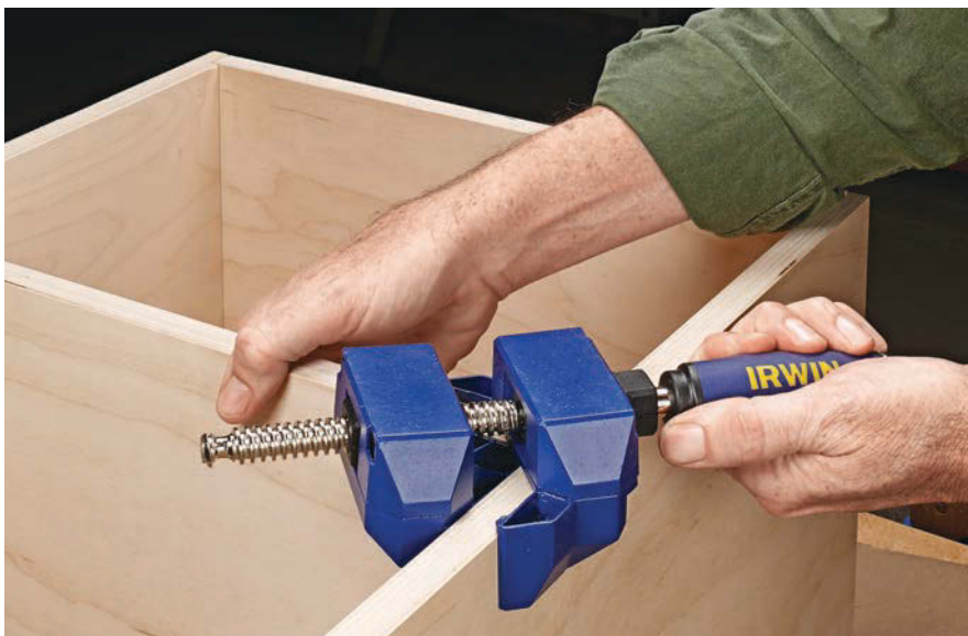
▲ Both the Bessey and Irwin angle clamps feature openings near the base of the clamp where the outer jaws come together. This simple addition to the clamps allows them to clamp T-joints, which is handy when adding shelves to case assemblies.
