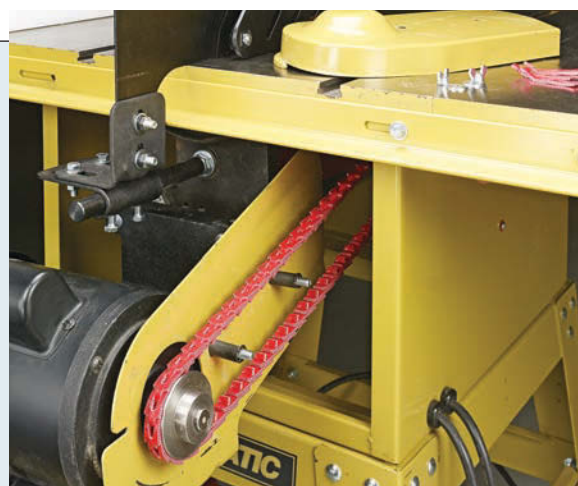
▲ Machined steel pulleys tend to run more smoothly than standard die-cast versions, and a link belt is easy to customize in length to fit your model of saw.
