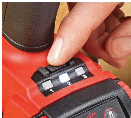
▲ Tools with brushless motors usually have lithium-ion batteries and other special features, like the push-button speed control on the Milwaukee impact driver.
