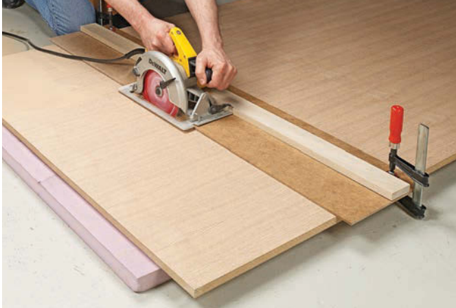
▲ This shop-built straightedge guide works well for crosscutting. Trimming the edges of the foam leaves room for the clamps.
