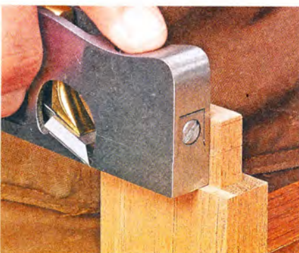
▲ A shoulder plane makes quick work of removing saw marks on cheeks and stepped shoulders.
