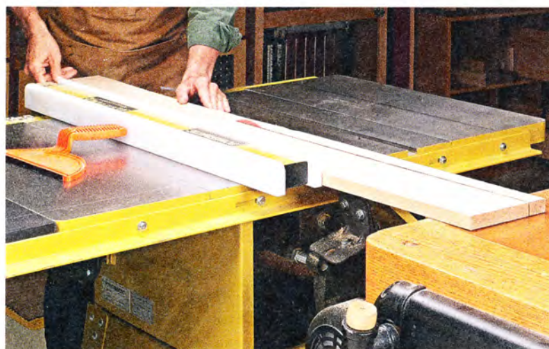
▲ Outfeed support is crucial when ripping long workpieces. One way to support the workpiece is to make your bench or other worktable the same height as your table saw.
