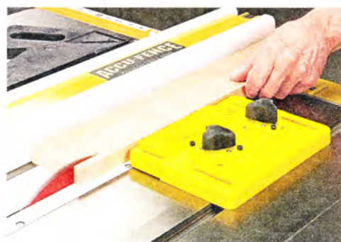
▲ A magnetic featherboard is easy to set up. Just put it in place and twist the knobs to engage the magnets.
