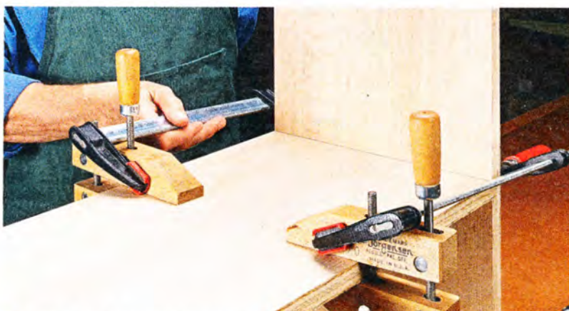
▲ For a wide assembly where your clamps don't have enough reach, attach handscrews to the dividers. Then clamp across the sides and the handscrews to draw the assembly together.
