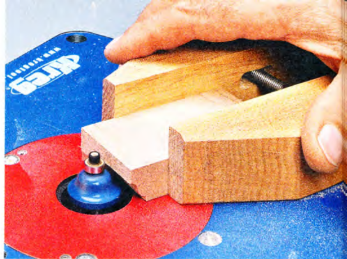
▲ Handscrews are great for machining small parts, thanks to the wood jaws.
