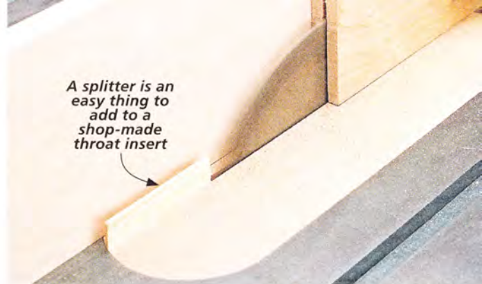
▲ A riving knife (left) or a splitter (above) prevents the kerf from closing up and causing kickback.
