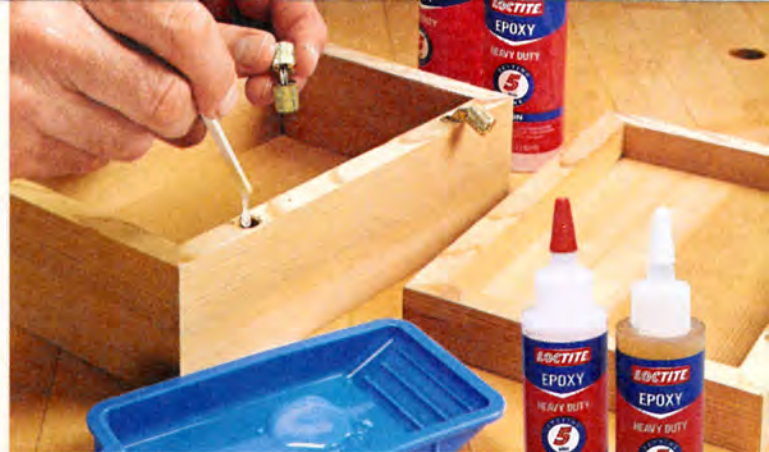
▲ A small dollop of epoxy in the hole bonds the barrel hinge to the wood for this small box project.
