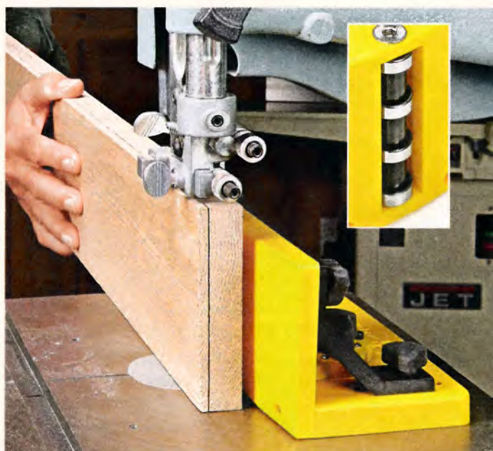
▲ The Magswitch Resaw Guide's single-point fence relies on four bearings to help the workpiece slide smoothly through the blade.
