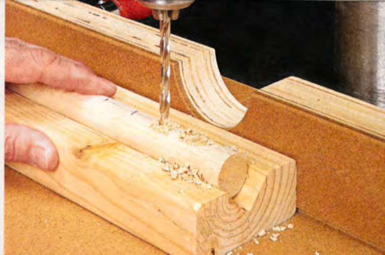
▲ Cut a \frac{3}{4} "-deep V-groove in the face of a 2x4 scrap, and you'll have the perfect holder when drilling holes in dowels, round table legs, or pipes.
