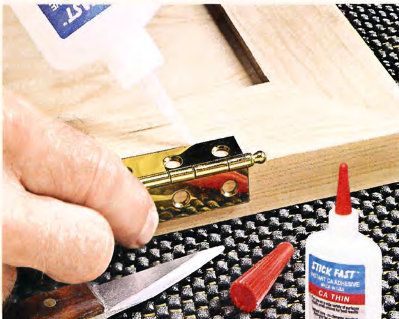
▲ A drop of cyanoacrylate will temporarily bond a metal hinge to a wood frame while you scribe the outline with a marking knife.
