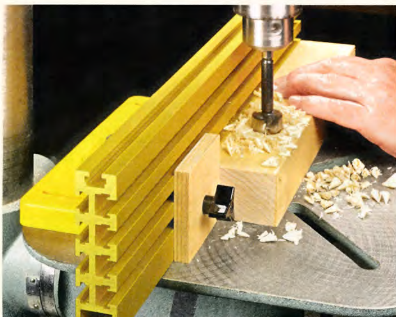
▲ This anodized aluminum fence features four T-slots and attaches to the magnetic base. The ease with which you can move and lock it down makes it a great drill press fence.
