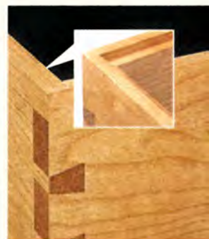
▲ Mitered shoulder dovetails allow for a seamless profile (top) or a rabbet (bottom) on the mitered edge.
