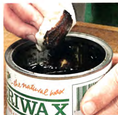
▲ A coat of tinted paste wax will hide minor scratches and restore an even sheen.
