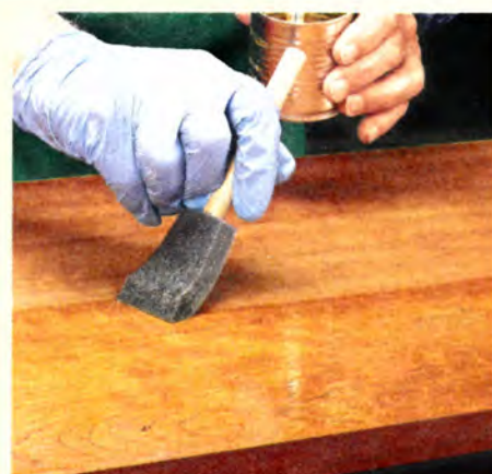
▲ The final step is to apply a coat of the original finish. Sometimes, a second coat may be necessary.
