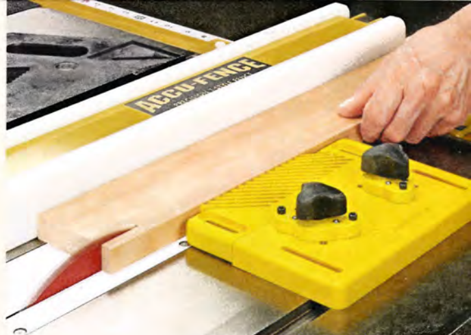
▲ A magnetic featherboard can be placed anywhere on the saw table for safer rip cuts.
