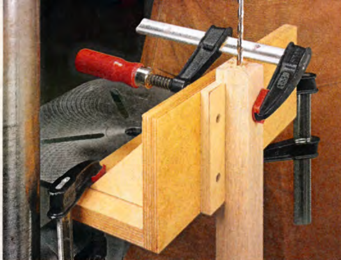
▲ This right-angle support makes it easy to drill holes in the end of a workpiece or the edge of a panel. Swing the drill press table to align the workpiece with the bit.
