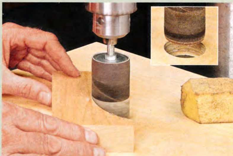
▲ Your drill press can do a lot more than just make holes. Outfit it with a spindle sanding drum attachment and an auxiliary table (inset) to smooth the edges of curved workpieces.
