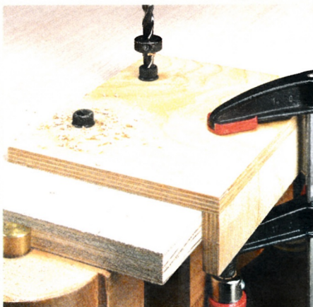
▲ The Dowelmax distance gauge lets you create evenly spaced holes along the edges of boards for assembling a panel.
