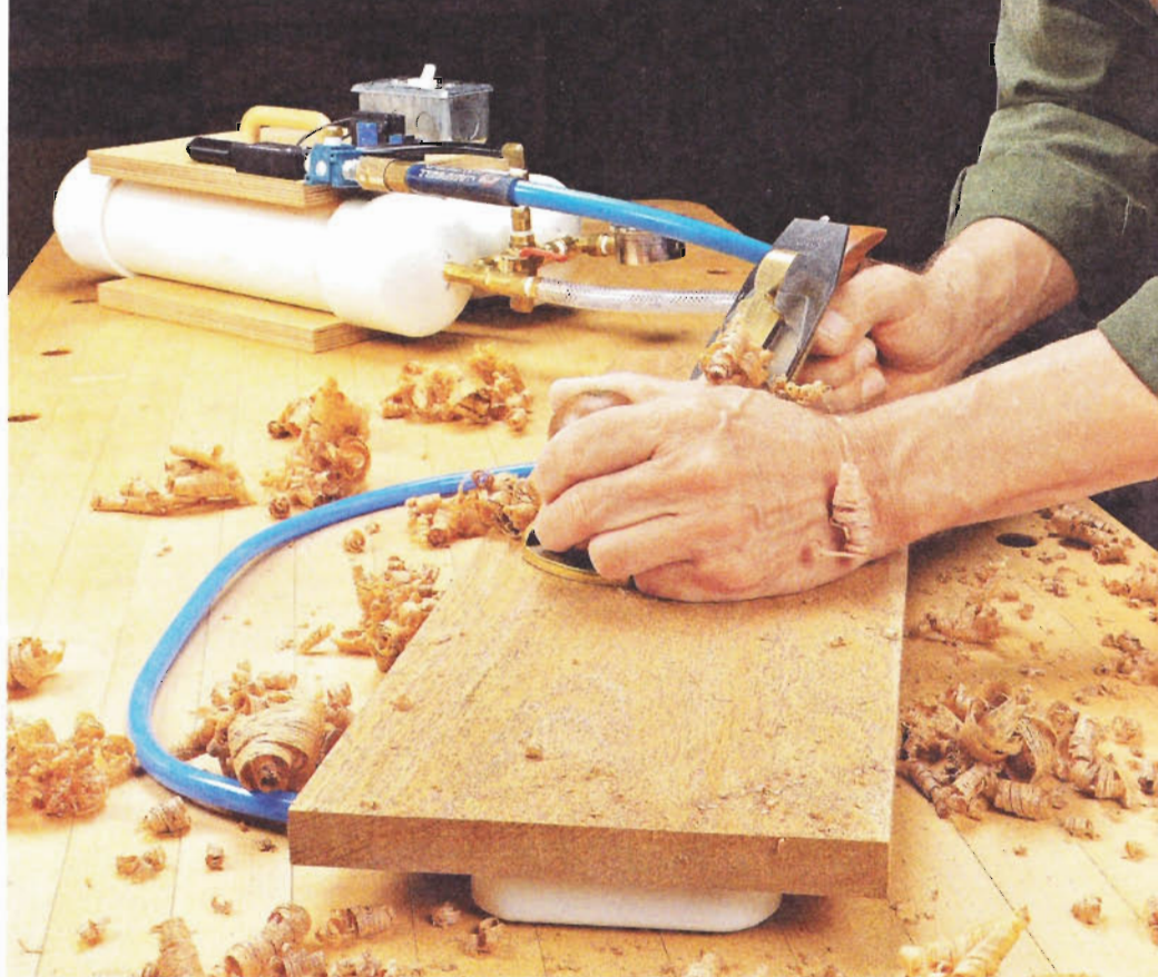
▲ Vacuum clamps grip the bench and the workpiece. All it takes is a tap on the footswitch to position or move a workpiece.
