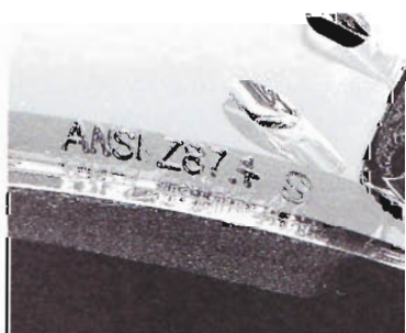
▲ The ANSI Z87+ mark shows the glasses can protect against high-impact accidents.
