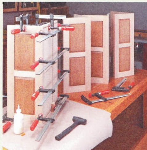
▲ When assembling the sides and backs, make sure to keep each section square as you add clamps.
