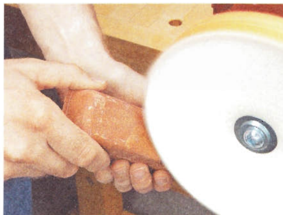
▶ All it takes is a light touch of the bar to charge the wheel with abrasive compound.
