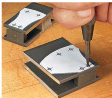
Center Punch. A punch is an easy way to locate points to drill and countersink holes for rivets.
