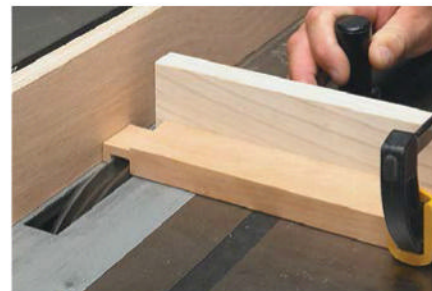
Tenon Shoulder. To define the length of the tenon, butt the workpiece against an auxiliary fence, then make a pass.
