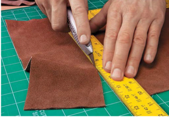
Cutting Leather. A framing square guides a sharp utility knife as you cut through the leather in one pass.
