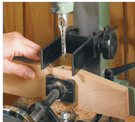
Making Mortises. A mortising machine and a 1/4" square chisel and bit make quick work of cutting the mortises.
