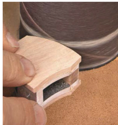
Shaping the Veneer. After gluing on the veneer, the sanding drum quickly trims it flush.
