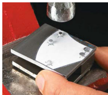
Drill & Rivet. Peening the aluminum rivets is an easy task and locks the assembly together.
