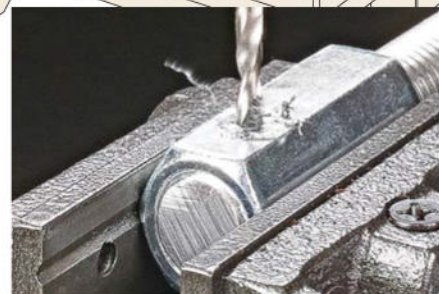
Clamp & Drill. A drill press vise holds the rod assembly securely while drilling the through holes for the pins.
