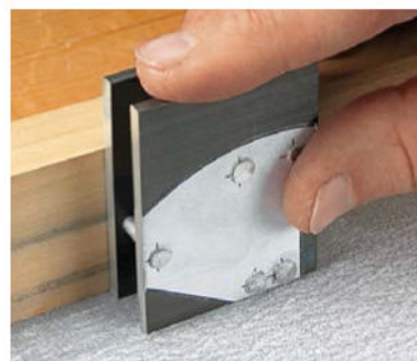
Sanding Smooth. Smooth the bottom square after sanding the rivets flush on one side.
