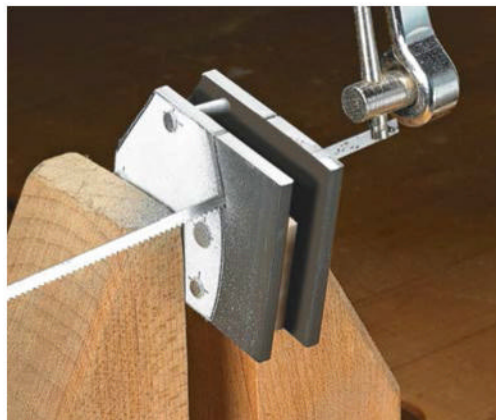
Cut To Shape. Begin by rough-cutting out the shape of the head assemblies. I found a coping saw works well to make these cuts.
