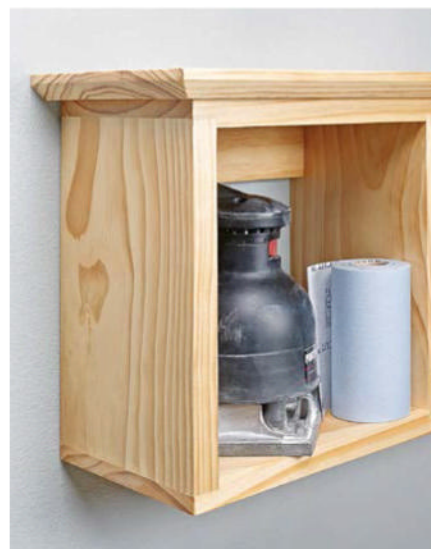
Wall Shelf. Rabbits and dados make building this shelf a quick and easy task.
