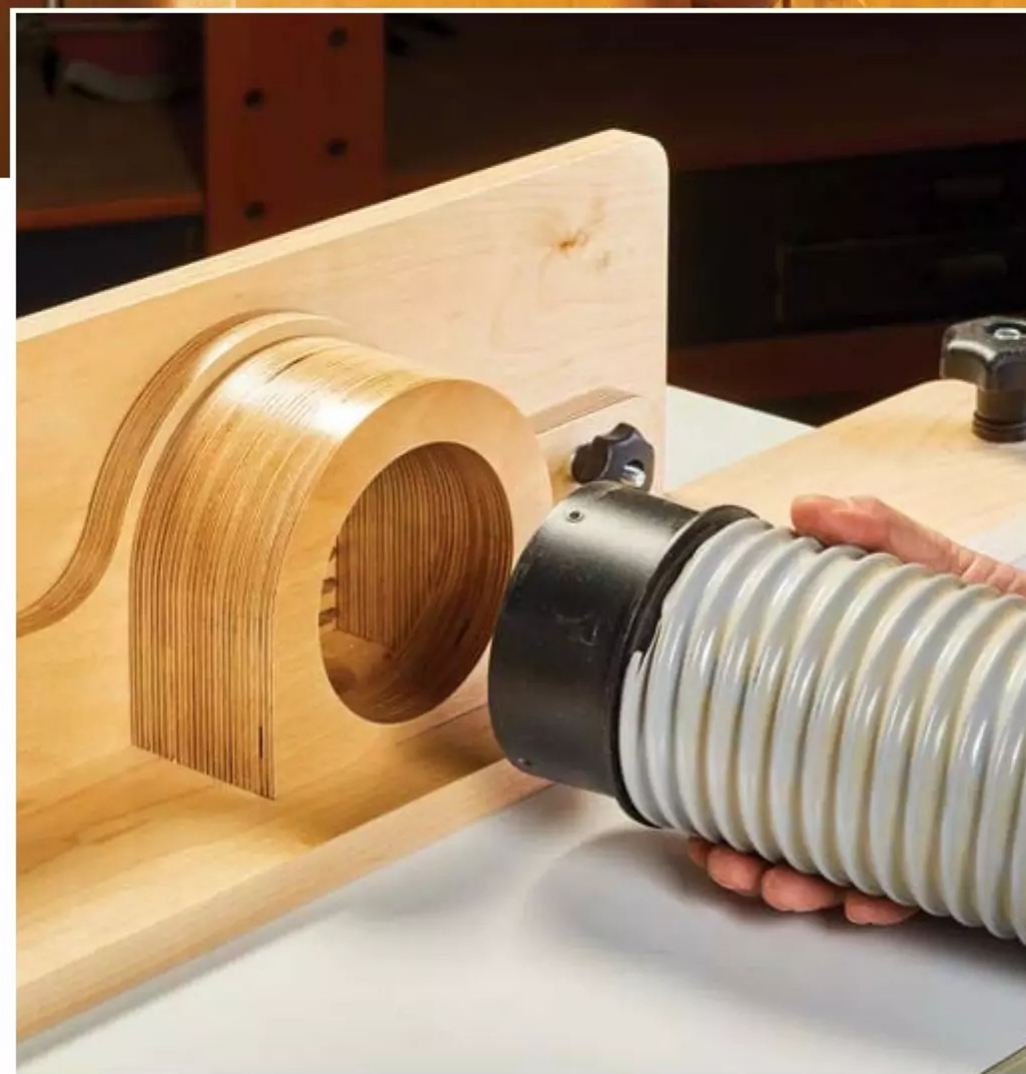
Collection Coupler. A couple of shop-made hose collars on the back side of the fence allow you to attach your dust collection directly for debris-free routing.
