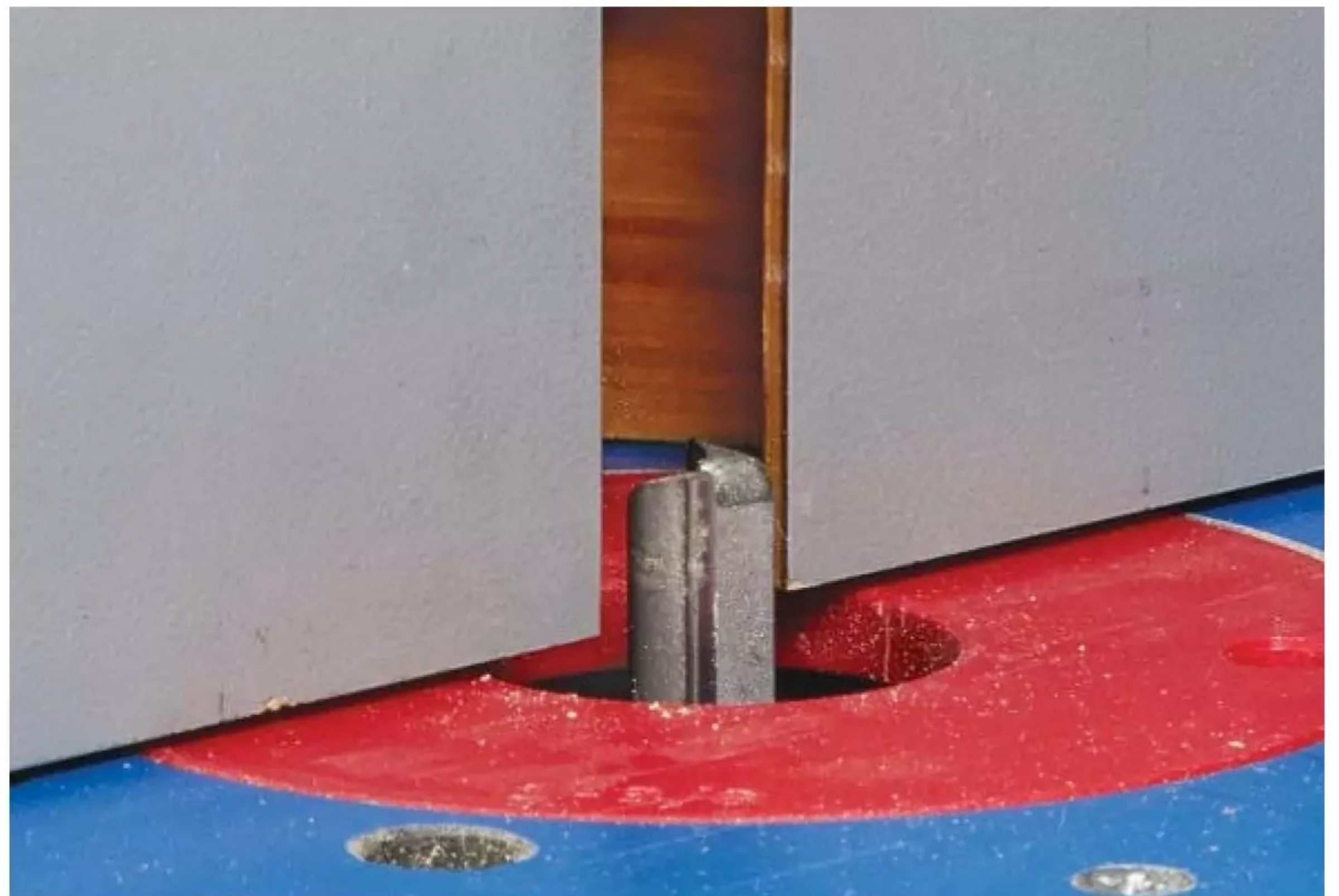
Adjustable Bit Opening. A fence with sliding faces allows you to adjust the size of the bit opening. It will be able to handle pretty much every bit and operation you can think of.
