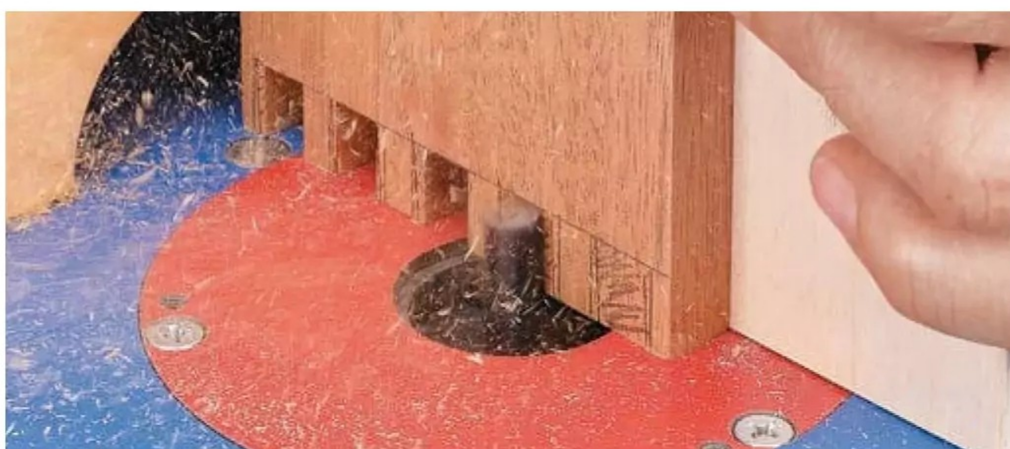
Remove the Waste. Install a straight bit sized to fit between the pins to remove the bulk of waste. Keep the wider side of the pins toward the bit to avoid accidentally cutting into them.
