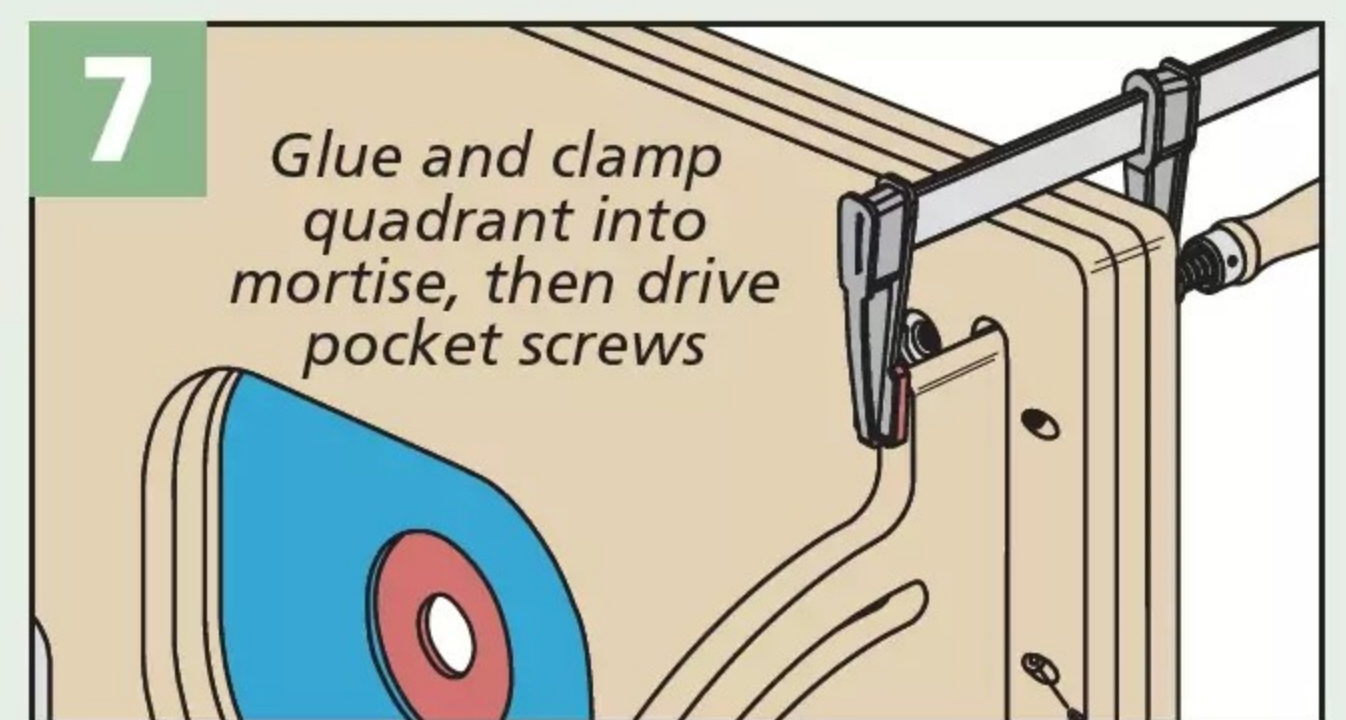
7 Reinforcements. Pocket screws augment the glue joint where the quadrant connects to the tabletop.
