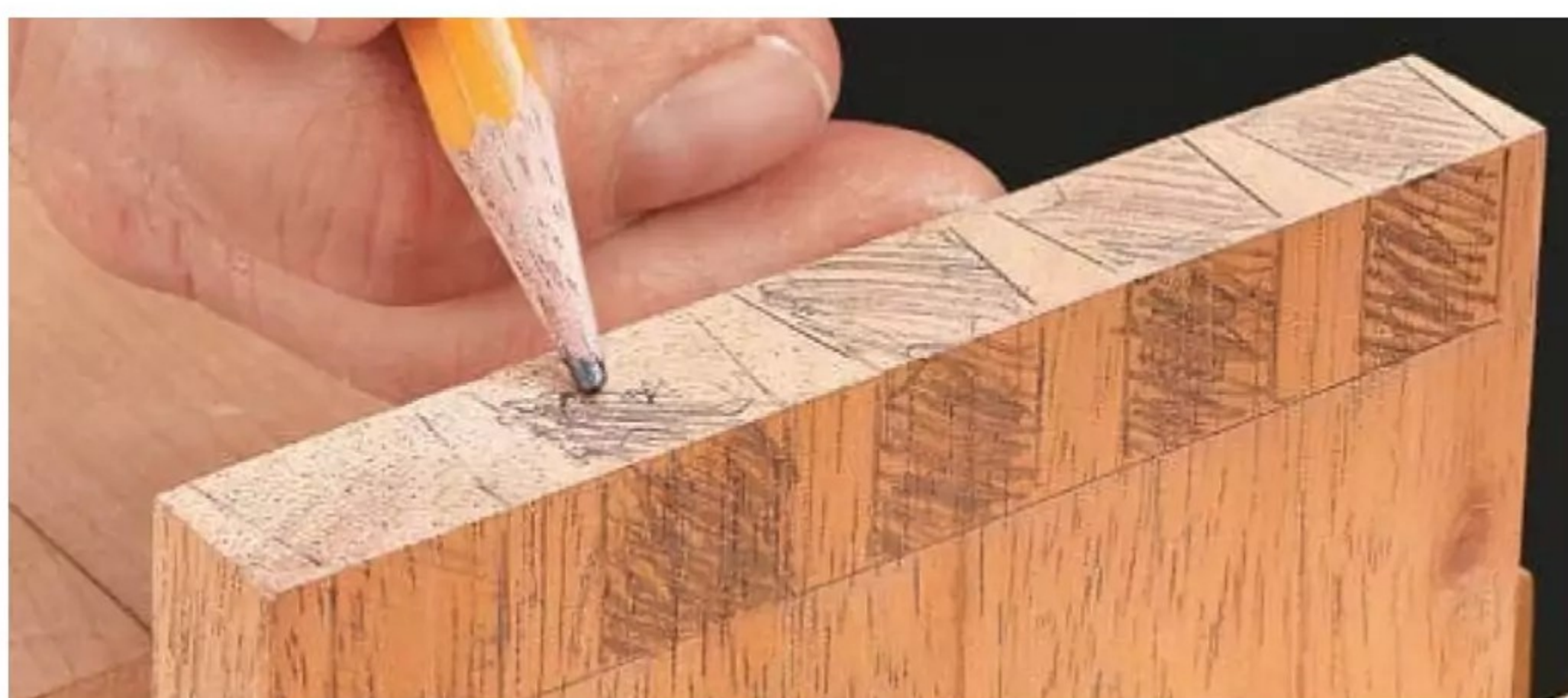
Color Prep-Work. By shading in the waste areas between the pins, you make it easier to line up the cuts with the straight router bit and reduce the chances for making a mistake.
