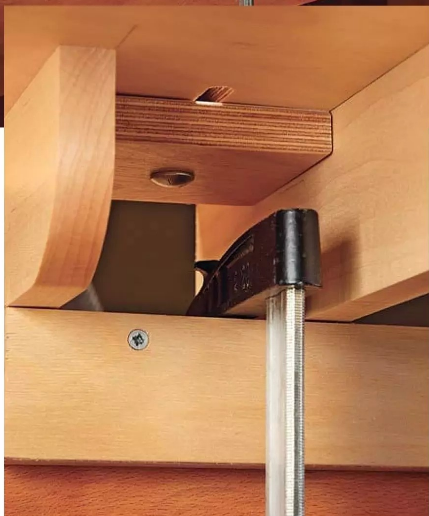
Clamp-on Table. A system of braces and cleats elevates the top and allows it to be secured with clamps.
