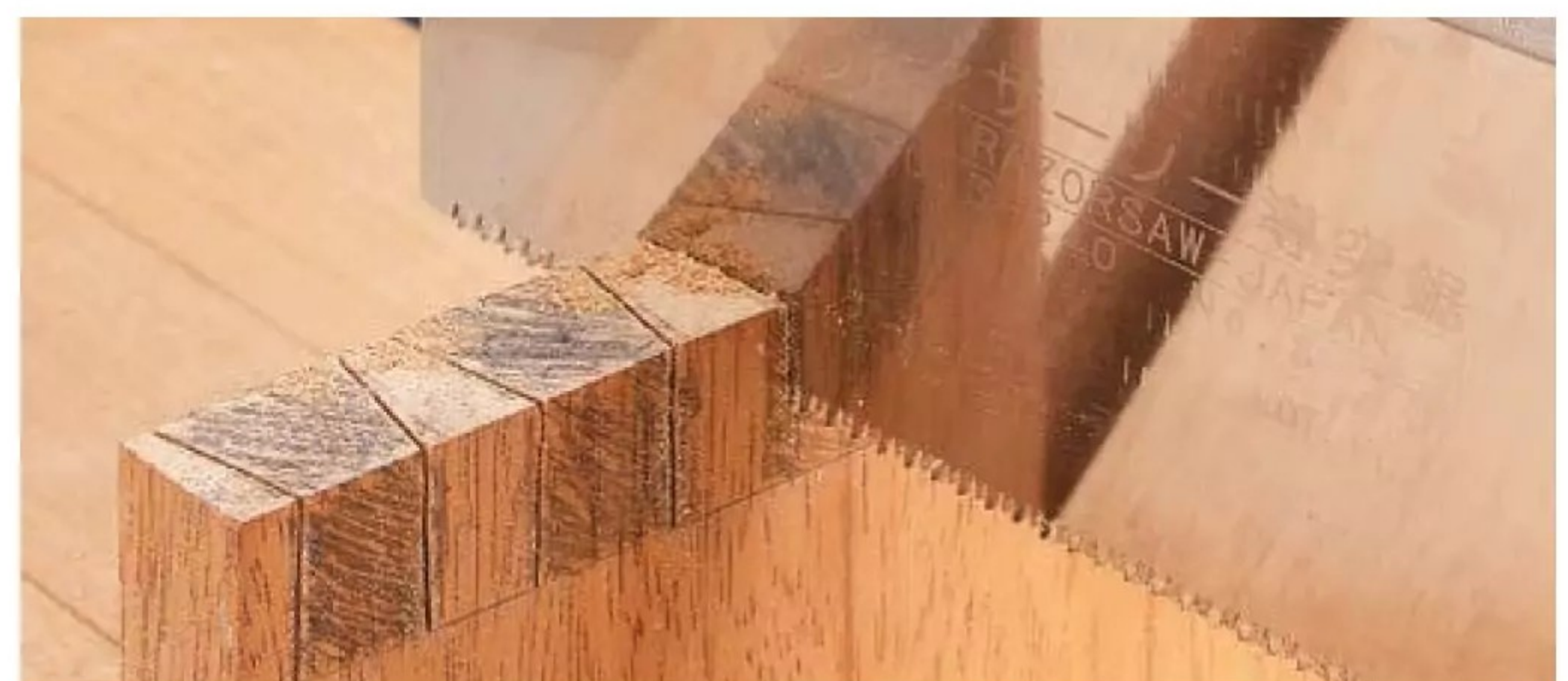
Begin Cutting. Use a hand saw to begin cutting the pins. The key is to leave the knife line intact on the pins for a good fit. You can clean up any excess during the final fitting.
