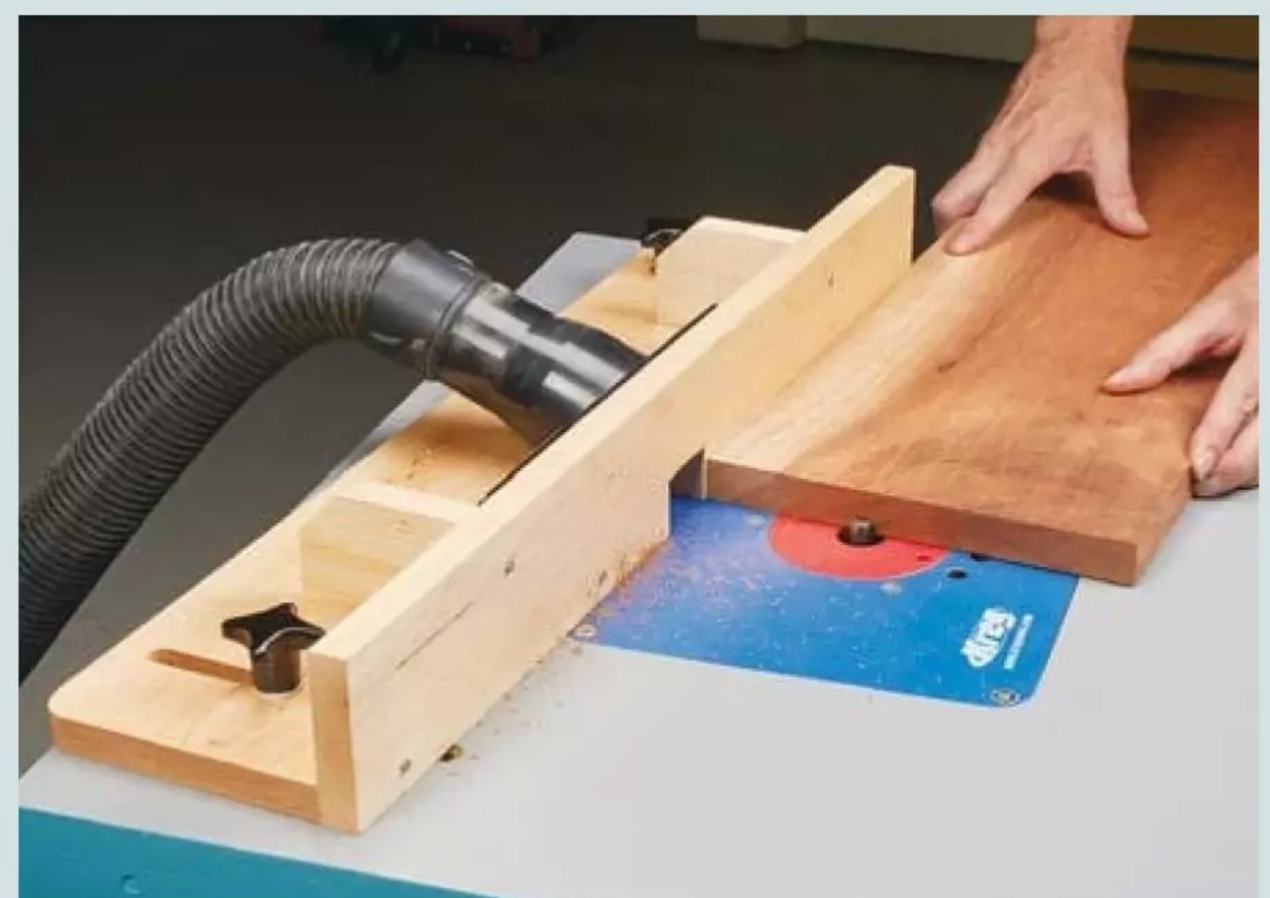
Router Fence Positioning. Unlike a table saw rip fence, the fence on a router table doesn't need to be parallel to the edge or miter gauge slot (if there is one).
