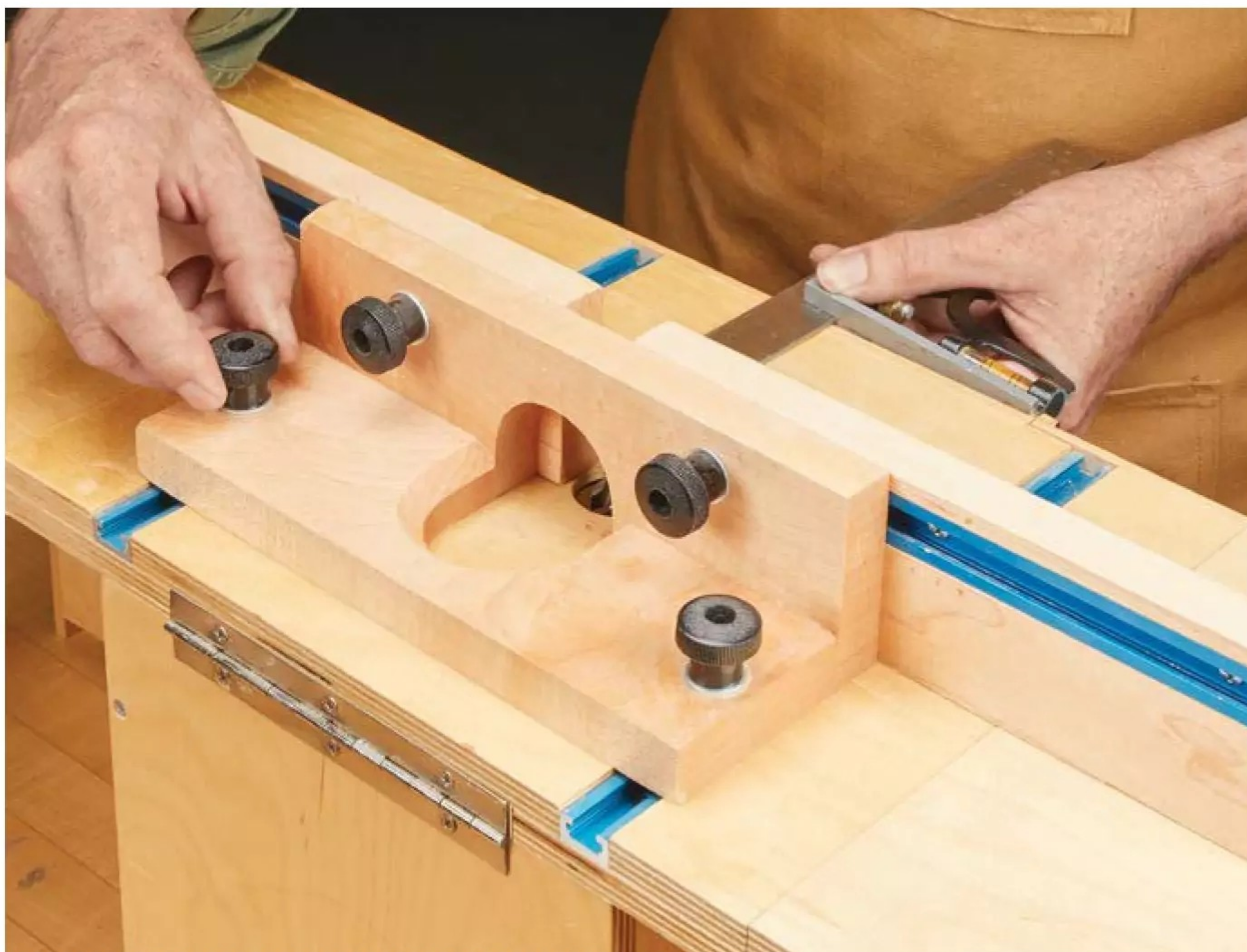
Adjustable Fence Setup. Flange bolts slide in a T-track and pass through holes in the fence base. Washers and knobs lock the fence in position (drawing at right). The fence slides back and forth smoothly when making large adjustments.
