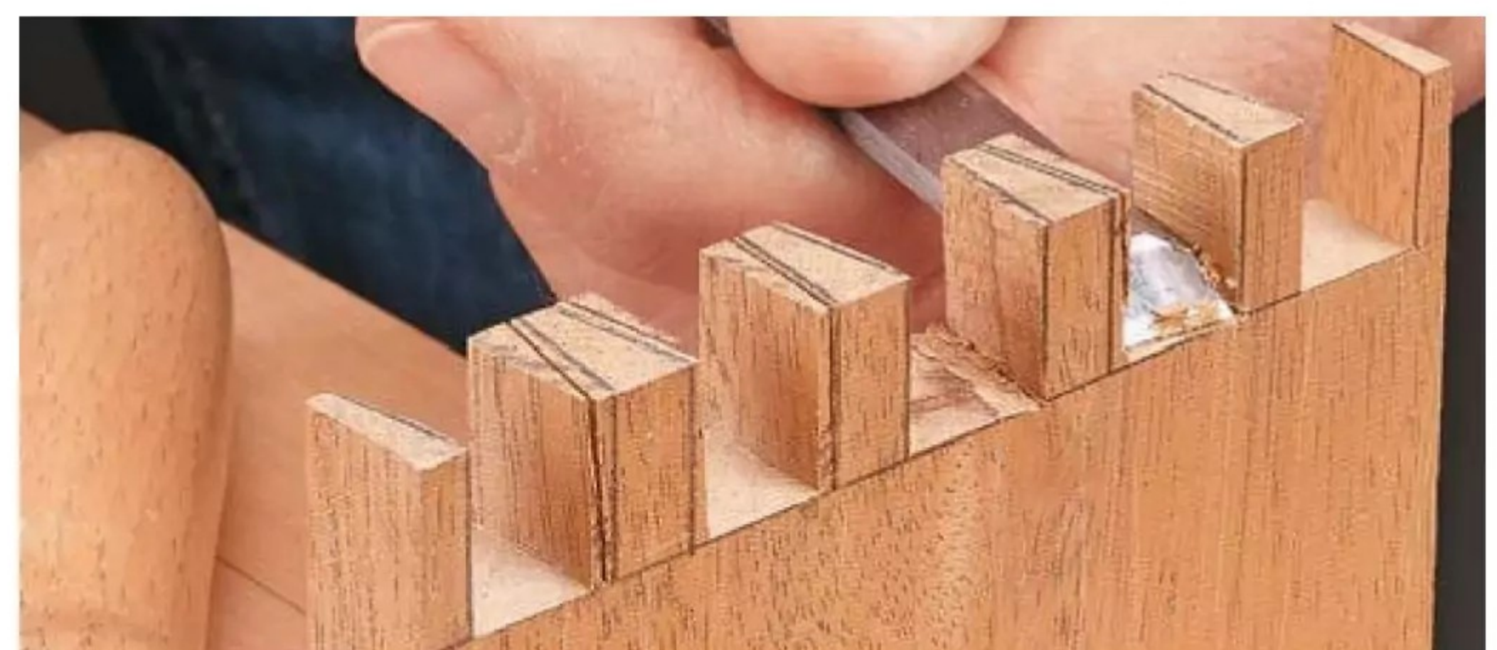
Tidy Up the Pins. The rest of the waste is easy to remove. I start with a coping saw to cut away the bulk of the material and then clean up and fine-tune the pins with a chisel.
