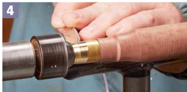
4 Brass Shaping. Start by turning away the brass ferrule, and getting that to shape. Leaving a large bulk of material in the handle will help reduce chatter from cutting the harder brass.
