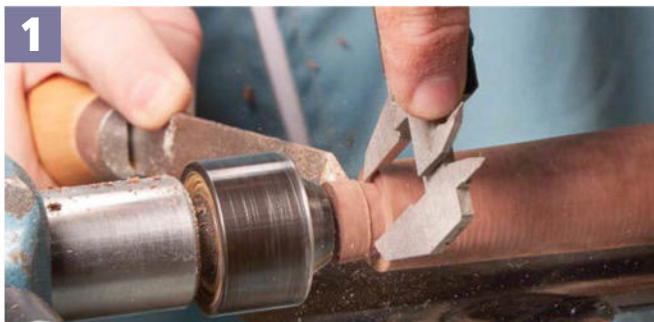
1 Ferrule Tenon. Turn a tenon on the tailstock end of the workpiece. Use a pair of calipers to measure the inside diameter of the brass tube, and transfer that to the blank.
