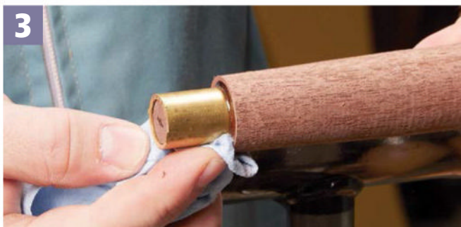
3 Glueup. Spread epoxy on the tenon and press the ferrule into place. Wipe away any squeezeout. Hydraulic pressure may push the ferrule off, so bring the tailstock up to "clamp" it in place.
