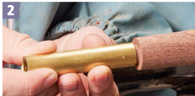
2 Test the Fit. Pull the tailstock away and test the fit of the tube. It should be snug the entire length of the tenon. Once you're happy with the fit, cut the tube to length.
