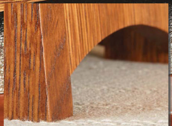
Fine Details. The sloped sides, tapered stiles, and a few curved details give this box strong Arts and Crafts appeal. Offset surfaces always add more visual interest.
