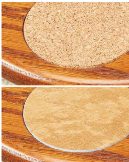
Coaster Material. Cork (top) or leather hide (bottom) are both suitable materials for the built-in coaster of the stand.
