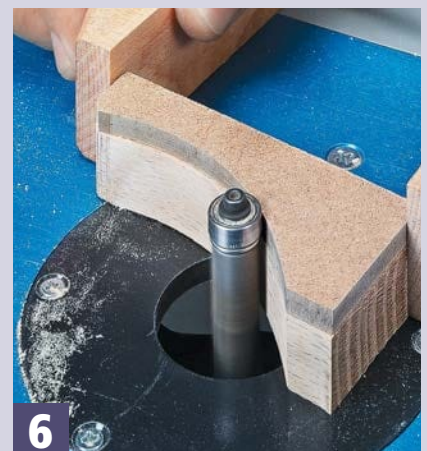
6 Final Trimming. With the template still attached, use a flush-trim bit to create a smooth, finished shape.
