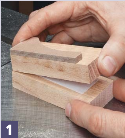
1 Stick & Stack. Use double-sided tape to stack the workpieces and fasten the template in place.
