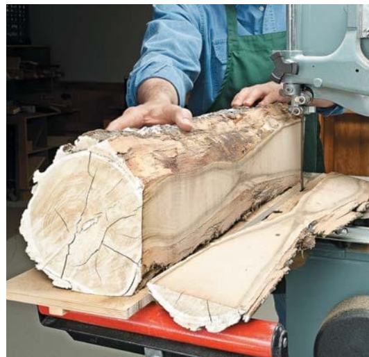
First Cut. Use a steady push to cut a wide, flat reference face on the log. An outfeed stand supports the sled.
