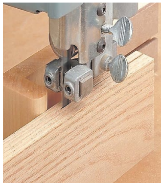
B. Stop/Pivot Block. An adjustable block does double duty as a stop (left) and a pivot block when resawing (right). Tightening a knob clamps the block on the fence.
