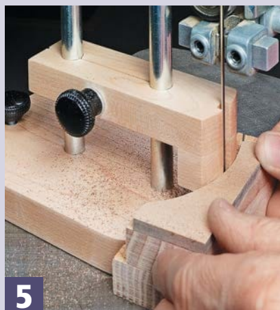
5 Cutting to Shape. Keep the template in contact with both points of the guide as you move through the cut.
