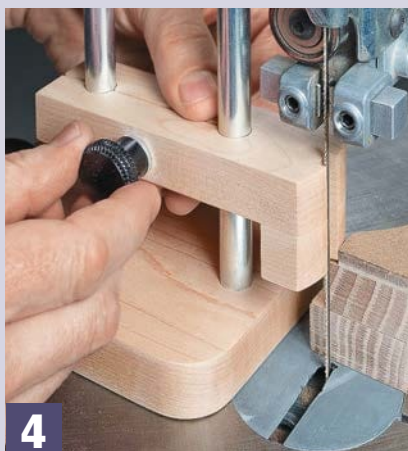
4 Guide Height. Adjust the guide so it contacts the template, making sure it doesn't contact the workpiece.
