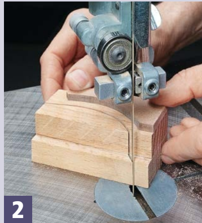
2 Roughing to Shape. To allow the workpiece to clear the base of the jig, you may have to remove some waste.
