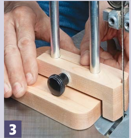
3 Jig Position. The blade fits in the notch on the guide. The points of the nose should extend \frac{1}{16} " beyond the blade.
