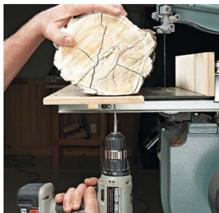
Overhang. Attach the log with screws so it overhangs the edge of the sled for the first cut.
