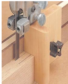
B. Stop/Pivot Block. An adjustable block does double duty as a stop (left) and a pivot block when resawing (right). Tightening a knob clamps the block on the fence.
