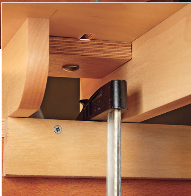
Raised Up & Locked Down. A system of braces and cleats elevates the top and allows it to be secured with clamps.
