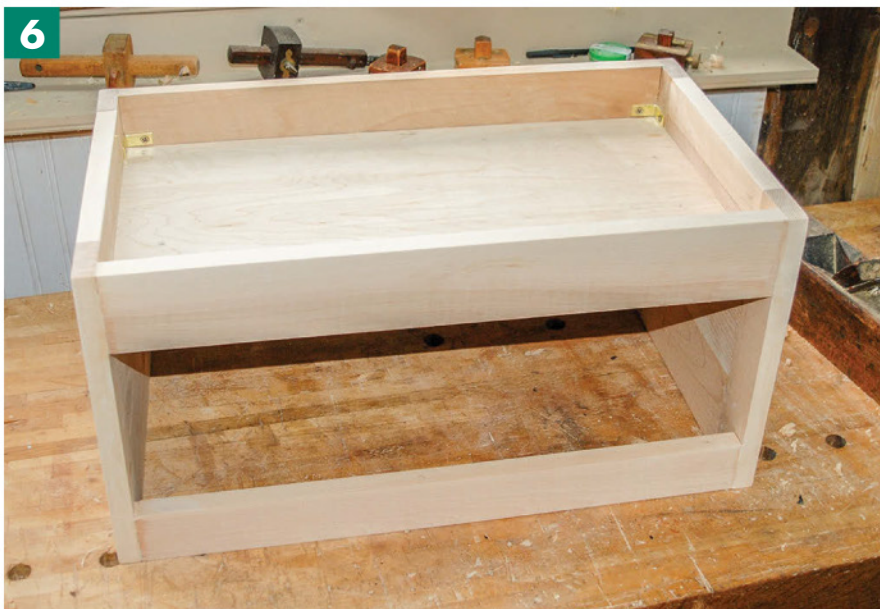
Pinned in Bottom. Size the bottom of the well to fit snugly in its opening. Once it's sized, attach the corner brackets to pin it in place on top of the ledger strips.
