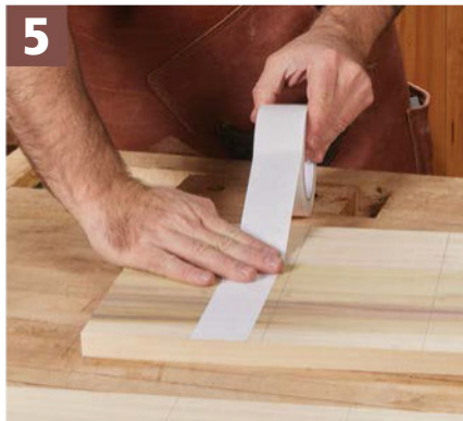
5 Stick Them Down. A pair of fences would guide the cuts on the dadoes, which I stuck down with double-sided tape.
