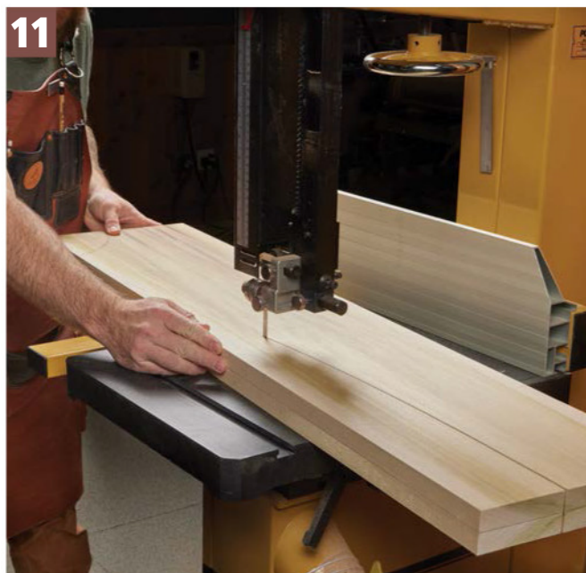
11 Rough Cut. Cut outside the layout lines at the band saw to remove most of the waste. This will save a good deal of time later on.
