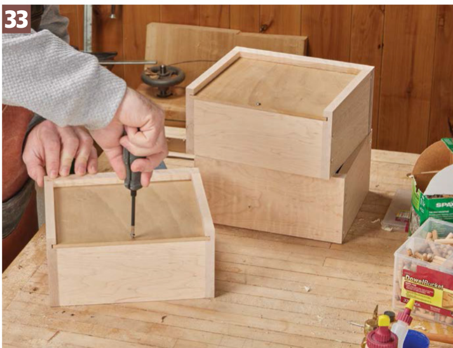
33 Drawer Bottoms. Slip in the bottom and drive in a screw to hold it. This makes the bottoms easy to replace should you need.
