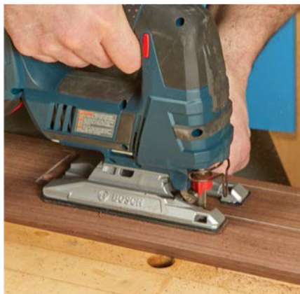
Drawer Opening. Drill out the corners, then use a jigsaw to rough out the opening for the drawer.
