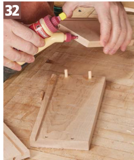
32 Dowel Glueup. To assemble the drawers, squeeze a bit of glue into the dowel holes, then fit the dowels in place.
