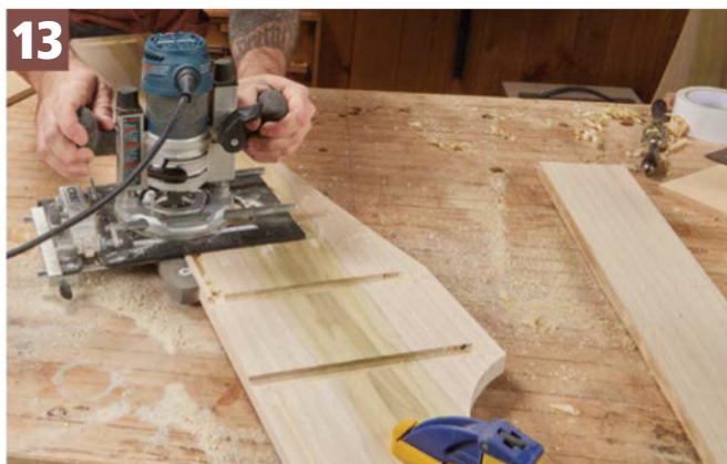
13 Back Rabbet. A rabbet along the back of each side will accept the back slats and the ledger board. Rout this using an edge guide.
