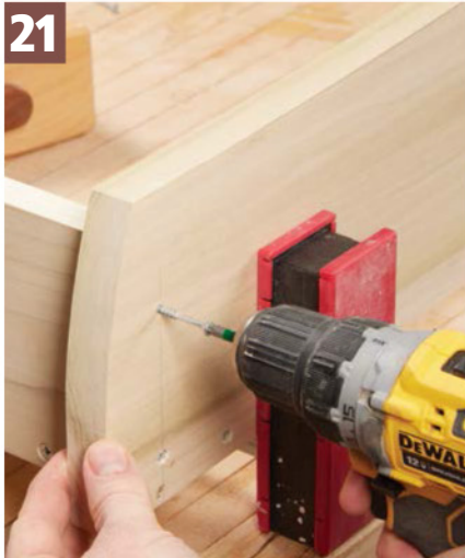
21 Secure with Screws. Drive a few screws in each joint. Spax screws don't require pilot holes, so you can drive them right in.
