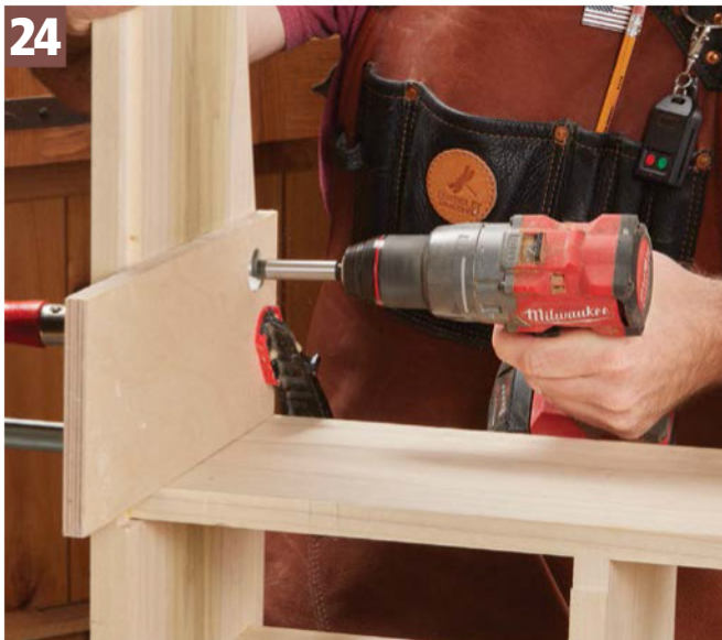
24 Drilling Template. A template helps position the Forstner bit to ensure the holes for the tool rest are aligned on either side.
