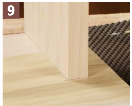
9 Check It Out. Fit the mating part into its respective dado to test the joint. Chisel away waste as needed for a good fit.
