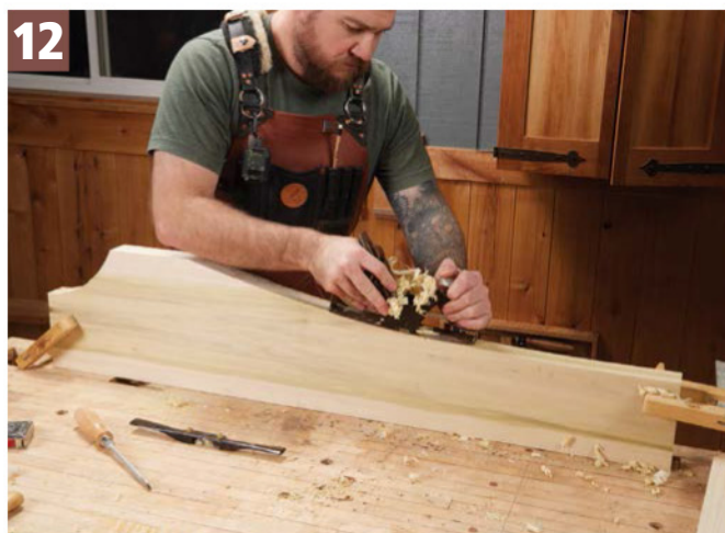
12 Work the Curve. Refine the shape of the curve. Rasps and sandpaper will suffice, but a compass plane is an ideal tool for this task.
