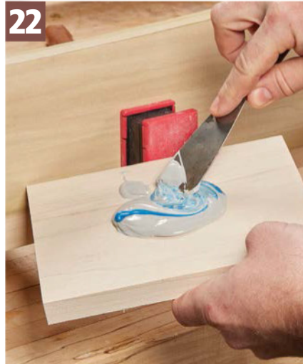
22 Wood Fill. Mix up Bondo , using a small amount at a time. Be sure the filler and hardener are thoroughly mixed.
