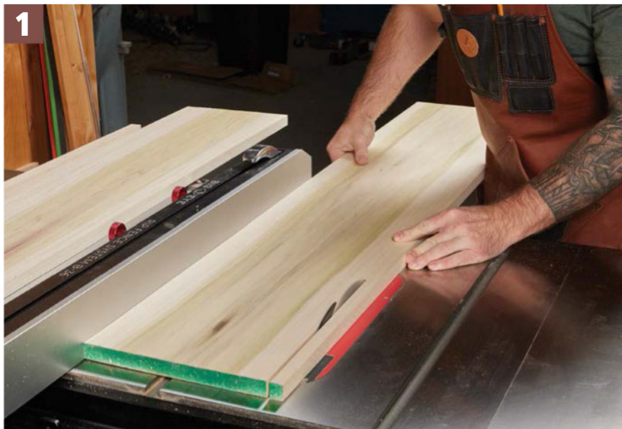
Rip to Width. Start this saw till off by milling down the stock for the sides, then cutting it to width. Poplar is available in wide boards, but you could glue up stock if you need to.
