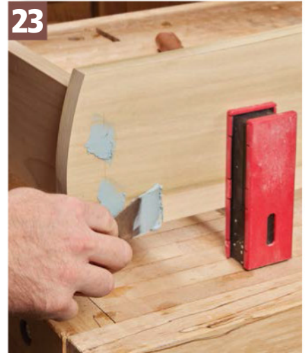
23 Cover the Holes. Cover the screw holes with the mixed Bondo . After 15-20 minutes, sand it flush with the surface.
