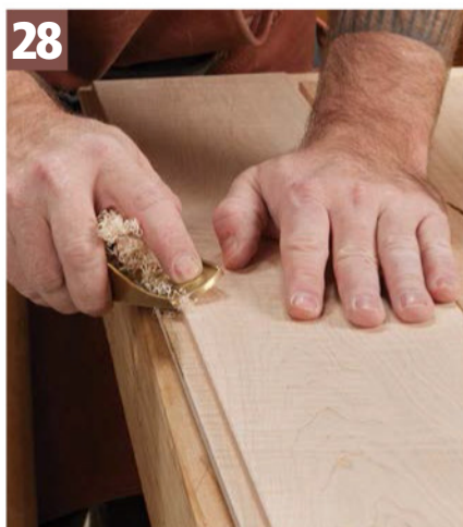
A Quick Chamfer. Use a block plane to chamfer the edges of the slats for a clean look and to help distinguish each one.
