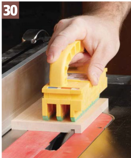
30 Bottom Panel Groove. A groove along the bottom edge of all the drawer parts will accept the bottom panels later on.
