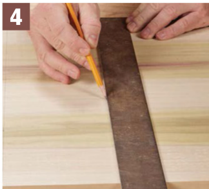
4 Side Dadoes. There are three dadoes in each side panel: one for the top, one for the bottom, and one for the divider.
