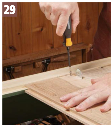
Screw 'Em Down. Screw the slats in place. A pair of screws on the same edge of each slat allows them to expand as needed.
