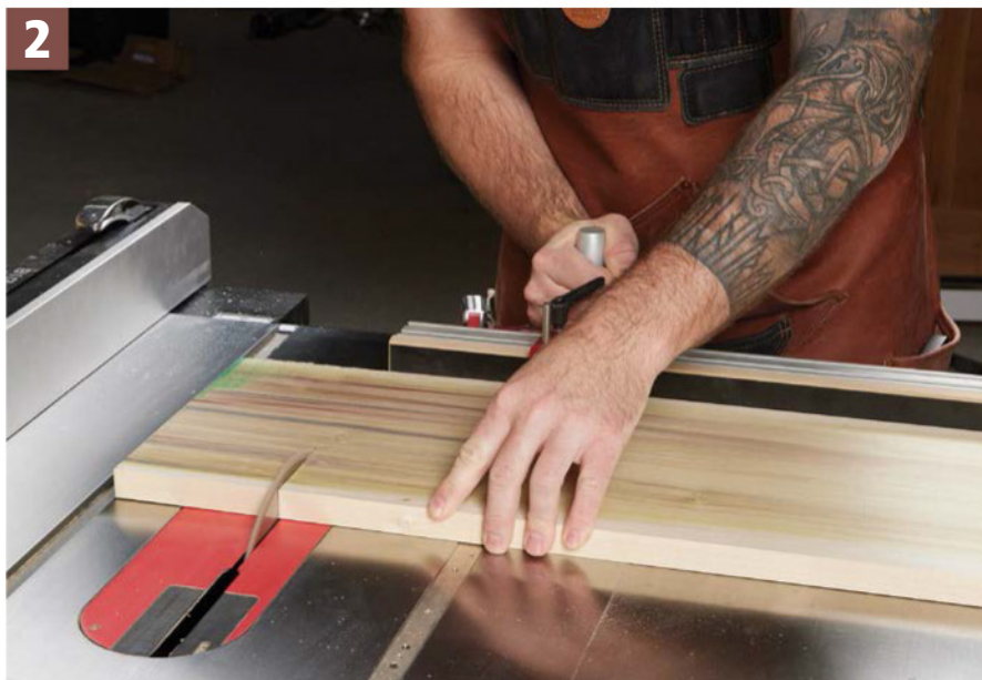
Crosscutting. I crosscut the side panels for the till at the table saw. I find my table saw and miter gauge to be far more consistently accurate than my miter saw.
