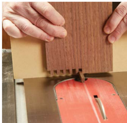
Finger Joint Jig. Building a simple jig with an auxiliary miter fence will ensure accurate box joints.
