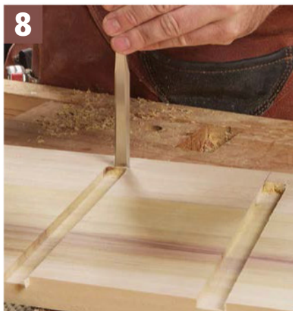
8 Square Up. Use a chisel to chop the ends of the dado square. Chop across the grain first to prevent splitting the joint.
