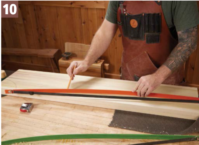
10 Arcing Layout. Lay out lines to shape the sides. A drawing bow, such as the one here, helps get smooth curves.
