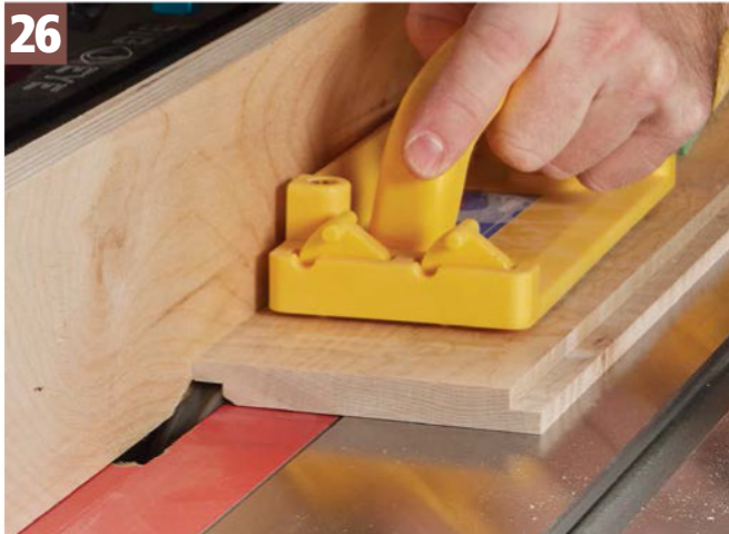
Shiplapped Back Slats. To create the back slats for this till, begin by rabbeting the edges of the back slats.
