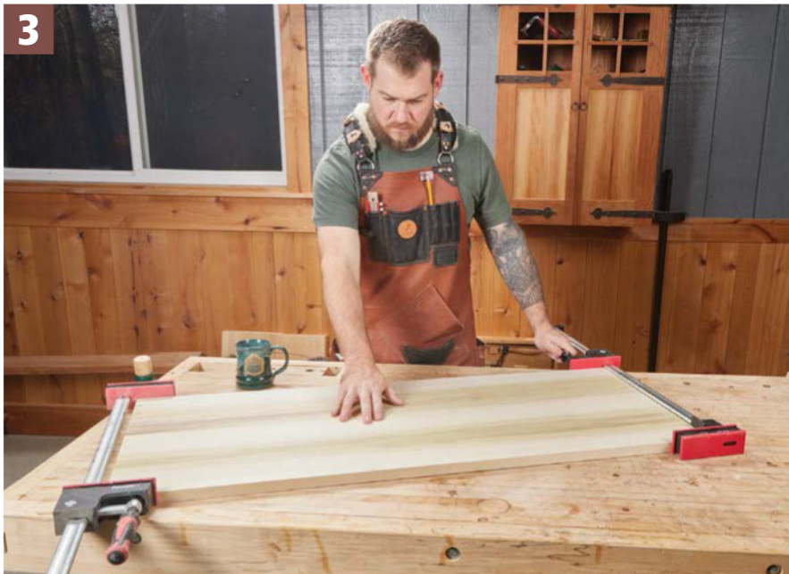
3 Joinery Layout. To ensure the joinery will line up from side-to-side, I clamp the parts together first before marking out the dado locations.
