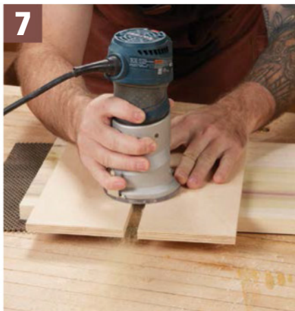
7 Routing Dadoes. A dado clean-out bit has a bearing to ride along the plywood fences while routing the stopped dadoes.
