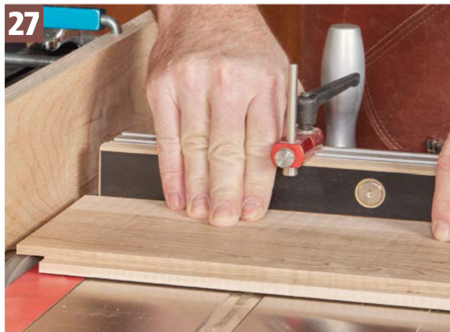
Room for the Cleat. To accommodate the top cleat that this till will attach to the wall with, rabbet the top, front face of each slat.
