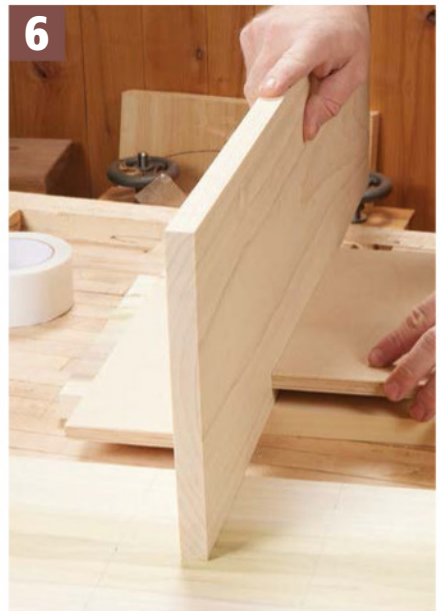
6 Dado Spacing. To ensure an exact fit in the dadoes, sandwich the mating part between two fences when setting up the dado cuts.
