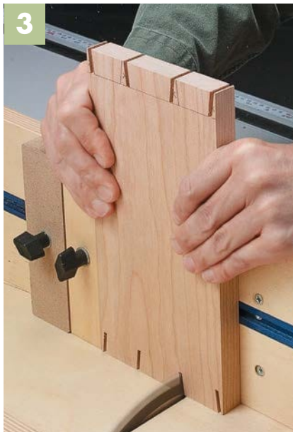
▲ Slip a spacer between the workpiece and the stop block to set up for the second set of cuts.
