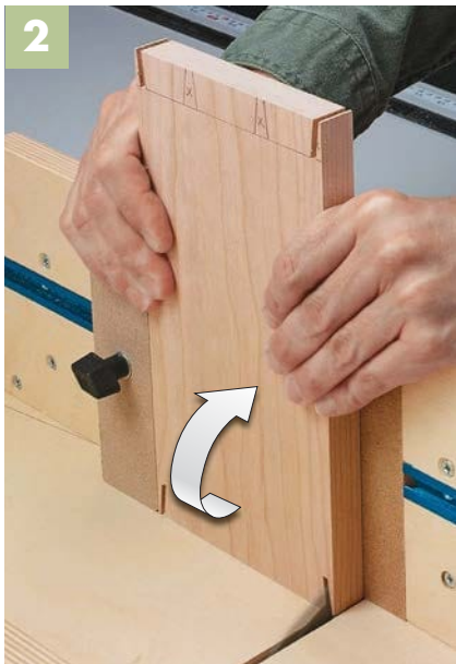
▲ A stop block registers your workpiece for the first cut. Be sure to rotate and flip the piece as needed.
