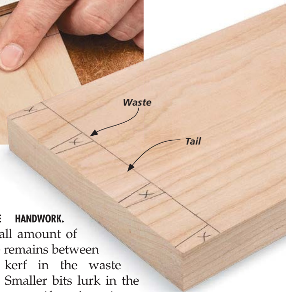
▲ Pencil lines are easy to see and all you need to set up the stops and spacers of the table saw jig. Scribe the baseline.
