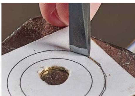
▲ Cutting thick metal with a cold chisel starts by cutting part way through on the vise anvil.
