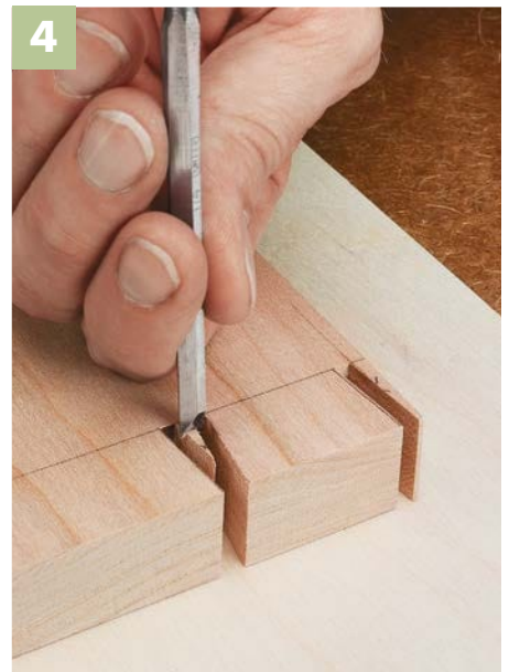
▲ The table saw cuts leave little waste to remove by hand. The saw kerfs and scribed line guide the way.
