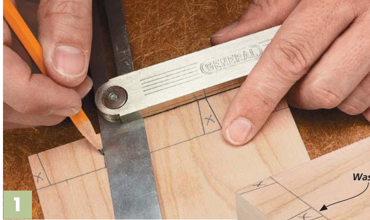
▲ Pencil lines are easy to see and all you need to set up the stops and spacers of the table saw jig. Scribe the baseline.
