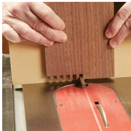
▲ Finger Joint Jig. Building a simple jig with an auxiliary miter fence will ensure accurate box joints.
