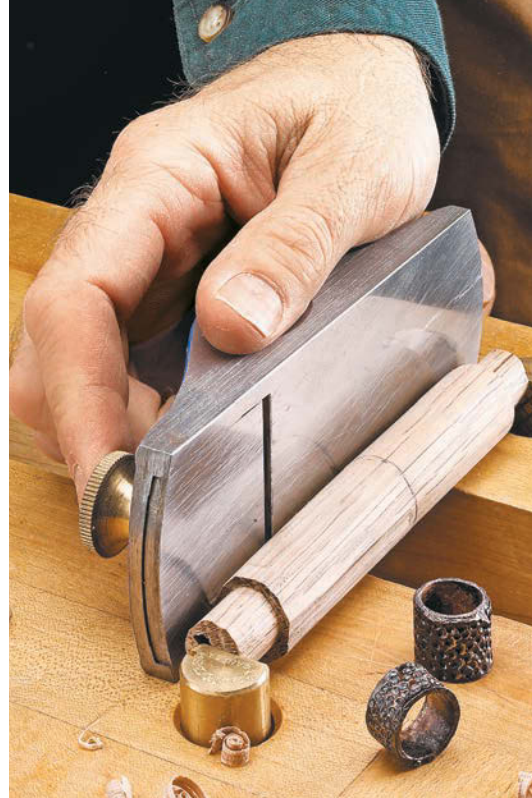
The Final Touch. Starting from the center, taper the handle toward both ends using a block plane to create a faceted, barrel shape.
