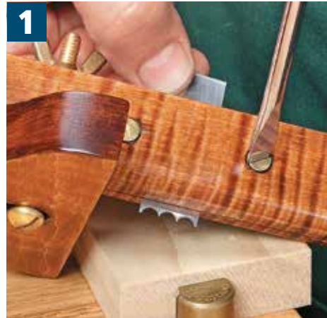
Cutter. Position the cutter in the beam to the desired depth and lock it securely by tightening the screws.
