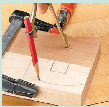
Drawing Arc. A block supports the tip of the compass when drawing the large arc on the upper fence piece.
