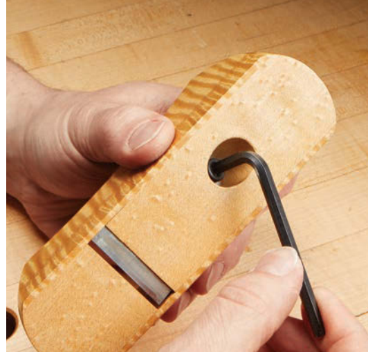
Securing the Blade. The blade is held in place by tightening the socket head cap screw with an Allen wrench.
