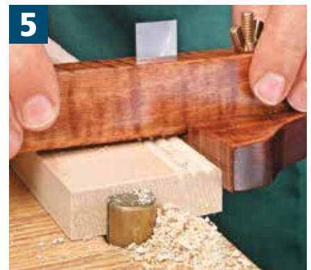
Cleanup. Use a light touch on the final pass to clean up the profile and remove waste from the creases.
