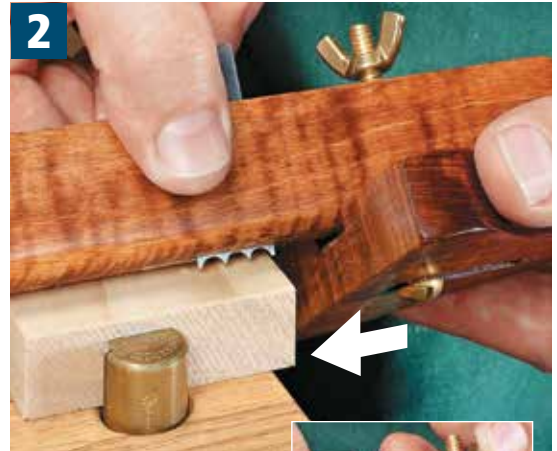
Fence. Set the fence to locate the profile. Then tighten the wing nut.
