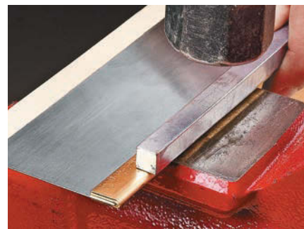
Crimp the Back. Finally, use the hammer and bar to crimp the brass back around the blade for a snug fit.
