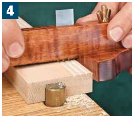
Multiple Passes. Tilt the scratch stock as you draw it across the workpiece with each pass to form the profile.
