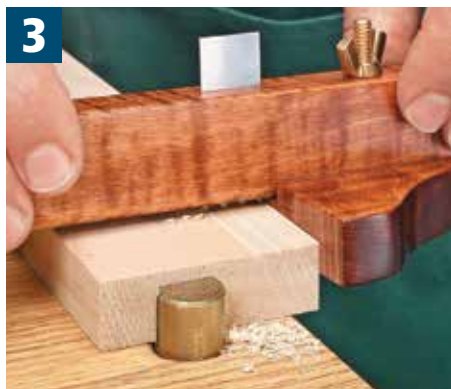
First Pass. On the first pass, lightly score the workpiece. Concentrate on keeping the fence against the edge.
