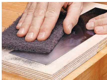
Clean Up. After filing away the rough edges, sand the bluing from the entire blade using a sanding pad.
