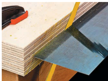
Use a Hacksaw. Clamping the blank between two pieces of plywood makes it easy to cut the blade to size.
