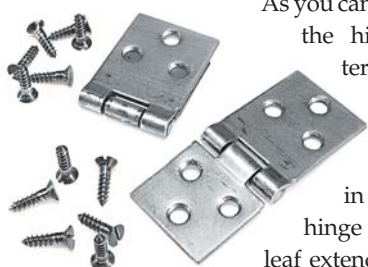
Hinges. The hinges used on a rule joint have a short leaf and a long leaf. This allows the hinge to bridge the joint.
