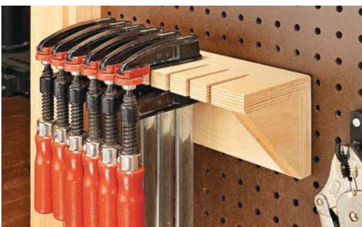
Racks. You can make plywood shelves and racks to store all kinds of tools on the pegboard racks.
