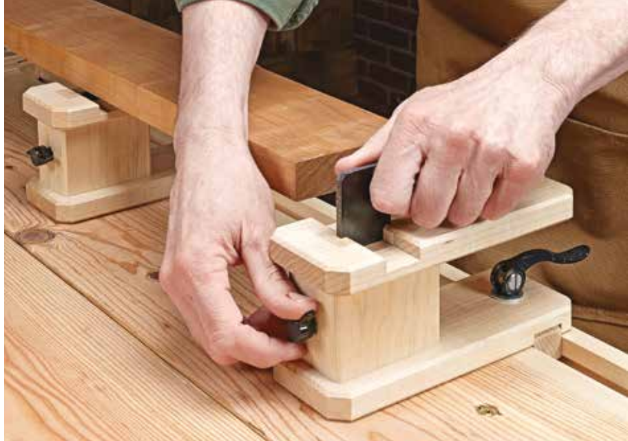
Support for Long Stock. A pair of supports slide along the bench rails and lock in place with cam clamps. An integrated, phenolic stop allows you to make accurate, repetitive cuts.
