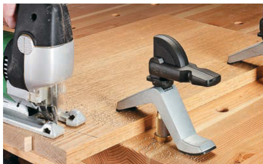
Hold-Downs. These cam-activated hold-downs secure a workpiece and allow you to reposition it quickly.
