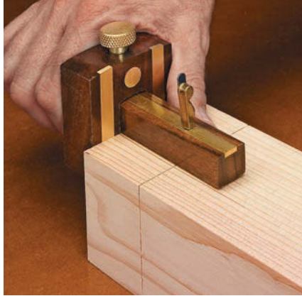
Shoulders. With a cutting gauge, score the shoulders to establish the tenon length.
