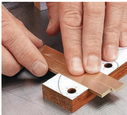
Shallow Dadoes. The gauge bars should project slightly above the dado and slide smoothly back and forth within it.
