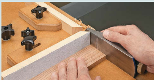
Square an End. With the fence set perpendicular to the edge of the shooting board, you can shave a hair off the end of a workpiece at a perfect 90° angle.
