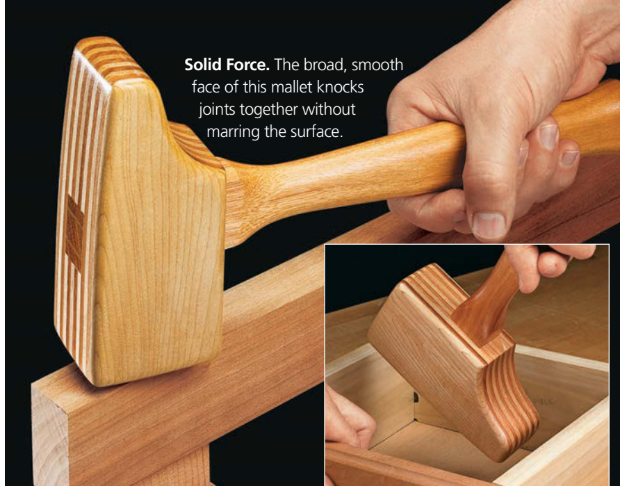
Gentle Taps. The small end reaches into tight areas to provide a little bit of "gentle persuasion" when joining parts.
