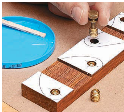
Install the Inserts. Use epoxy to secure the threaded inserts into the stopped holes drilled in the gauge body.
