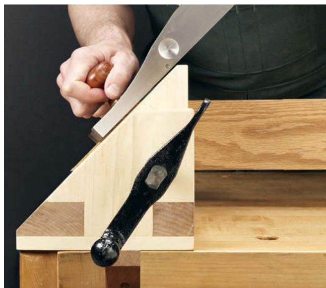
Position the Workpiece. When you clamp the workpiece in the miter jack, leave it slightly proud for trimming.
