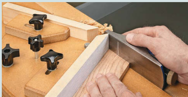
Other Angles. By disengaging the locking pin, you can adjust the fence for any angle. Simply lock it in place at the desired angle, adjust the fence, and you're ready to plane.
