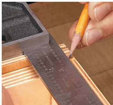
Lay Out Corner. Use a pencil and a combination square to mark the layout lines to guide the chisel.
