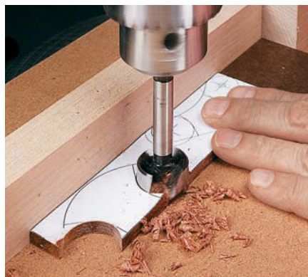
Shape the Cap. Form the inside radius of the cap first, then trim the remaining waste away at the band saw.
