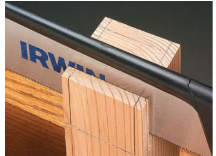
Cheek Cuts. Level the saw to complete the cheek cut. Take it slow to avoid overcutting.
