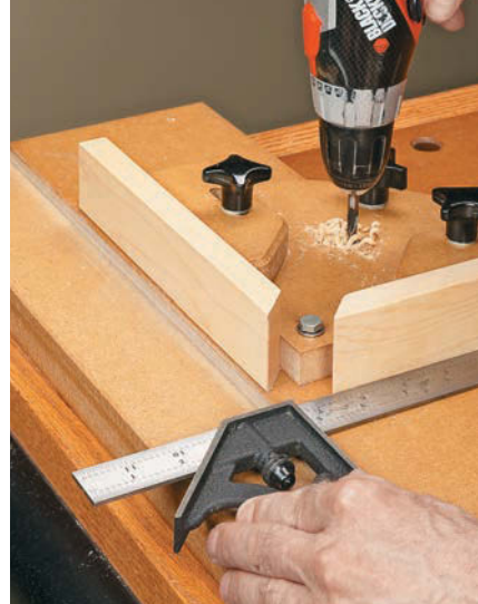
Square It Up. Repeat the process in order to drill the two holes in the fence base for the pair of 90° settings.
