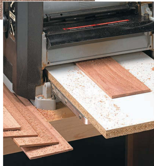
Planing Sled. Each strip is fastened to a sled with double-sided tape for planing.
