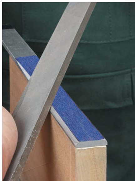
File the Edge Bevels. When shaping the bevels on the edges of the chisels, it's best to take long, even strokes for consistency.
