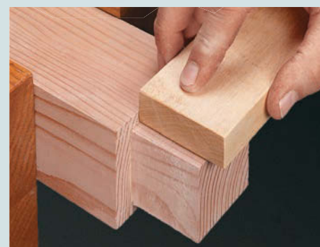
Sanding Block. A hardwood block with sandpaper on one face makes quick work of fine-tuning the fit of the tenon to the mortise.
