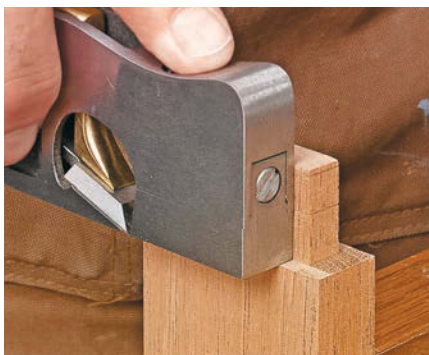
Plane It Smooth. A shoulder plane makes quick work of removing saw marks on cheeks and stepped shoulders.
