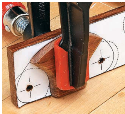
Attach the Cap. The removed pattern provides a reference for gluing and clamping the cap in the correct location.
