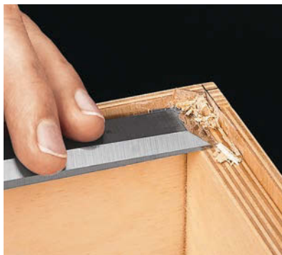
Remove Waste. After defining the corner with a vertical cut, clean out the waste with a paring cut.
