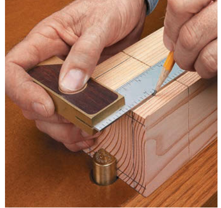
Cheeks. Transfer the marks on the end of the workpiece down each of the faces.
