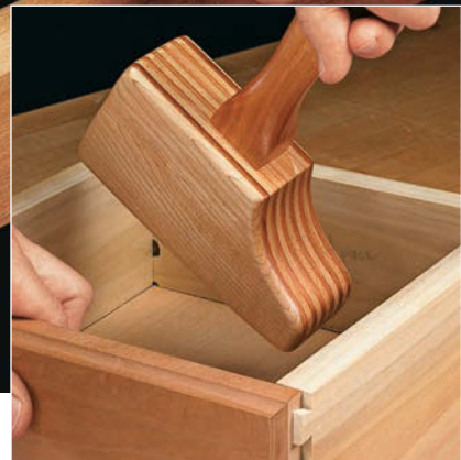
Gentle Taps. The small end reaches into tight areas to provide a little bit of "gentle persuasion" when joining parts.
