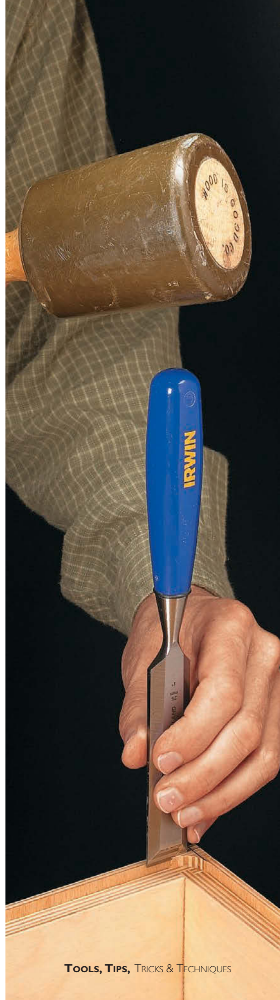
Remove Waste. After defining the corner with a vertical cut, clean out the waste with a paring cut.
