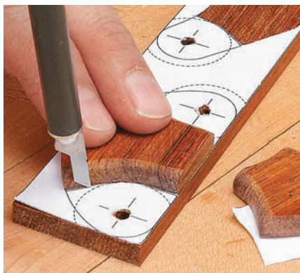
Locating the Cap. Use each cap as a guide to score the pattern, then remove those pattern pieces from the top.
