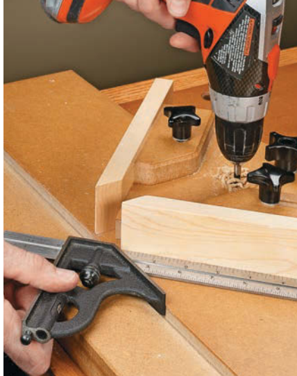
Setup for 45°. After positioning the fence, drill a hole in the base using the hole in the fence base as a guide.
