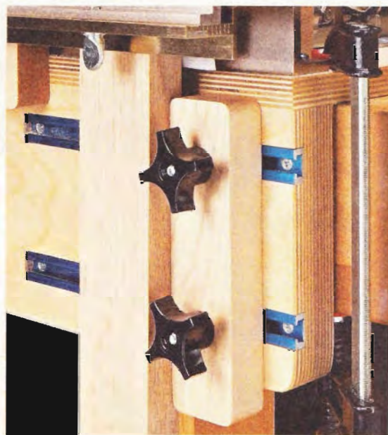
▲ The tenon stop provides a reference edge for positioning the tenon stock and making sure it's square to the jig and router.
