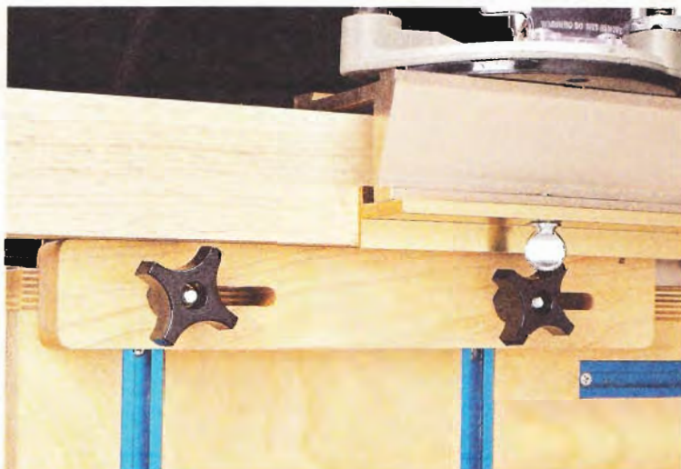
▲ In addition to holding the stock at the correct height, the mortise stop also allows you to move it right or left to perfectly position the workpiece by aligning your layout marks.
