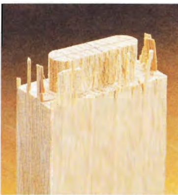
▲ The manual acknowledges that "flashing" can be a problem when cutting tenons.
