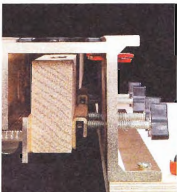
▲ The knobs are cumbersome and too slow when securing and removing a workpiece.
