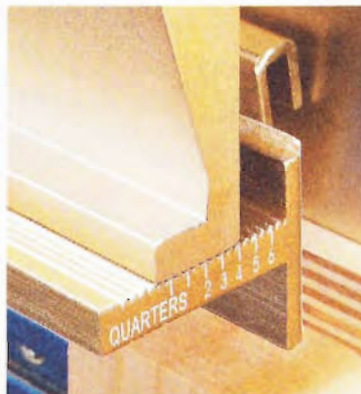
▲ Set the fence to match the thickness of the stock.
