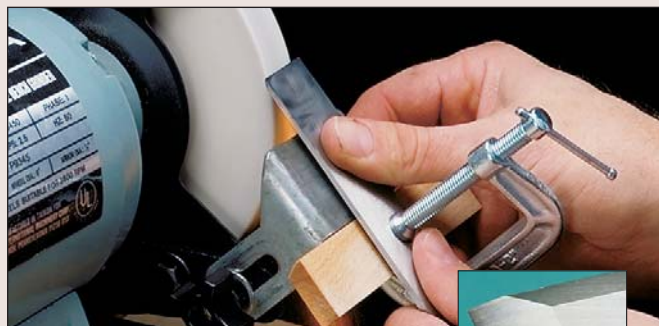
Grinding Wheel. A grinding wheel leaves a "hollow" bevel (see inset photo). A white, 60-grit aluminum oxide wheel leaves a smooth surface.
