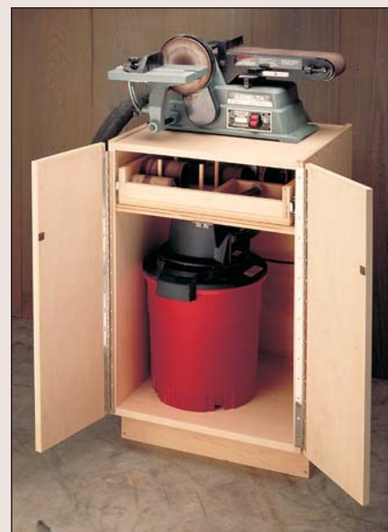
Shop Vacuum. Another solution is to dedicate an inexpensive shop vacuum to each sawdust-producing machine.
