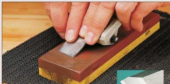
Waterstone. Next, the hollow-ground chisel is honed on a waterstone. This produces a small "flat" at each end of the bevel (see inset photo).
