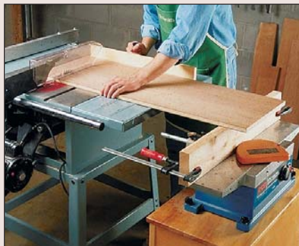
Support Work With Another Tool. A board clamped to the jointer fence supports workpieces on the table saw.
