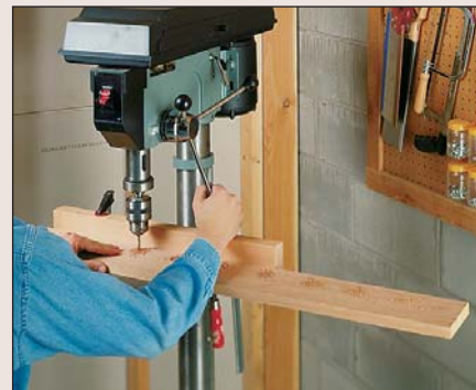
Use Corners. Even with this drill press tucked in a corner, you can still work with long workpieces.
