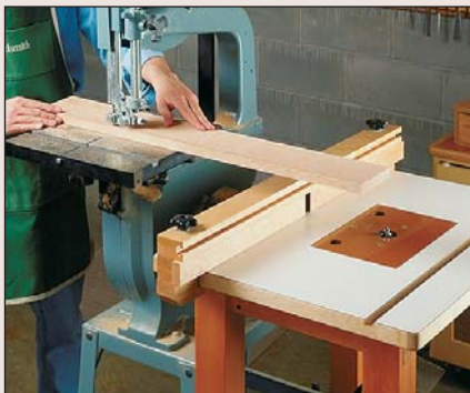
Overlap Tool Heights. Take advantage of different table heights by overlapping infeed/outfeed areas.
