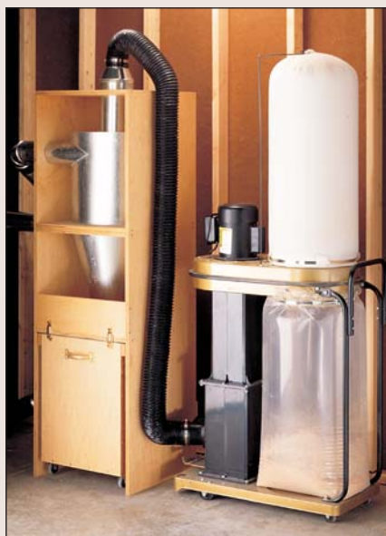
Dust Collector. If you have room, a dust collector is one of the most effective ways to contain dust in a small shop.
