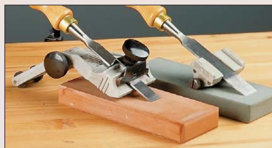
Honing Guides. A honing guide holds the chisel at the proper angle for sharpening. The guide will hold chisels of different widths and also plane irons.
