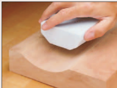
A piece of foam insulation board can be used to sand an irregular shape. First cut the block to rough shape.
