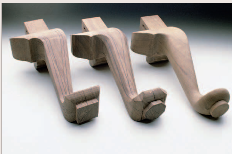
There are three basic stages in making a cabriole leg. In Stage 1, the blank is cut to basic shape on the band saw. In Stage 2, the corners are filed off. Finally, the corners are rounded over and the leg sanded smooth in Stage 3.
