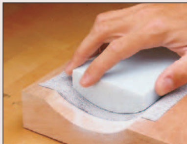
Smooth the shape of the block by rubbing it across a piece of sandpaper stuck to the workpiece.
