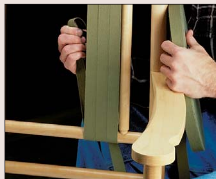
2 Now wrap the tape around the top and bottom rails, positioning the tape edge-to-edge. Make sure the tape in front is perfectly vertical.
