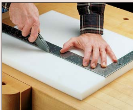
3 With half the tape wrapped, clamp it to a rail (refer to Step 4). Cut a foam pad to fit between the rails with a 1/2" gap around each edge.
