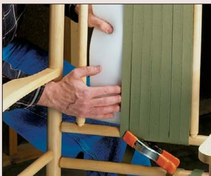
4 With the tape still clamped, feed the foam between the two layers of tape. Continue to wrap the warp until you reach the opposite side rail.
