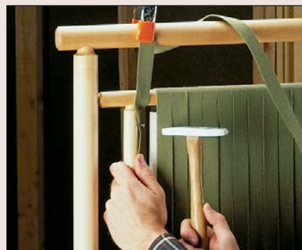
5 After the last row is completed in front, wrap the tape around to the back and up to the top of the side rail. Tack it in place and trim the excess.
