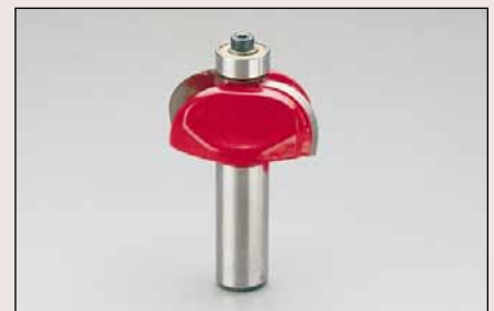
Anti-kickback Bits. A bit with less cutter surface exposed lessens the likelihood of kickback.
