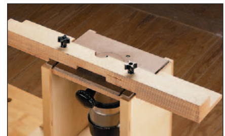
The router table fence slides forward and back. Plus it provides infeed and outfeed support for workpieces.
