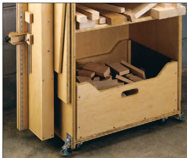
The removable scrap bin is big enough to hold lots of cut-offs. But the handles make it easy to lift out and empty.
