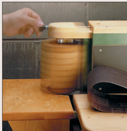
Changing Belts. Tightening a quick-release tension device makes it easy to install or change a sanding belt.
