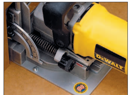
Pre-drilled holes in the base of some plate joiners can be used to screw it in place directly onto the table.
