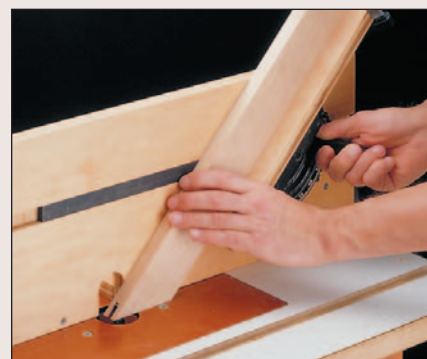
Angled Pieces. The miter gauge and an auxiliary fence are able to tilt forward or backward, which really helps when you're routing grooves for splined miters.
