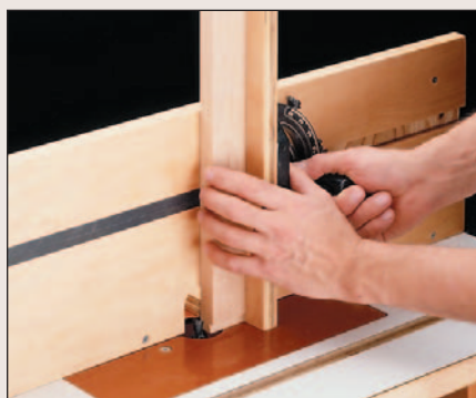
Long Pieces. Long narrow pieces need even more support than panels. Adding a miter gauge with an auxiliary fence keeps the piece from tipping forward or back.
