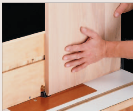
Large Panels. Routing a dovetail tongue on the ends of a panel can be difficult with a short fence. This tall fence keeps the panel exactly 90° to the router bit.
