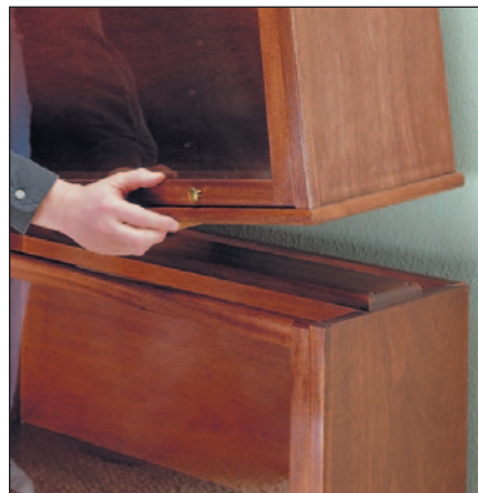
The cleat system is very sturdy. These interlocking cleats create a quick, secure connection so the sections can be assembled in a matter of seconds.
