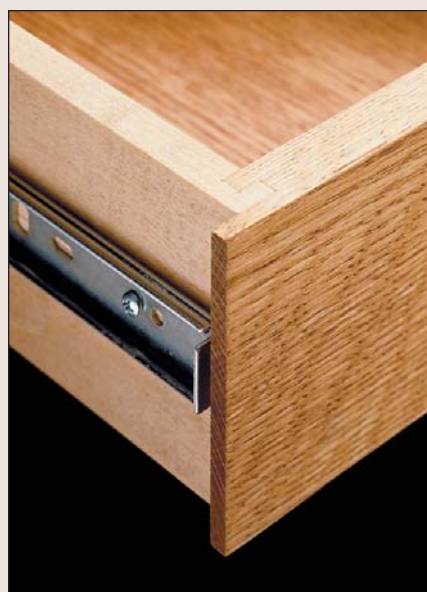
Lipped Joint. To hide the metal slide portion of the drawer slide, this locking rabbet has a lip on the drawer front that extends past the side.
