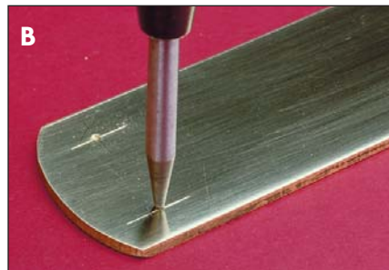
To keep the drill bit from "skating" across the plate, use a punch to make small dimples where the screw holes will be.
