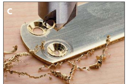
A regular countersink bit can be used to drill the countersinks in the brass plates. (Also refer to the Shop Tip on page 37.)
