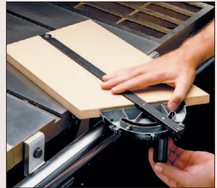
Second Angle Setting. Flipping the angle gauge over and repeating the process automatically sets the miter gauge to the exact opposite angle.
