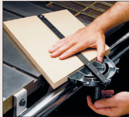
First Angle Setting. To set the first angle, hold the miter gauge upside down, pivot the head so it's tight against the end, and lock it in place.
