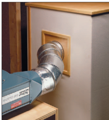
To avoid sharp turns, a pair of adjustable elbows connects the vacuum on the cyclone to the filter box.
