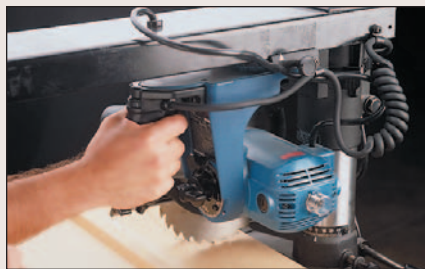
Universal Motor. Because it operates at high speed, a tool with a universal motor runs louder.
