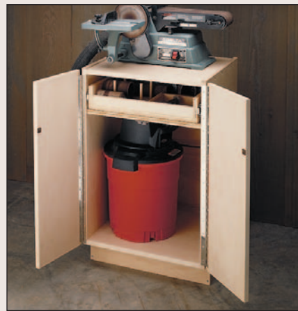
Shop Vacuum. Here, an enclosed cabinet is used to muffle the shrill pitch of a shop vacuum.
