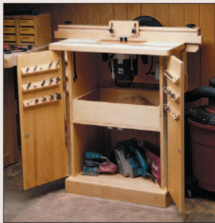
Router Cabinet. An enclosed cabinet decreases the noise level of this router from 100dB to 90 dB.
