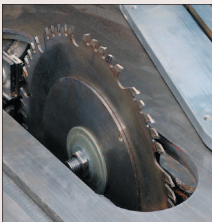
Stabilizer. By adding side support, a stabilizer damps noise produced by a wobbly blade.
