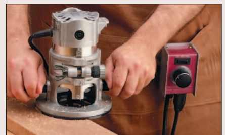
Speed Control. To reduce the RPM (and noise) of a fixed speed router, use a speed control unit.
