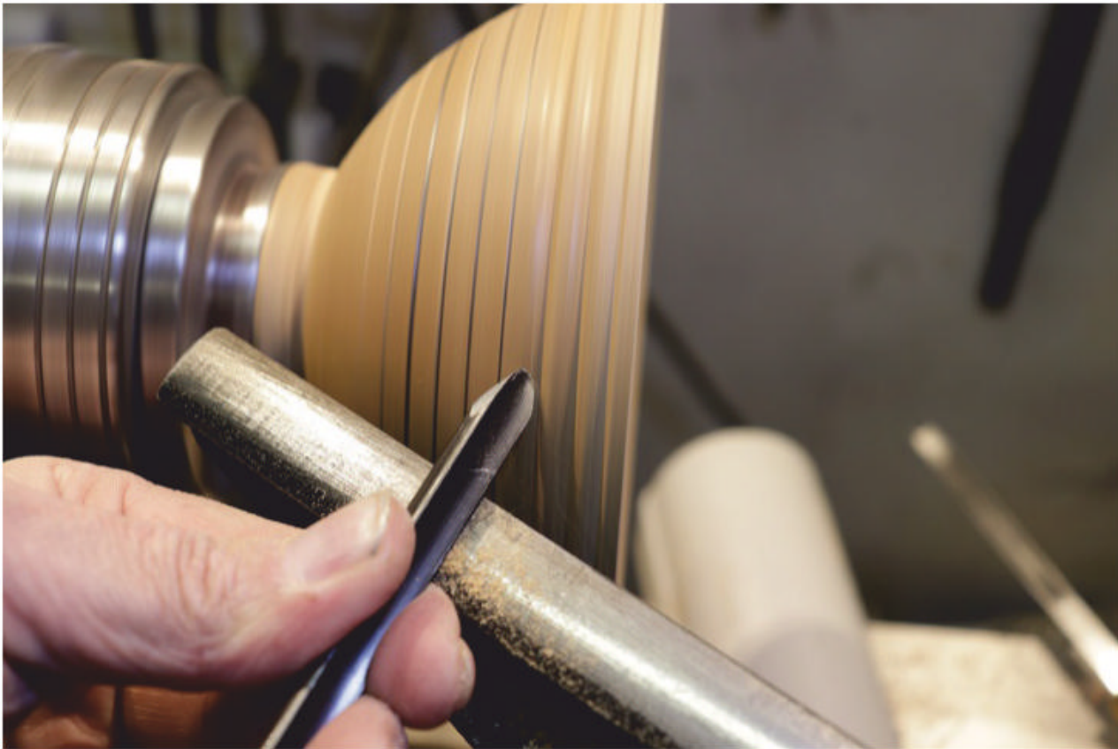
▲ Using a spindle gouge to cut the right-hand side of the bead.
