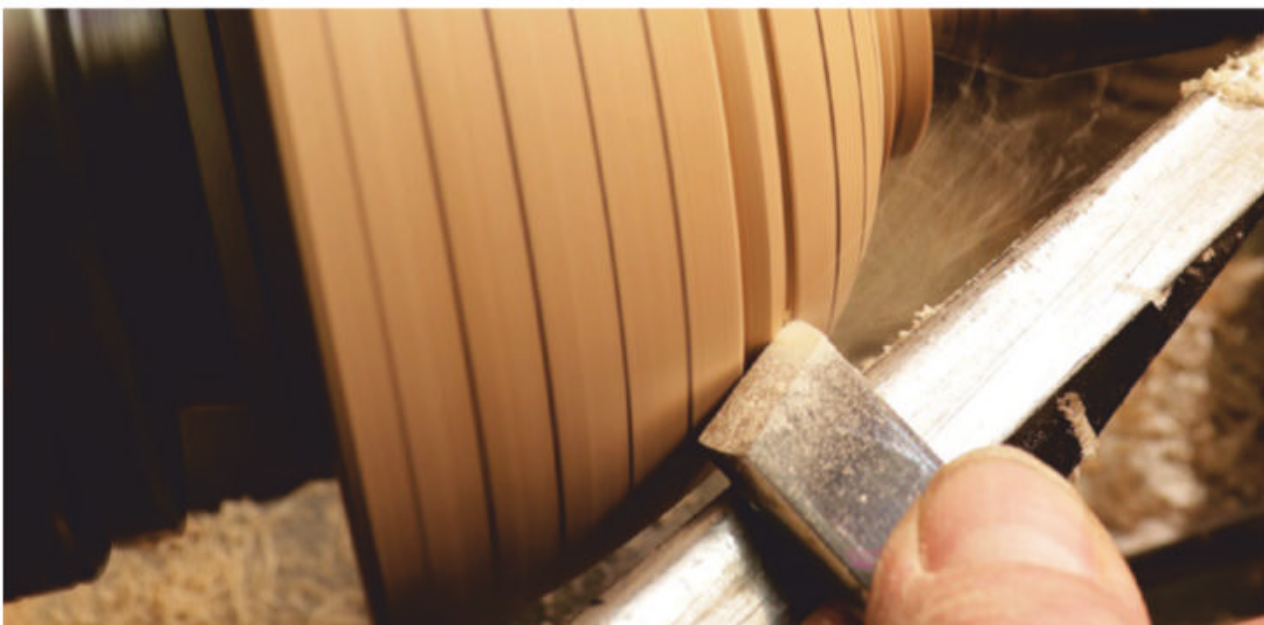
▲ Using the skew chisel to form a bead.
