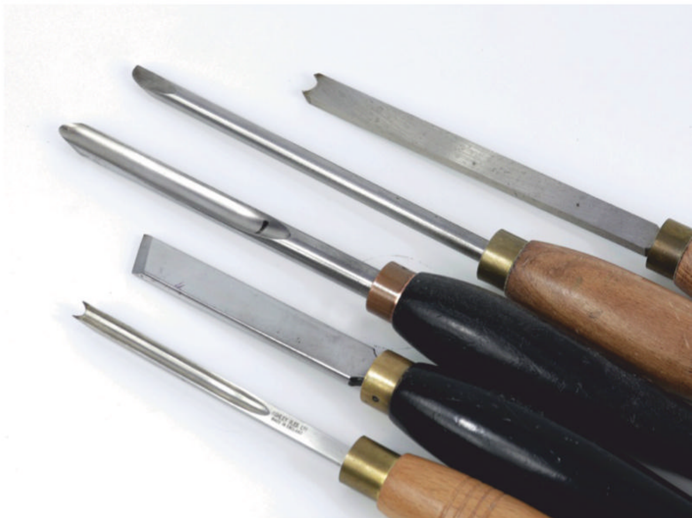
▲ Tools from the top: bead-forming tool, scraper, spindle gouge, skew chisel, bead-forming tool.
