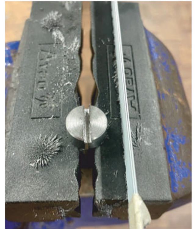
▲ The slot in the machine screw was cut with a hacksaw equipped with two blades.
