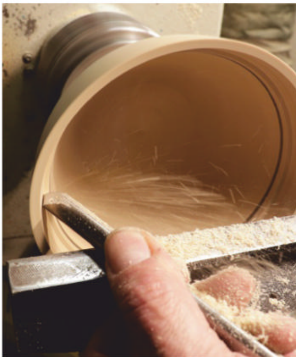
▲ Cutting down to the inner rim depth.
