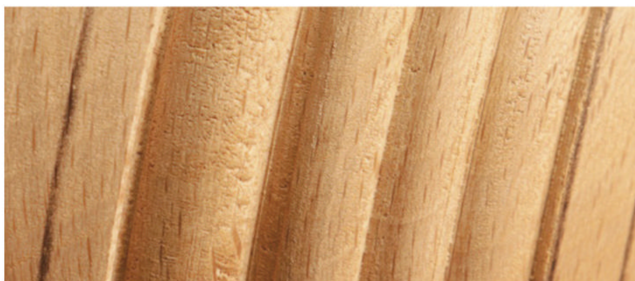
▲ Cut beads. One bead shows badly torn grain.
