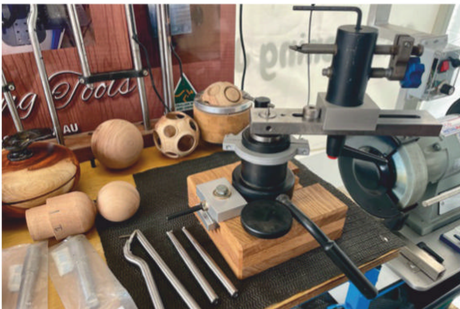
▲ Gerald Rensen from Jesse Engineering showcased his clever ball turning jig and the special tungsten carbide extension arms crafted specifically for Aussie timbers.
