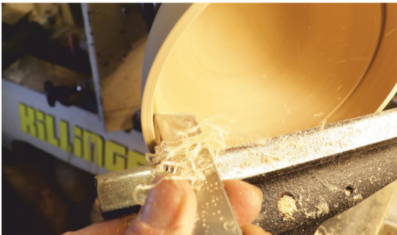
▲ A skew used in scraping mode to sharpen detail.
