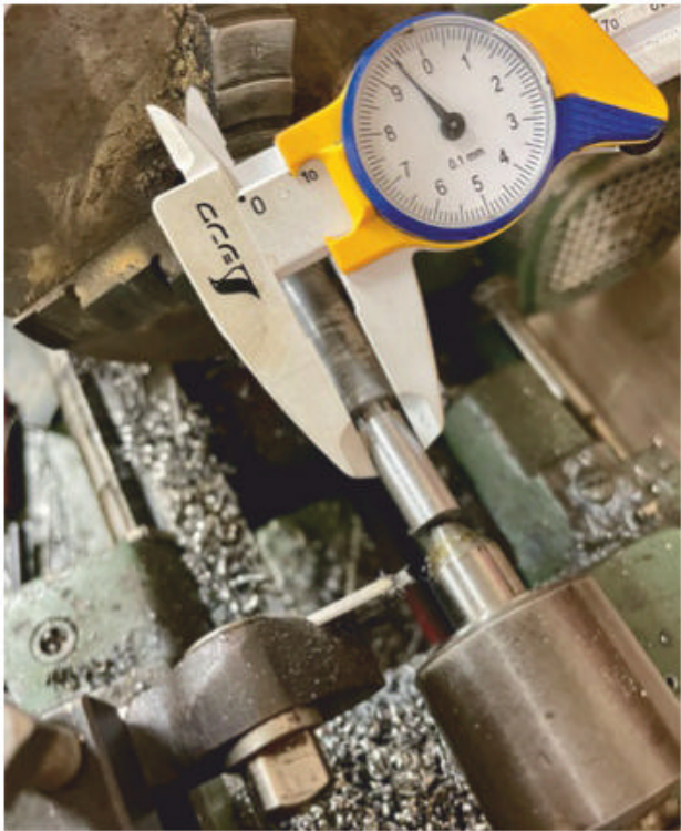
▲ The bolt stock necked and then turned down to 9.5mm diameter.
