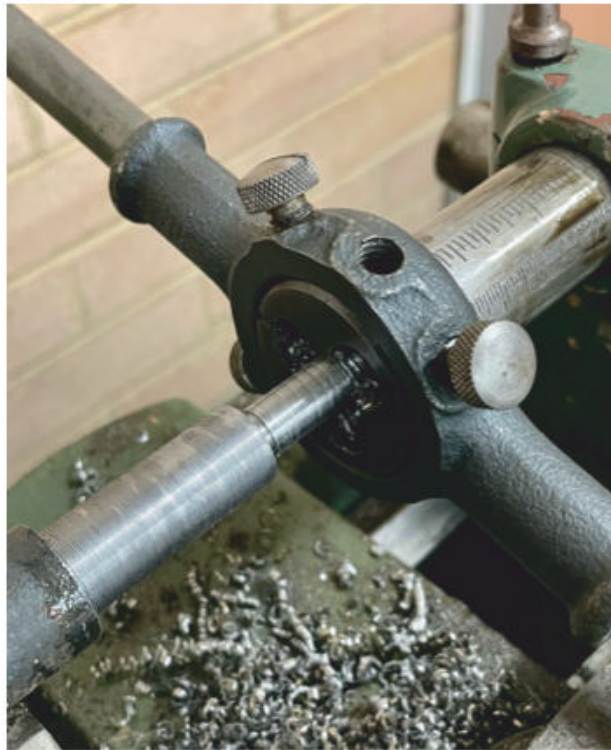
▲ Using the tailstock to support the 3/8" Whitworth die as it cuts the thread.
