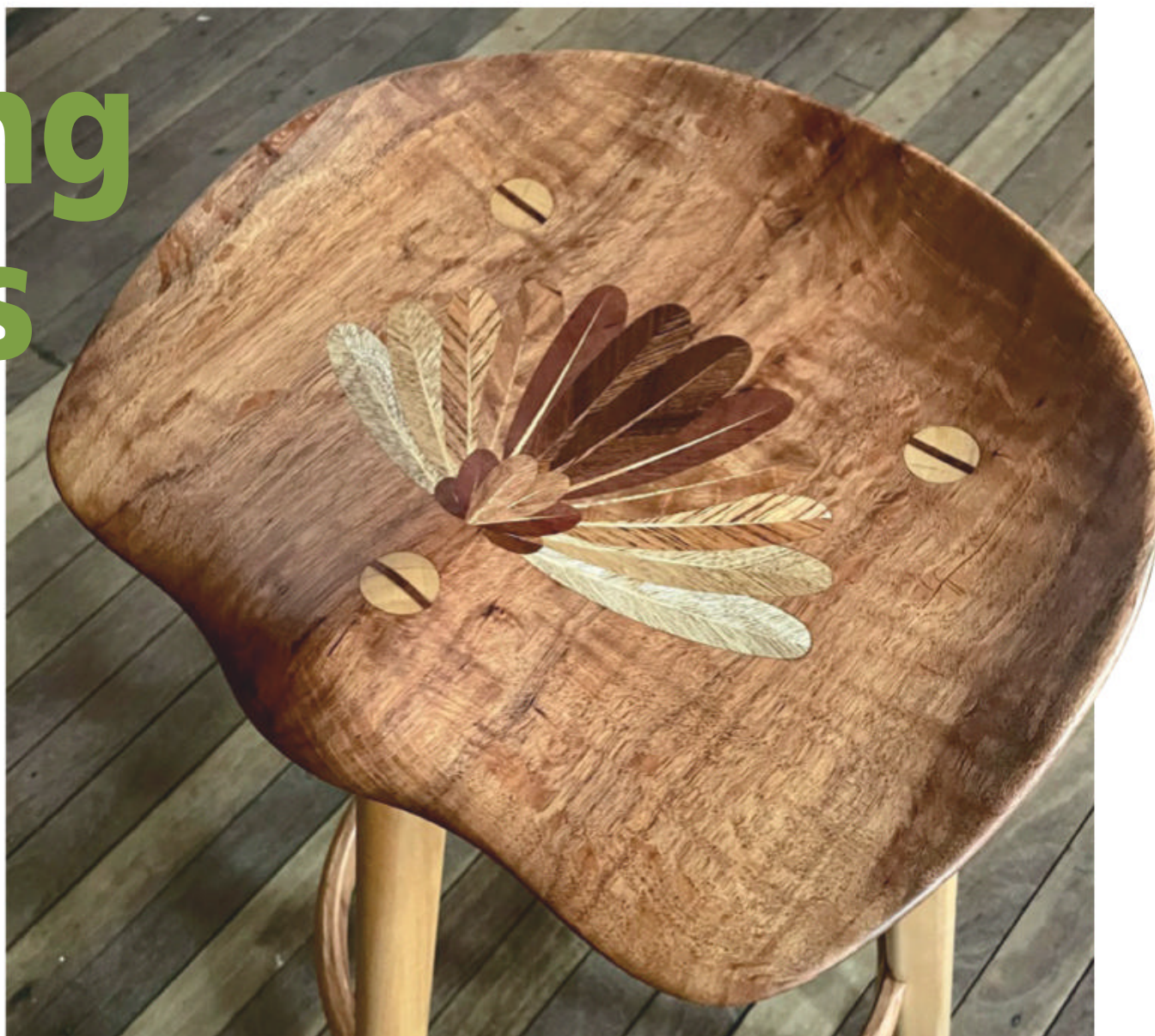
▲ Garan Hale "headed" the wedges on his magnificent Stella stool (see page 21) to avoid splitting the seat when the leg tenon expanded in its mortice.
