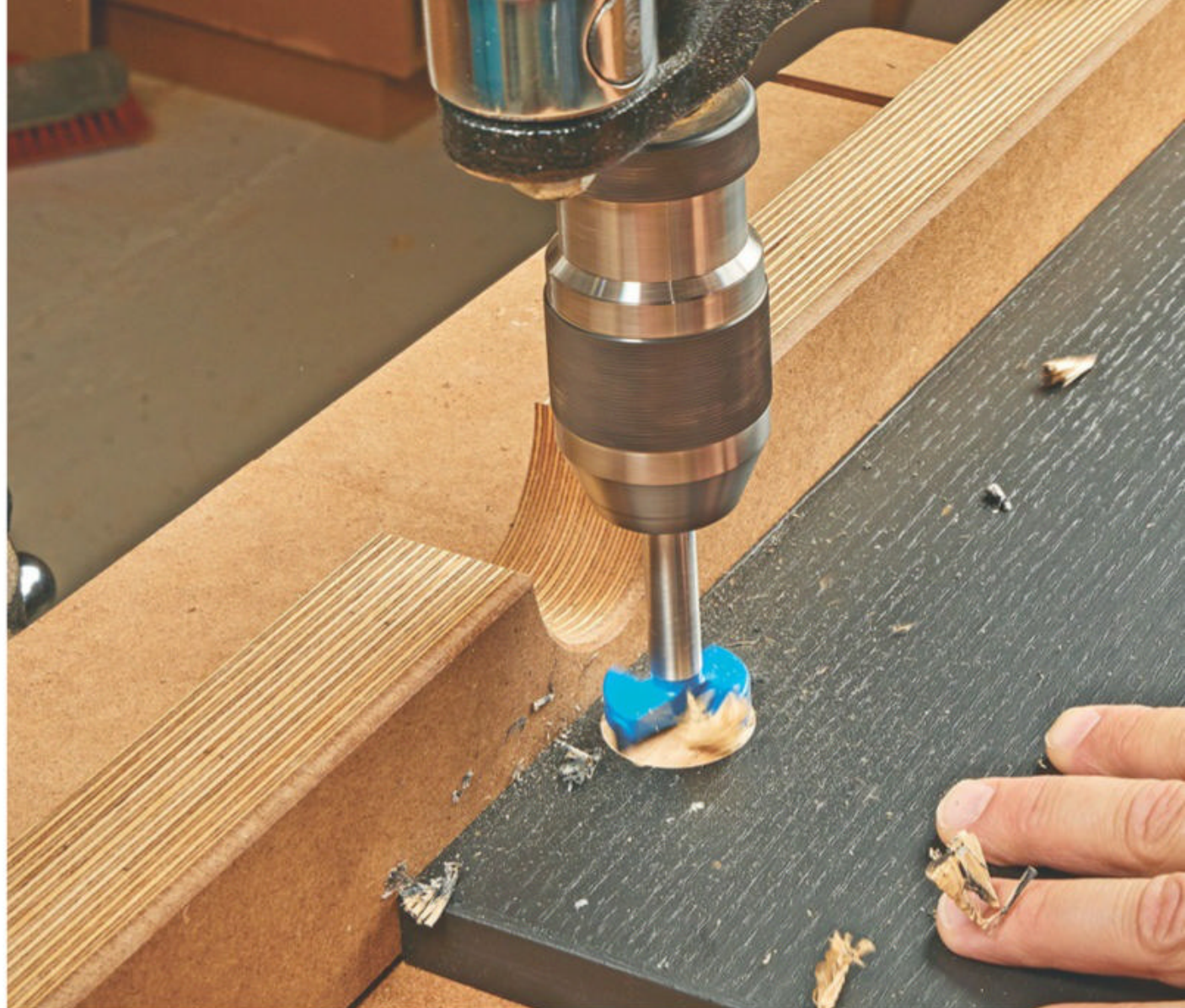
▲ A carbide Forstner bit lasts longer than high-speed steel bits. I find that running the bit at 1000-1500RPM results in a smooth, clean hole.
