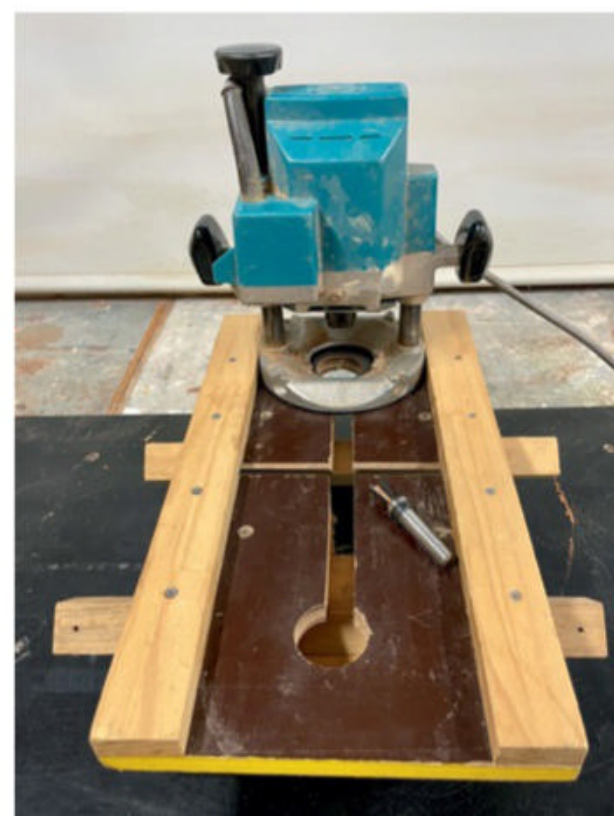
▲ The router sled needs to be a snug fit and have an entry and exit hole cut either end.
