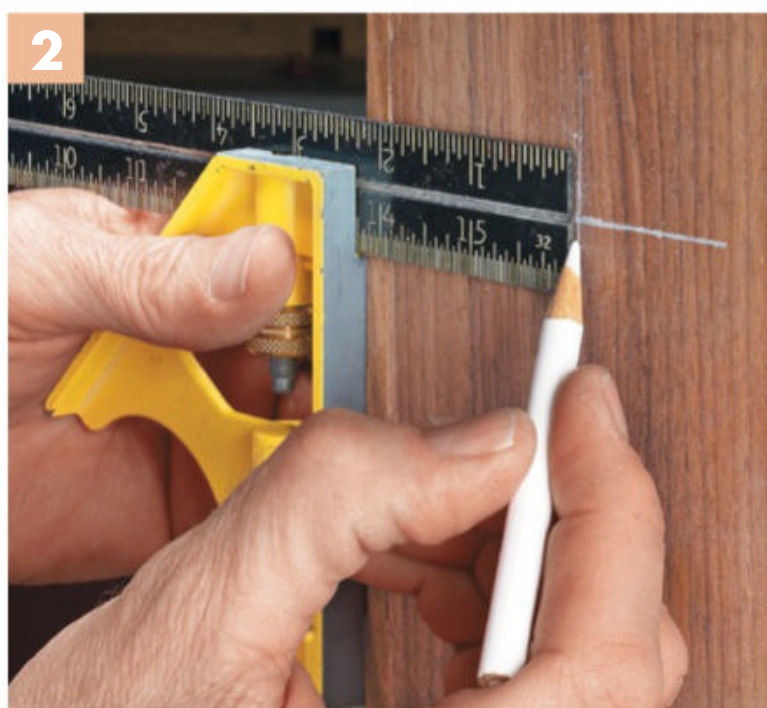
▲ After marking the vertical location of the centrepoint of the hinge, you can mark the offset based on whether the door is inset or overlay.
