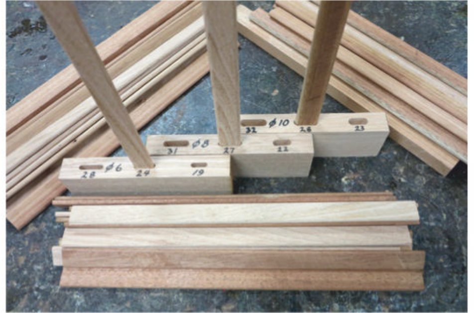
▲ Thinking outside the box had us playing around with screen sizes that matched the slots that the DOMINO machine can cut.
