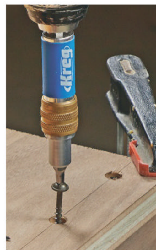
▲ The square bit works perfectly with any Kreg pocket screws. You can plug the hole with a 9.5mm dowel.
