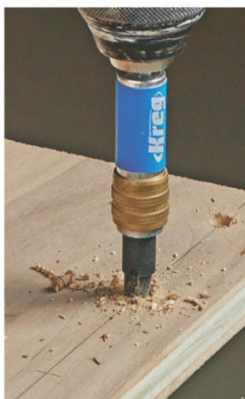
▲ First drill all of the counterbores to the desired depth. Then you can flip the bit to the driver side.
