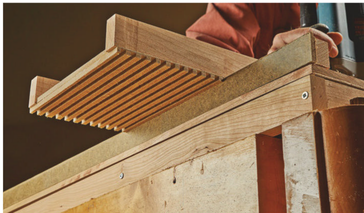
▲ Grooves in the bottom of the router carriage index on the Masonite carriage guide attached to the fixed jaw. This allows you to plane in a straight line and move across the board in even increments.
