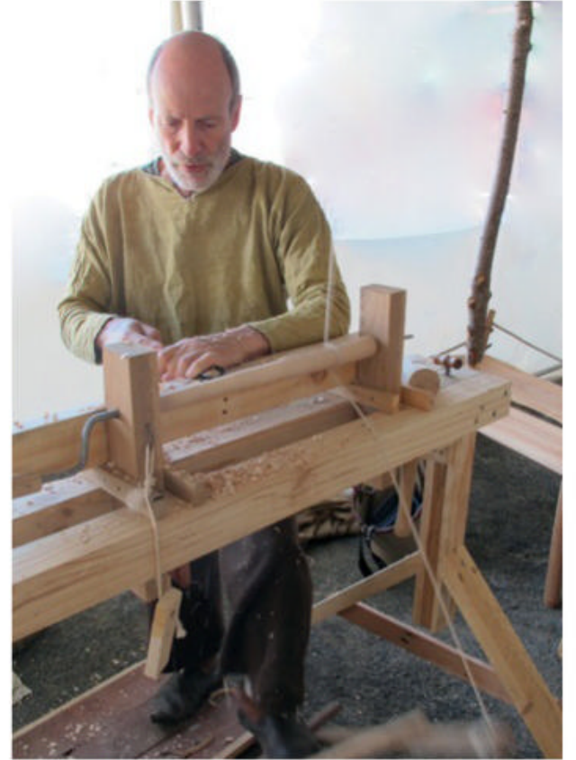
▲ Roy Davi (the Leura Bodger) at his pedal lathe turning chair spindles with a pole lathe.
