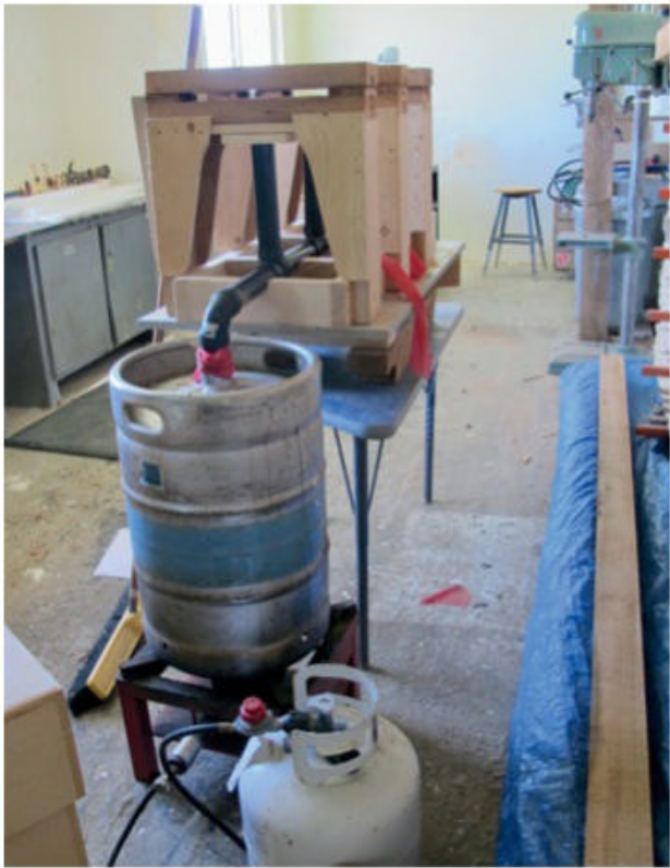
▲ The steaming jig set up and ready for action. The piped steam was focused on the kerf joint.
