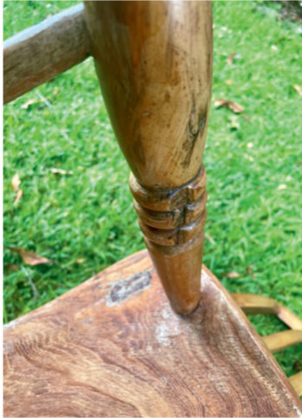
▲ Bodgers made the most of the material available. The defect in the leg was hidden by the chairmaker.
