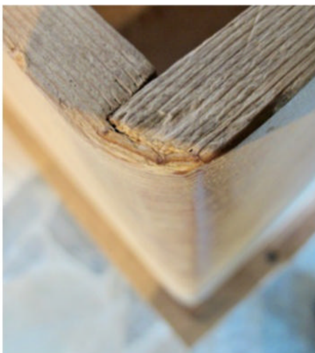
▲ An icon of coastal craftsmanship. The folded kerf joint can clearly be seen in this box.
