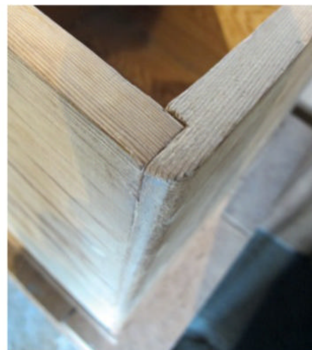
▲ The rebate and butt joint locks the box together and incorporates wooden pins.
