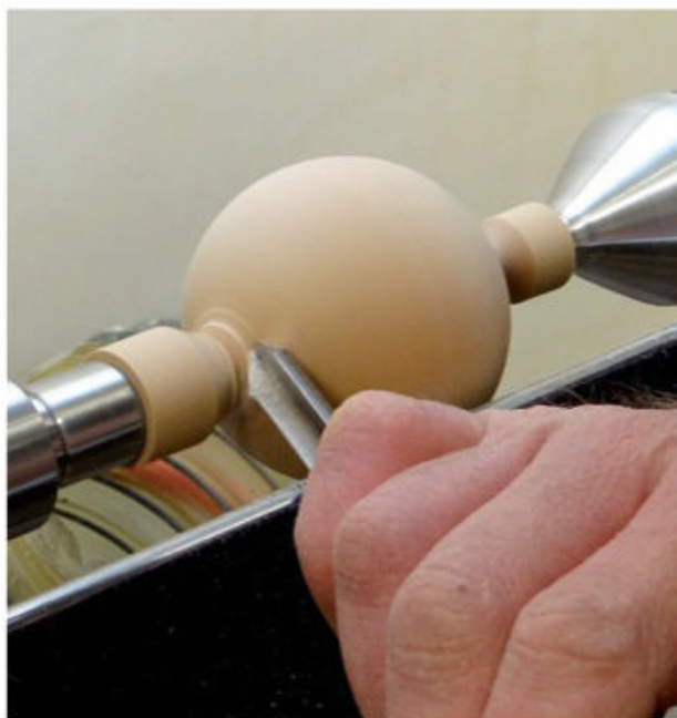
▲ Extending the curve by hand.
