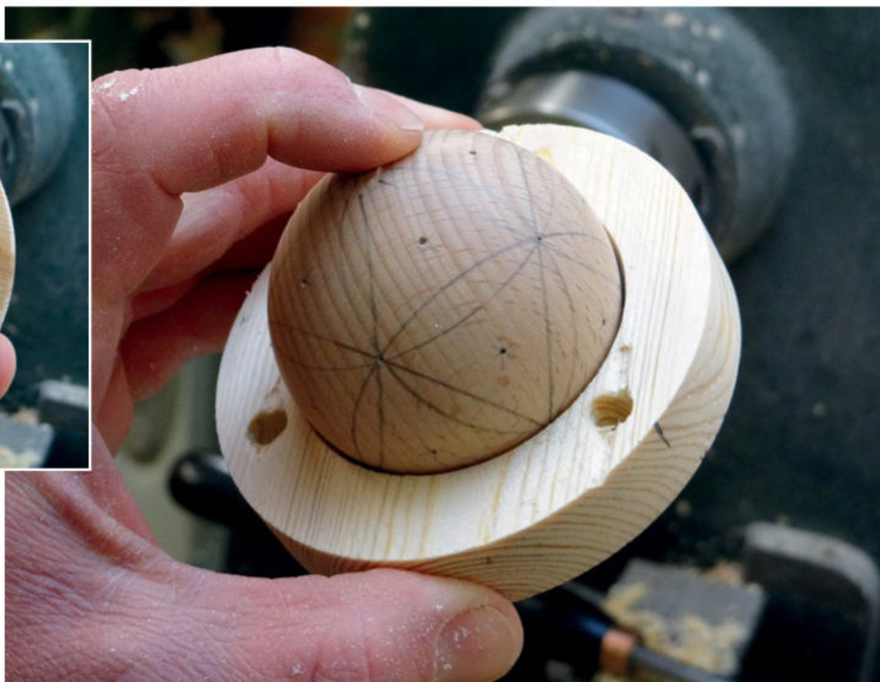
▲ Relieving the underside of the ring to hold the sphere in place.
