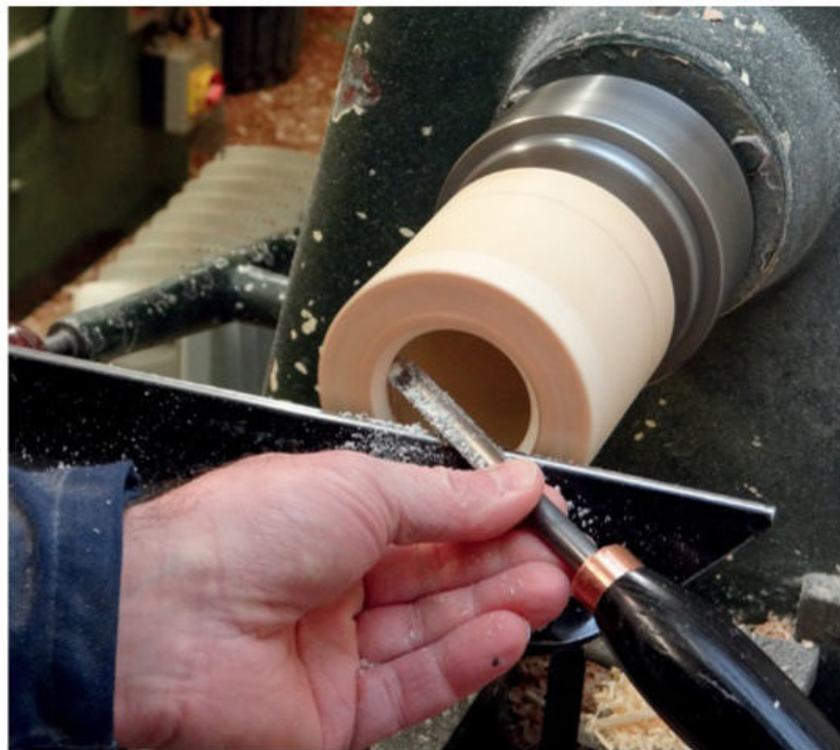
▲ Relieving the underside of the ring to hold the sphere in place.
