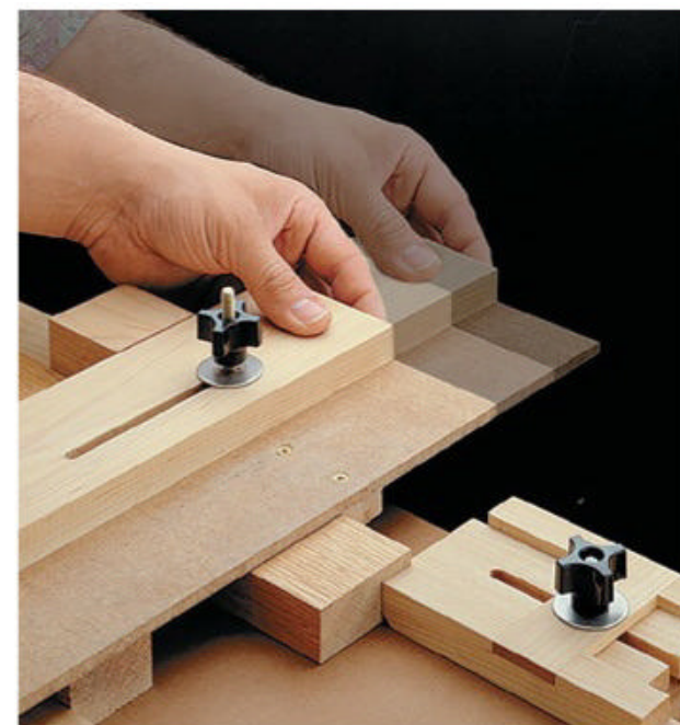
▲ Backup Block. To reduce chipout, slide the fence in so the backup block butts up against the workpiece.
