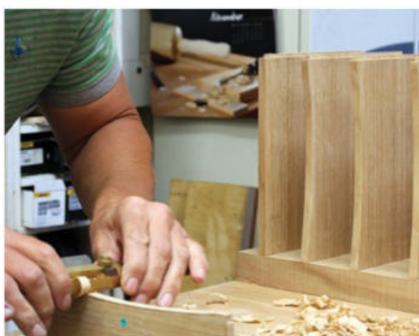
▲ Smoothing the curves to allow finger access to the drawers.
