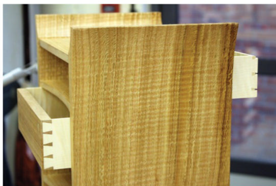
▲ The drawers being fitted from the rear to ensure a smooth piston fit.
