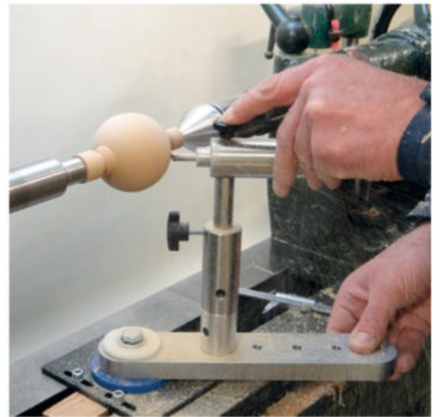
▲ Using a sphere jig.
