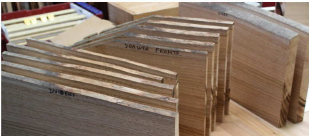
▲ Parts cut on the bandsaw and being allowed to settle.
