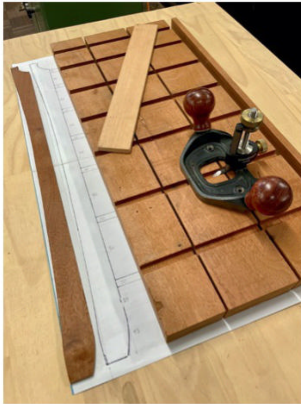
▲ Cleaning up each trench with a hand router removed inconsistencies.
