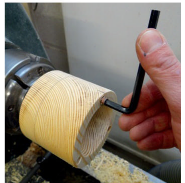
▲ Fitting the threaded inserts.
