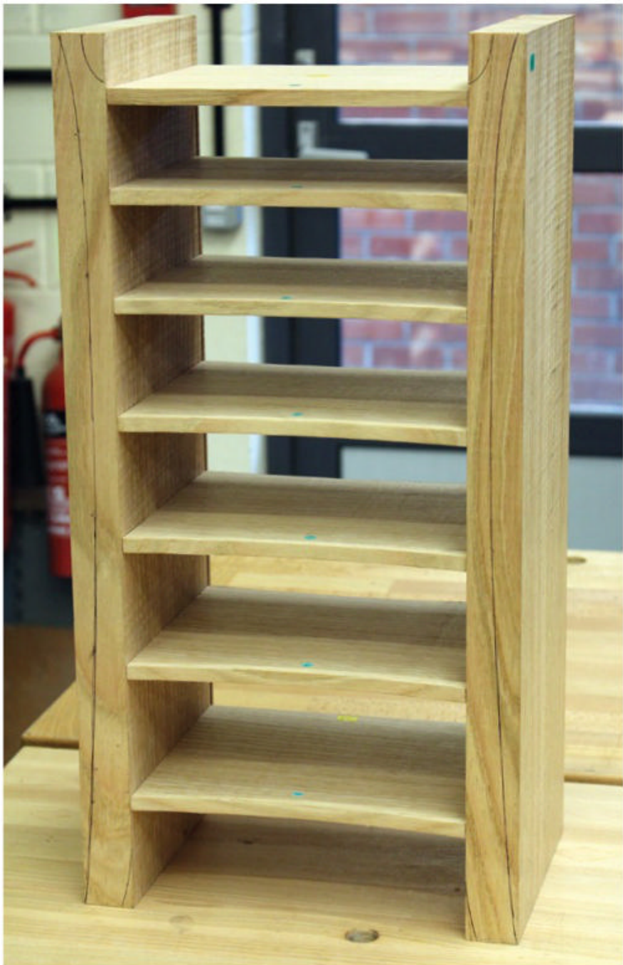
▲ A dry fit to check everything.
