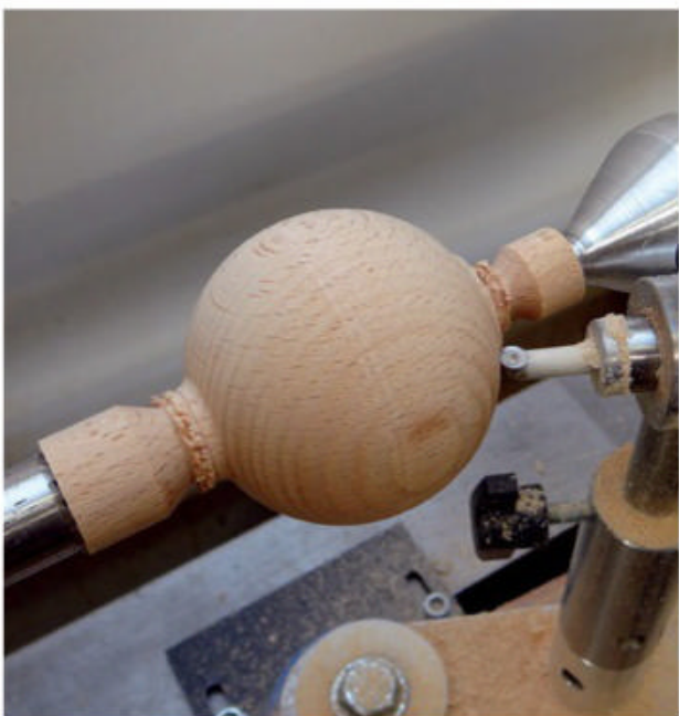
▲ The sphere jig can't get right round the ball.
