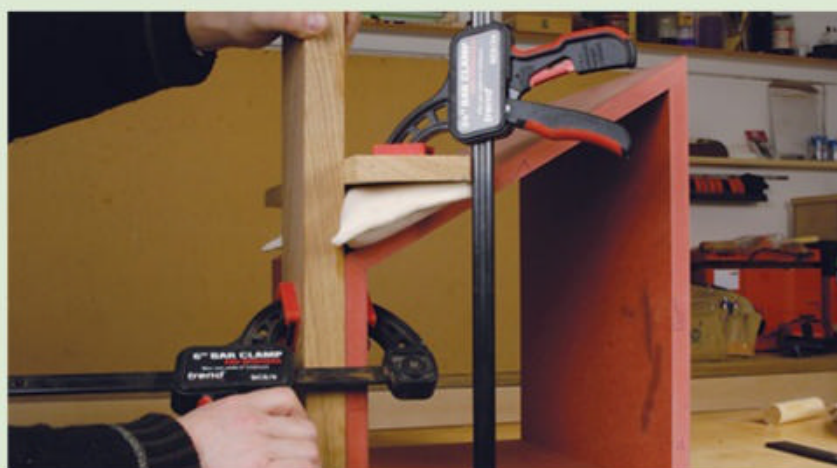
▲ Use a sandbag to fill the void between pressure blocks on angled joints.
