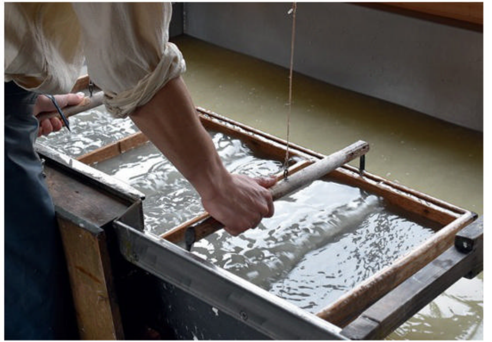
▲ After the mulberry fibres are boiled with soda, neri is added to evenly distribute the fibres as they settle onto a bamboo rack.
