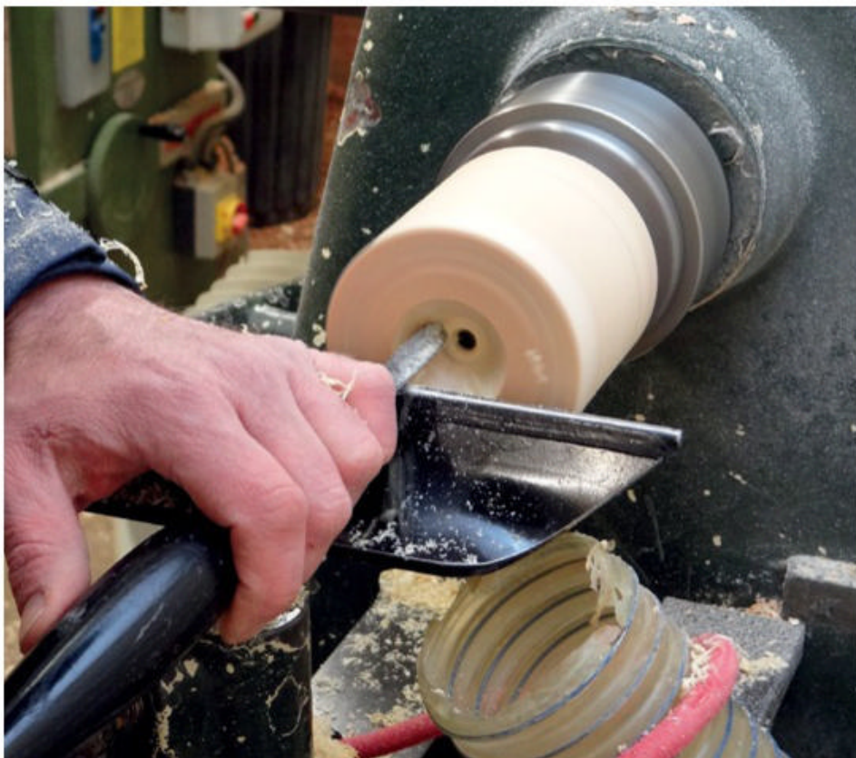
▲ Beginning to hollow the securing ring.
