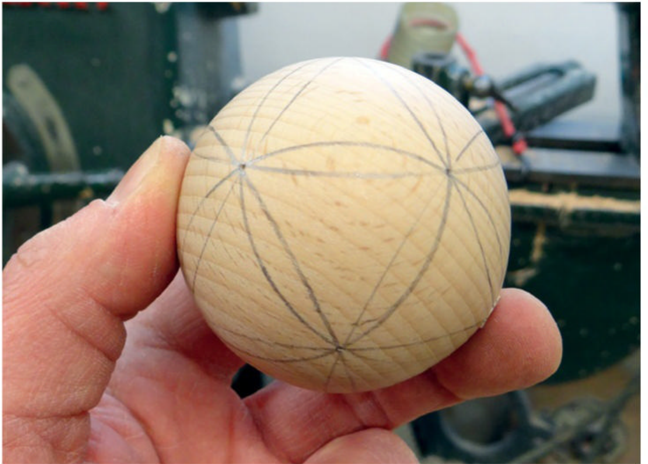
▲ There are triangles in the pattern and the centre of each needs finding.
