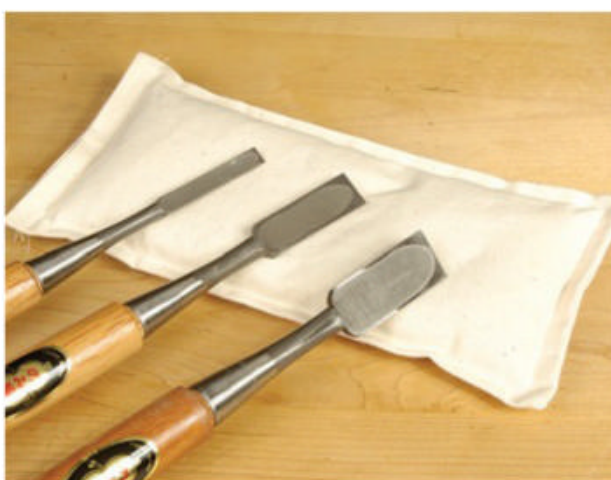
▲ When not in use as part of an efficient assembly line sandbags also make a very good rest for tools with a delicate edge.
