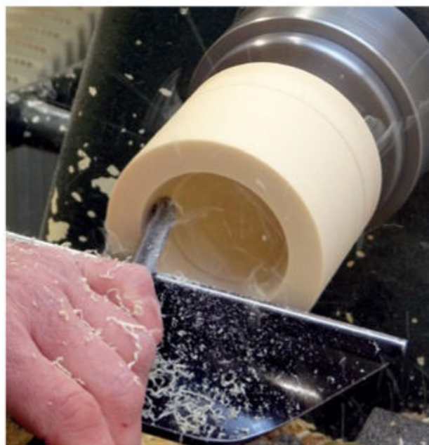
▲ Hollowing the pine block to hold the sphere.
