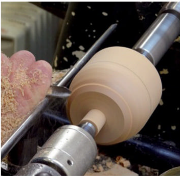
▲ Turning a ball freehand.
