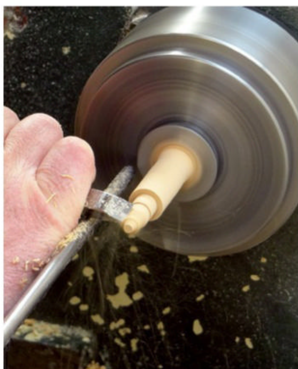
▲ Turning the point of the spike.
