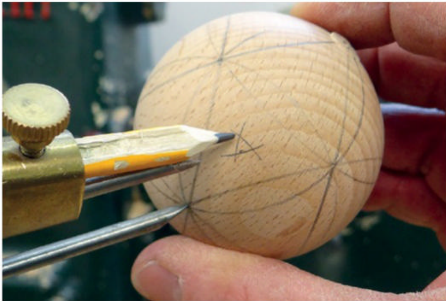
▲ Using my compass to find the centres of the triangles.
