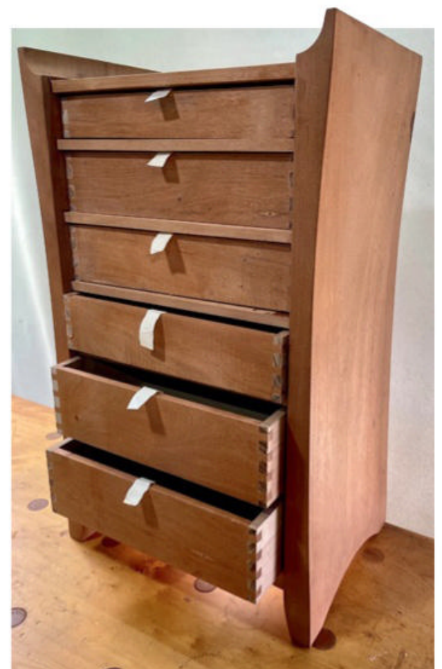
▲ I used masking tape as drawer pulls while tweaking the faceless drawers so they slid neatly in place.
