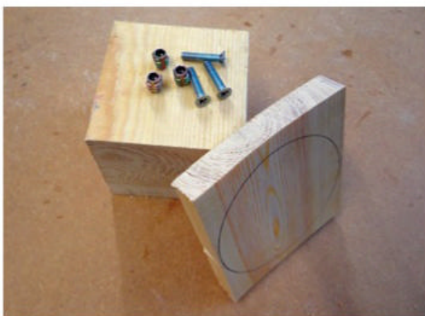
▲ Components for the sphere holding jig.
