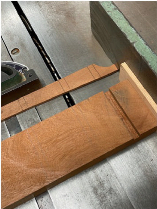
▲ The profiled rod sets the datum for the first cut, the spacer lines up the second.
