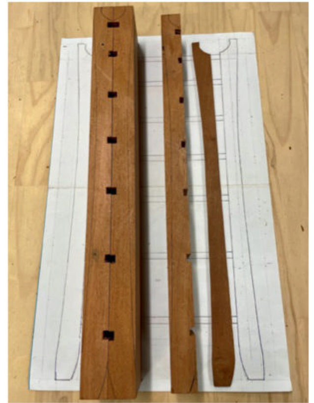
▲ After the trenches were dressed, it was time to trace and then cut the profiles on the bandsaw.
