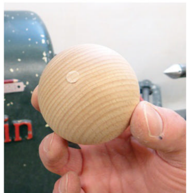
▲ The finished sphere showing the cut-off area.
