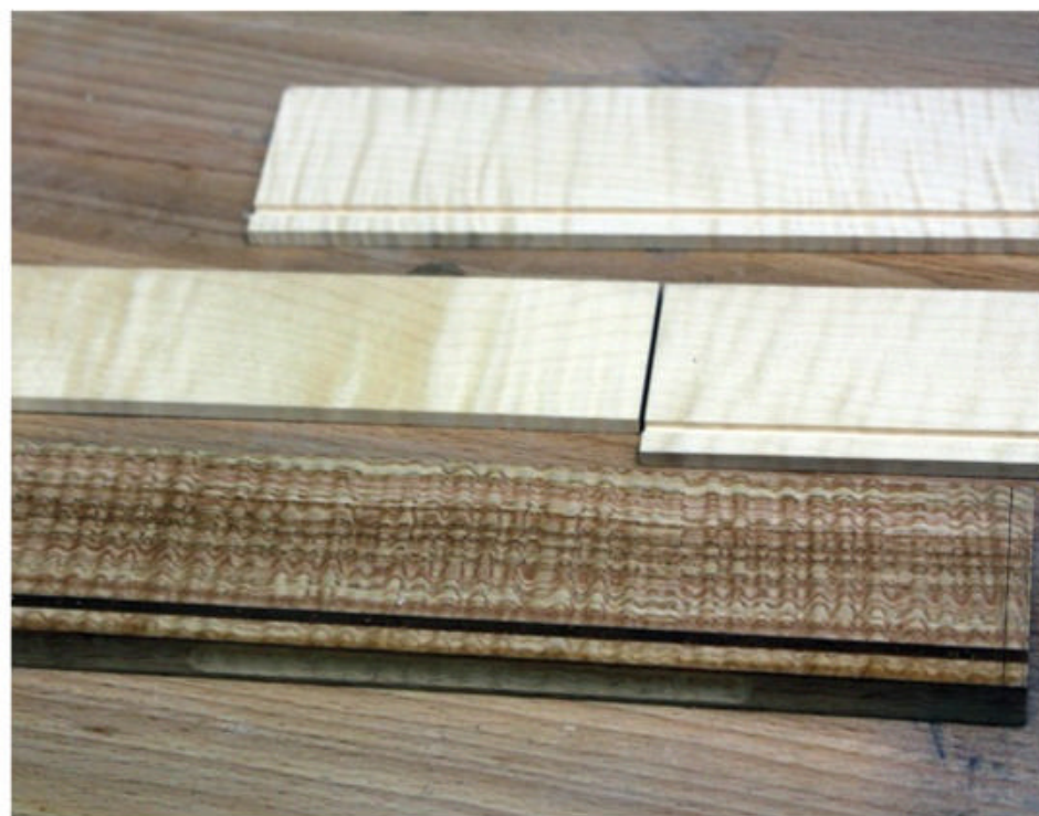
▲ Routed grooves in the drawer parts, note the narrower rear piece.
