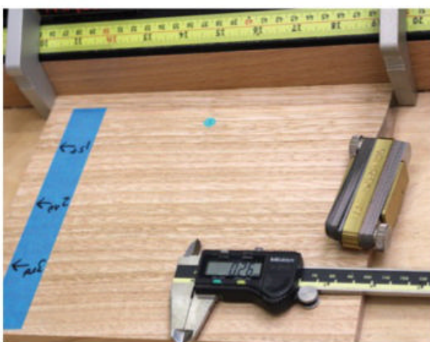
▲ Checking the taper against stops with a feeler gauge.
