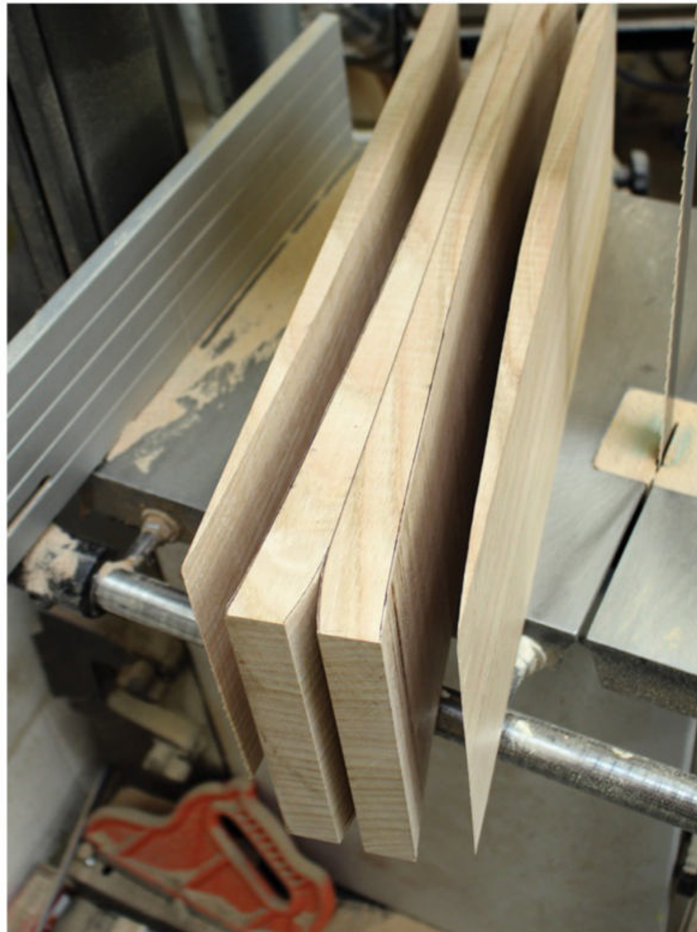
▲ Cutting curves on the bandsaw.
