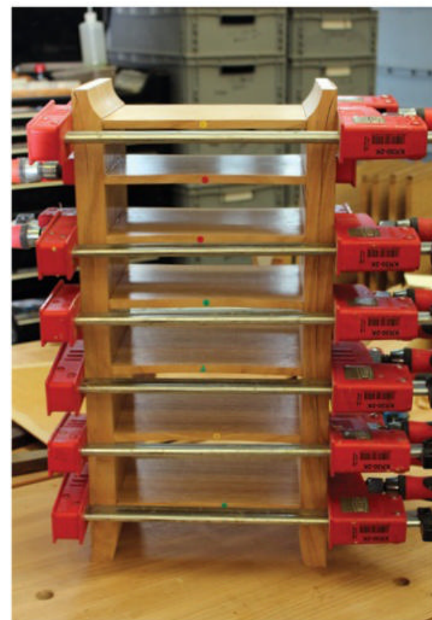
▲ Gluing up the carcass using the offcuts to keep the clamps square.
