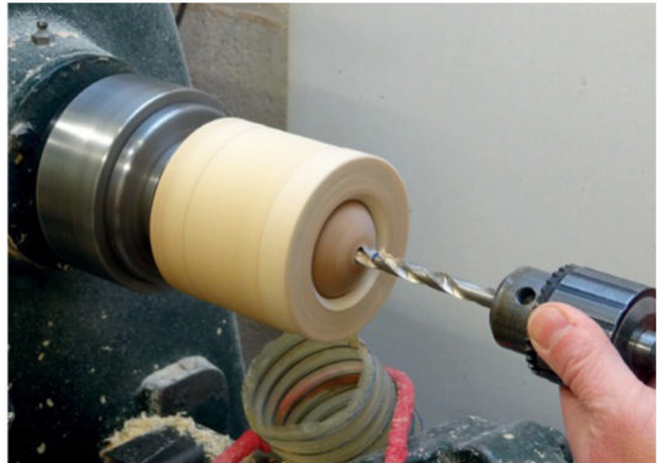
▲ Drilling the hole.
