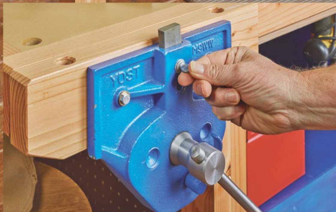
▲ The quick-release vice that's integrated into the front of the bench earns its keep in multiple ways. The wood vice face holds parts firmly in place without marring the surface. And the dog holes open a world of workholding possibilities.
