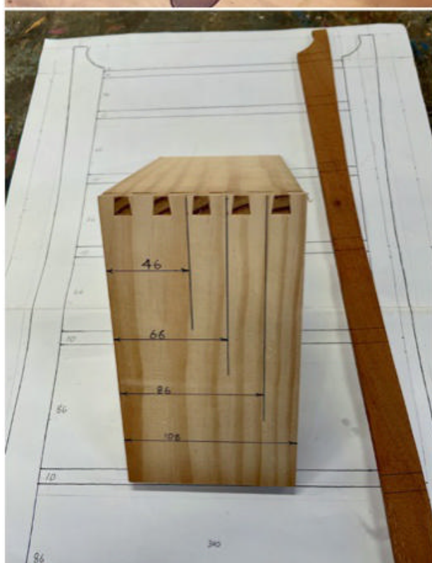
▲ The 10mm Gifkins dovetail example helped determine drawer size and cabinet height.
