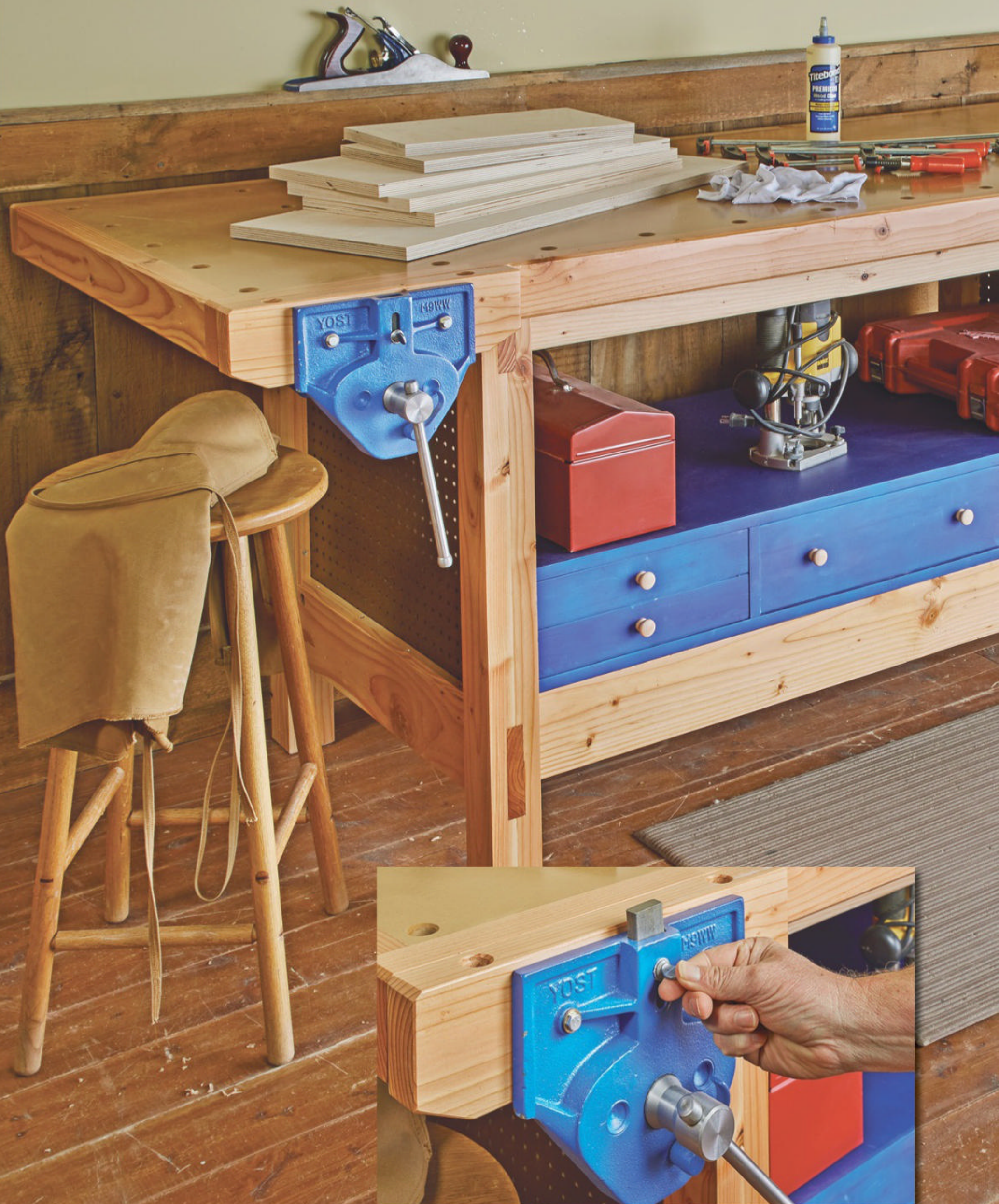
▲ The quick-release vice that's integrated into the front of the bench earns its keep in multiple ways. The wood vice face holds parts firmly in place without marring the surface. And the dog holes open a world of workholding possibilities.
