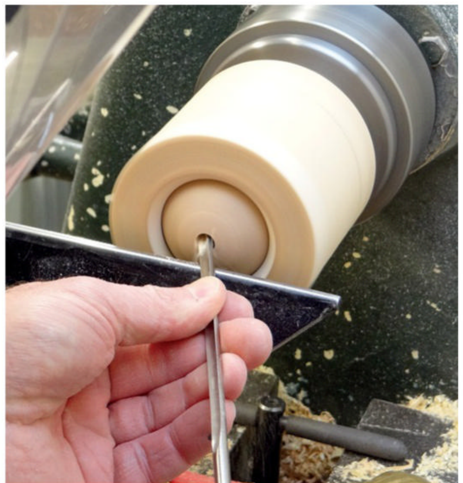
▲ Enlarging the hole with my 6mm spindle gouge.
