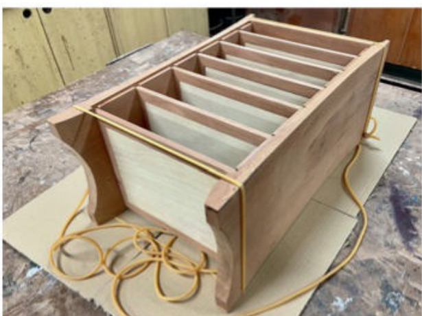
▲ Drawer supports and top installed, base curved and surgical tube at the ready for a test assembly.
