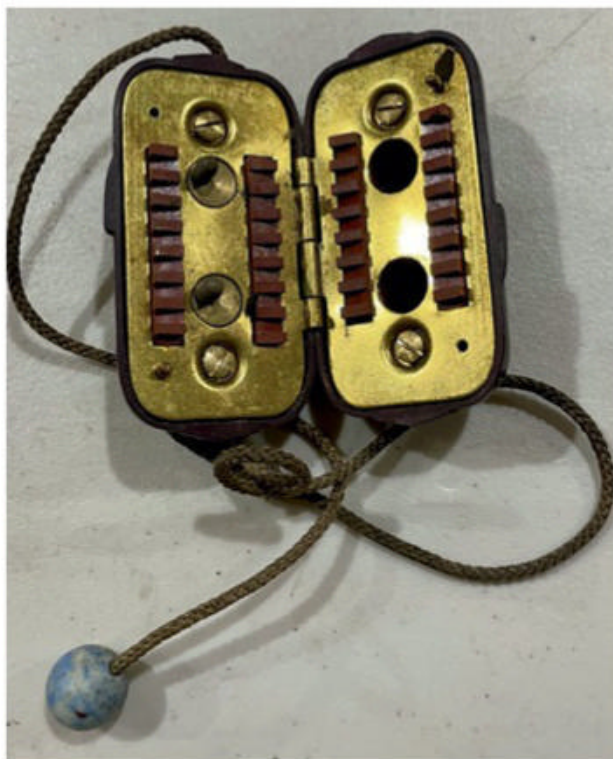
▲ A razor blade was positioned on the lugs, case closed, strings pulled, edges honed.
