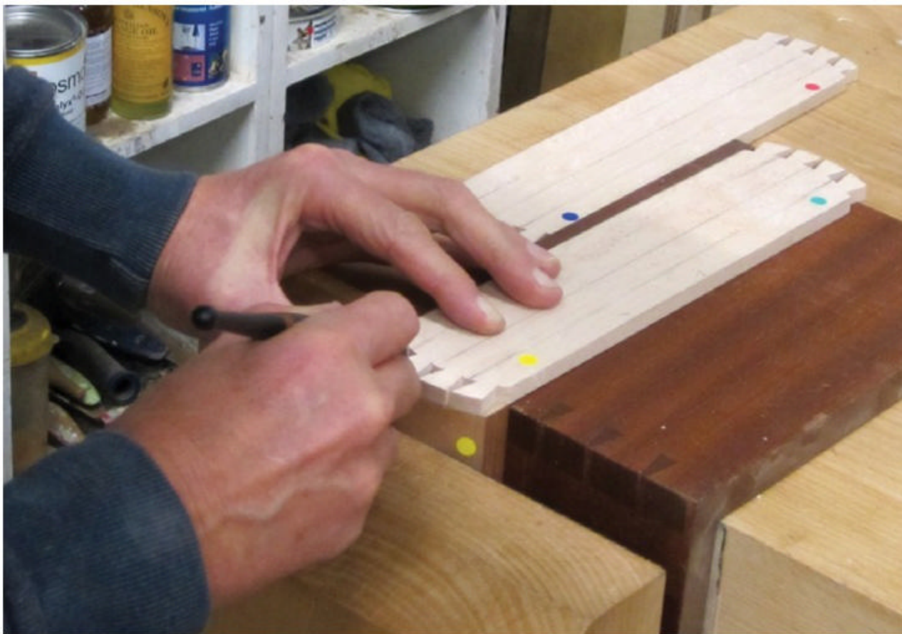
▲ Marking the pins using my alignment board.
