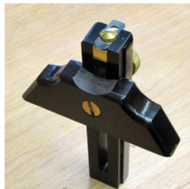
▲ My adapted cutting gauge filed to handle marking out the curves.
