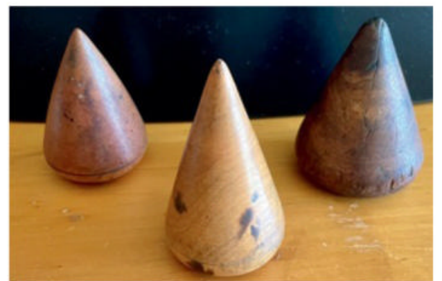
▲ When a plumber worked with lead pipes (plumbum) they used turnpins to create flange joints. Turnpins are fortuitously beautiful objects that have become collectable items in their own right.
