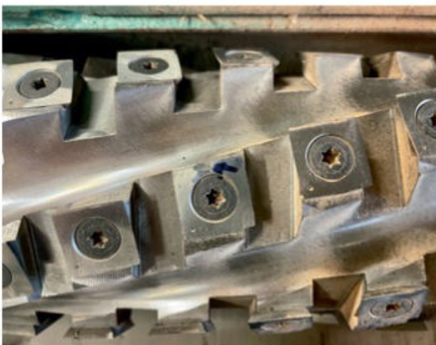
▲ After two years of use (and abuse) the cutting head has just one chipped insert (notice the witness mark bottom left).
