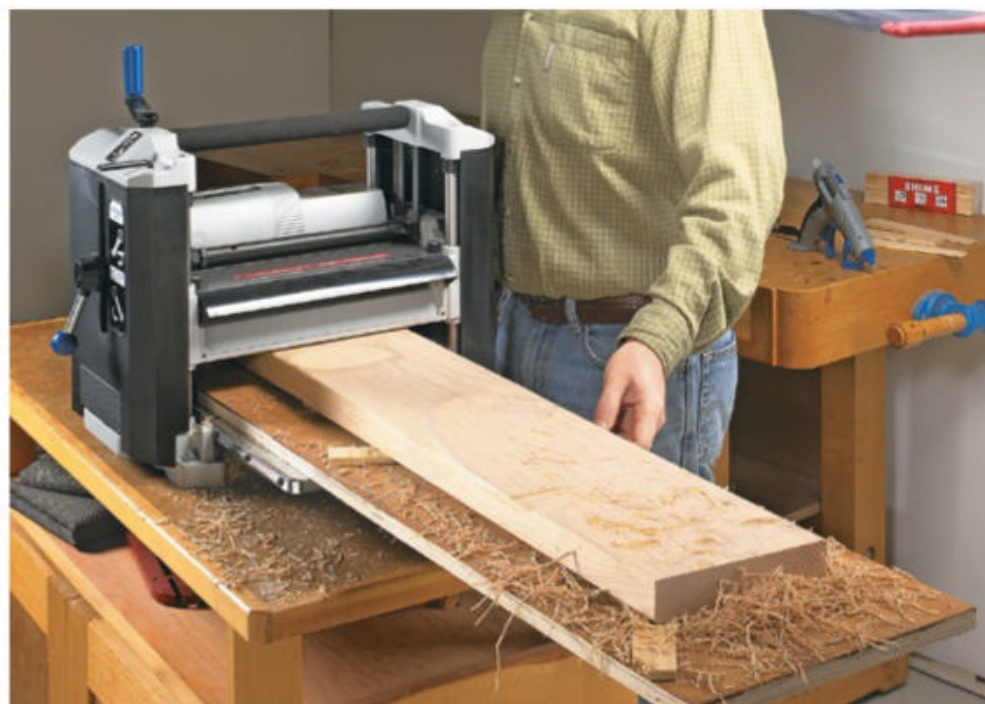
▲ You can flatten one face of a board using a thickness planer by supporting it on a sled. Thin wedges or shims keep the workpiece from rocking during the process.
