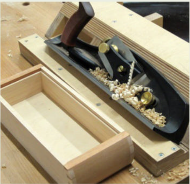
▲ The lining being shot on a mitre shooting board.
