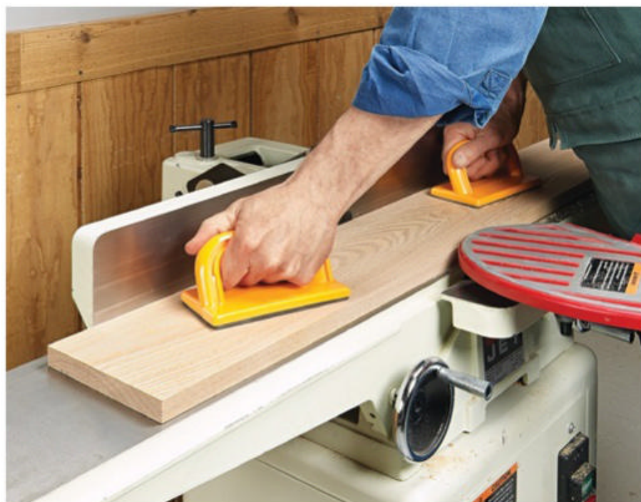
▲ A jointer can flatten the face of a board that's as wide as the cutterhead or narrower. Use even pressure with push pads to remove cupping and twist.
