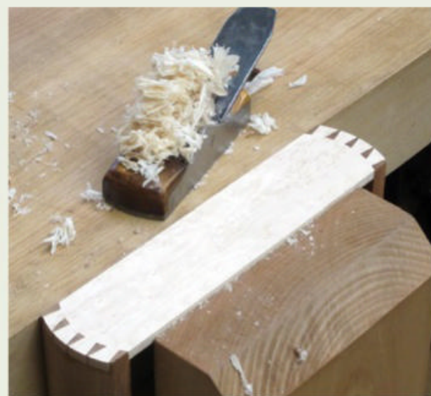
▲ Cleaning up the sides including removing all trace of the base lines.
