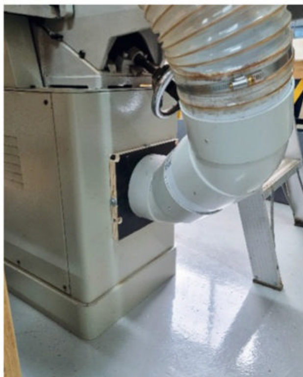
▲ The jointer required a 150mm step-down fitting to connect to the system.
