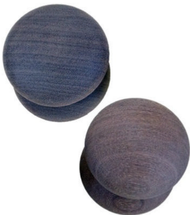
▲ The difference between the cross grain (top) and end grain (bottom) knobs.
