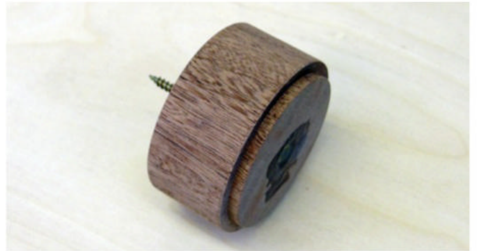
▲ The screw chuck ready for action.
