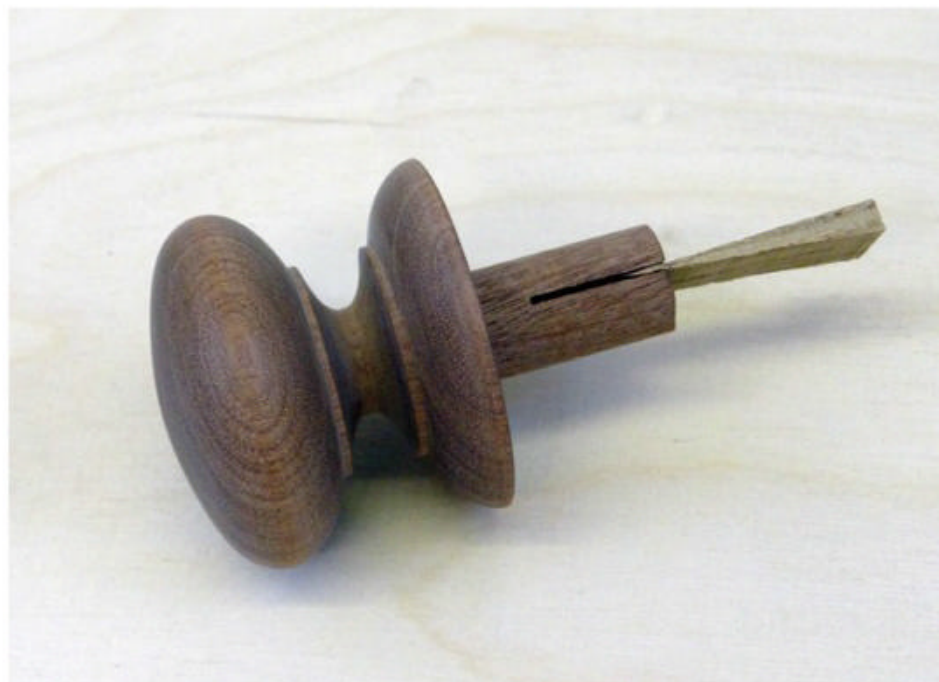
▲ The wedged tenon before fitting.
