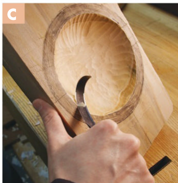
▲ For fine, trim cuts, extend your hand with your thumb protected. Choke up on the handle for maximum control.
