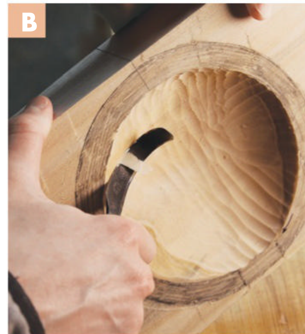
▲ Another option is to pull the knife using your dominant hand. Keep your thumb tucked below and away from the path of the blade.
