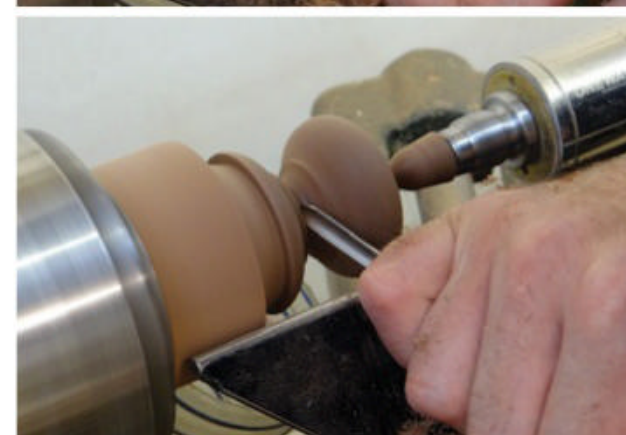
▲ The shaping process of the cross grain knob with the wing of the spindle gouge.
