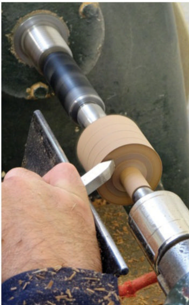
▲ Slicing the base of the knob to form a clean undercut.
