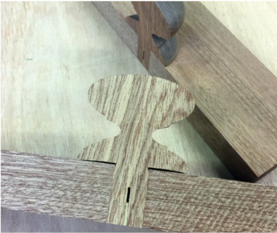
▲ Cross section of a wedged tenon fixing.
