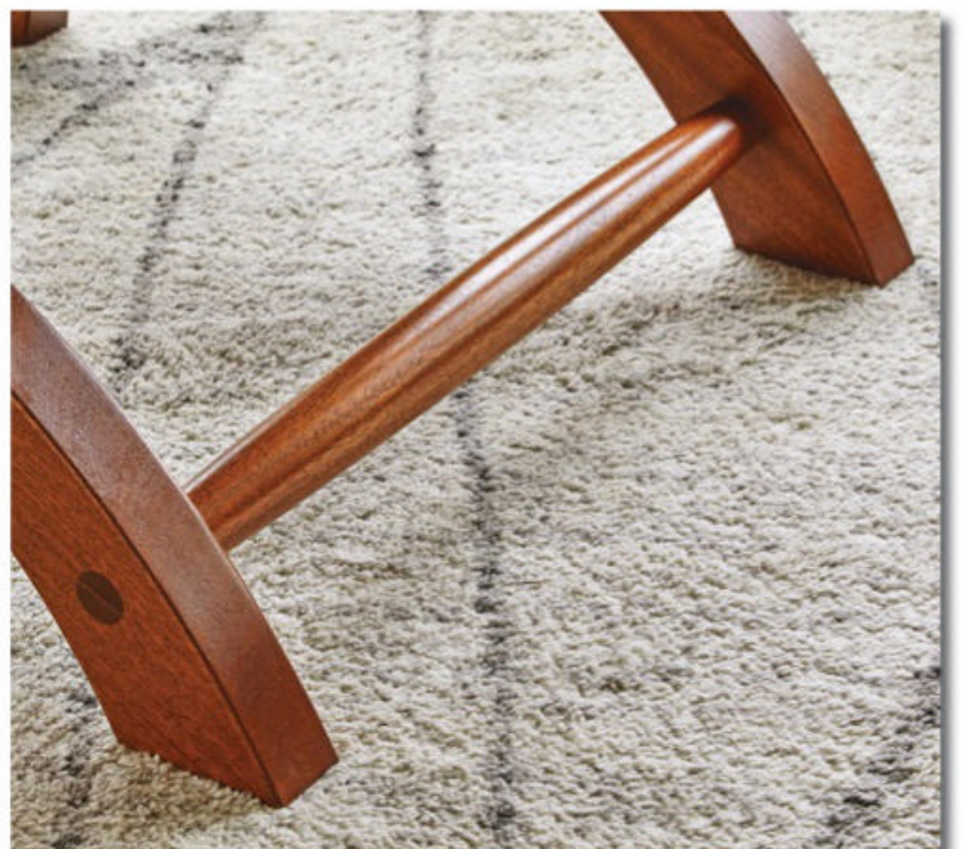
▲ The tapered rails are turned on the lathe (they could be shaped with a spokeshave) and reflect and echo the curves that make this chair so organic and inviting.
