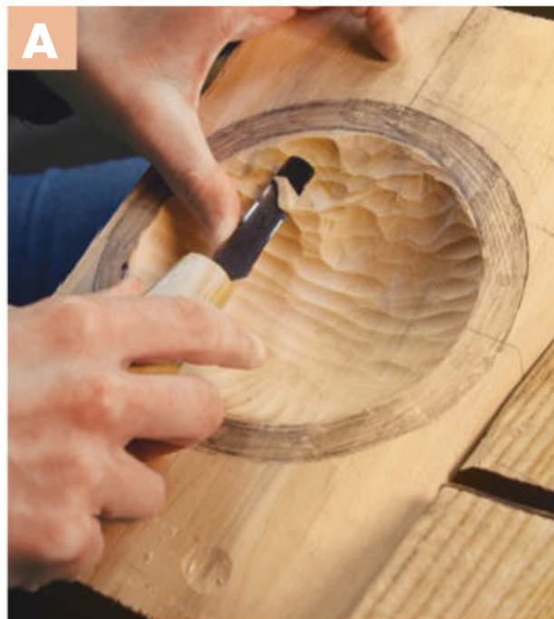
▲ Working across the grain allows you to remove material quickly. Use the thumb on your other hand to drive the blade forward.
