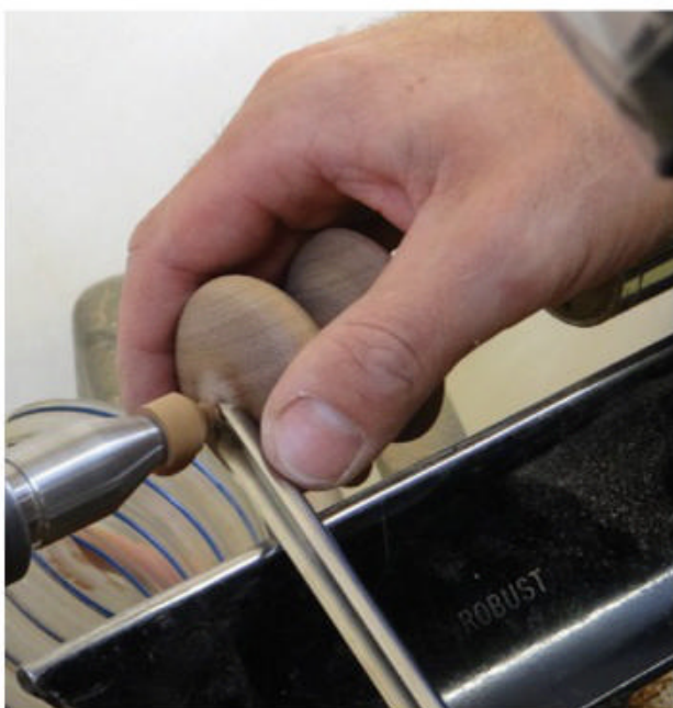
▲ Parting off with the spindle gouge.
