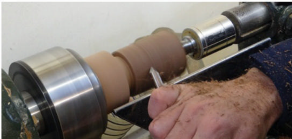
▲ Roughing out with the spindle gouge.
