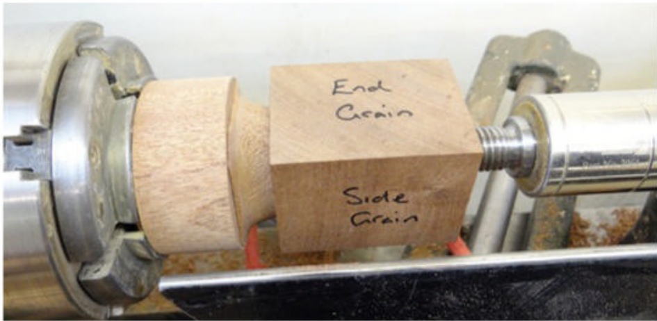
▲ Cross grain knob mounted on the screw chuck.
