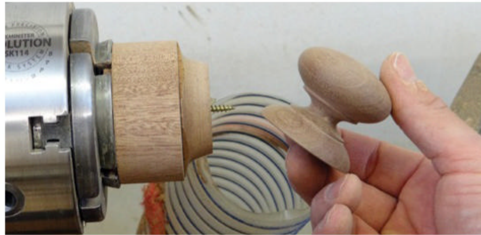
▲ The cross-grain knob and screw chuck, showing the spacer block.
