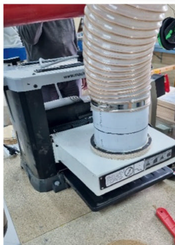
▲ The thickener has a direct connection to the 150mm extraction hose.
