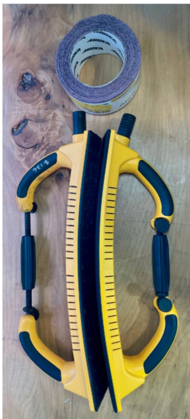
▲ The Mirka flexible file board is perfectly suited to boatbuilding and can be adjusted to match the profile of a hull.
