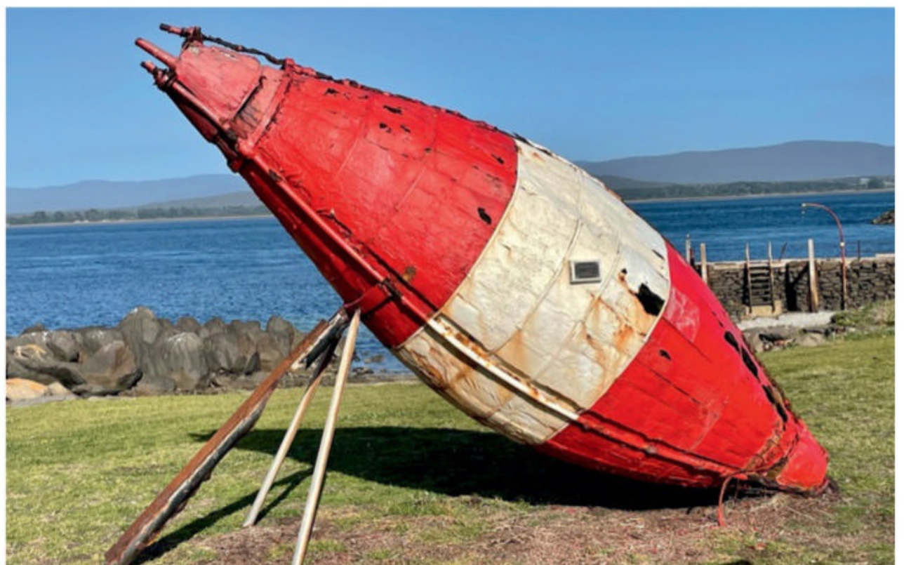
▲ Huon pine marker bouys were used on the Tamar River from 1835 to 1960. Coopers crafted these amazing symmetrical bouys out of 19mm-thick double tapered staves.
