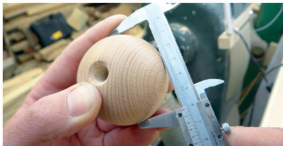
▲ Checking the size of the finished tama.
