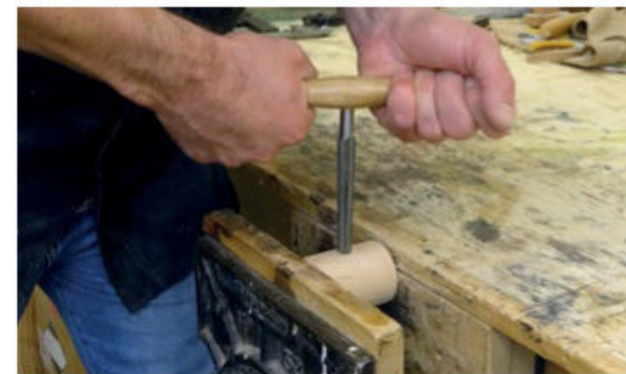
▲ Reaming the hole in the sarado.
