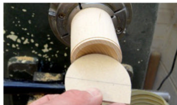
▲ Checking the cup is deeper than the ball with a template.
