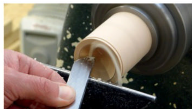
▲ Refining the cup with a negative rake scraper.
