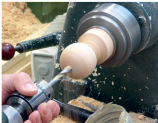
▲ Drilling the hole in the tama.
