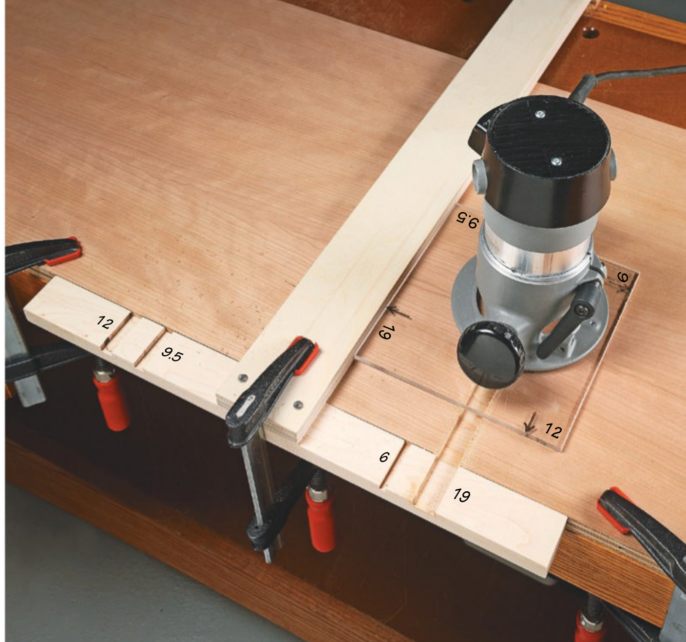
▲ A workshop-made T-square makes easy work of routing trenches of four different widths. The offset auxiliary router baseplate is the key. Each of the four edges of the baseplate positions the centreline of the trench in a different location.
