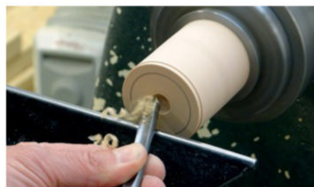
▲ Beginning to turn the cup with a spindle gouge.
