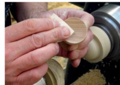
▲ Sanding the sharp edges of the cups.
