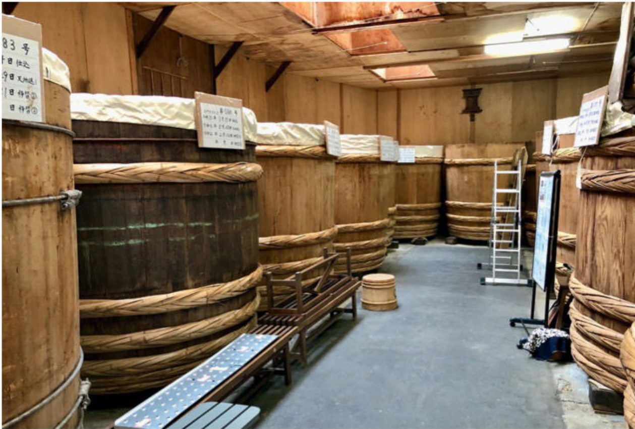
▲ The Ishii miso brewery has been making miso in tall wooden vats since 1868. Traditional braided bamboo hoops are now replaced with threaded steel rods.
