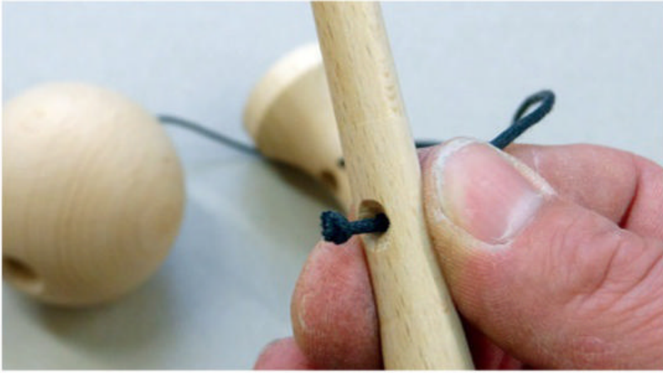
▲ The knot sits in the countersink on the ken.
