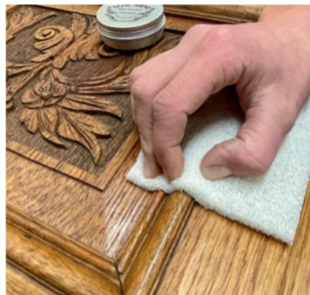
▲ White "0000" synthetic steel wool pads don't shred (unlike steel wool) when waxing a finish.
