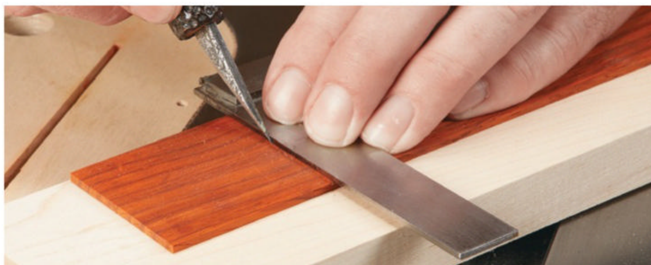
▲ For thin, splintery woods, lightly scoring the cutline with a knife reduces chipping from the saw blade.
