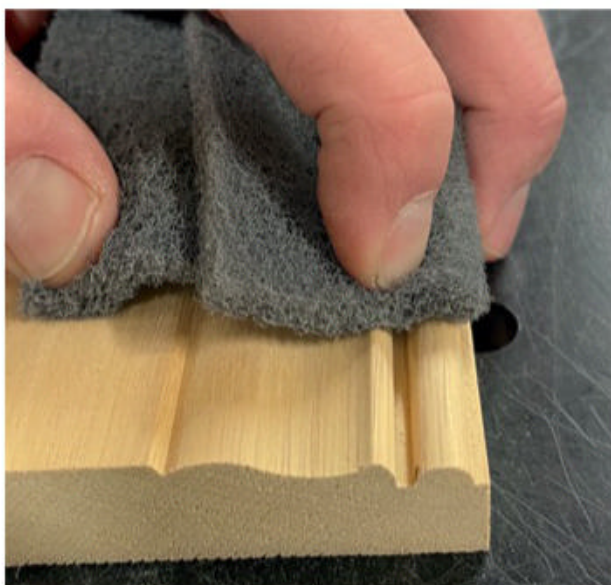
▲ Grey synthetic "000" steel wool pads readily conform to complex profiles and don't rust.
