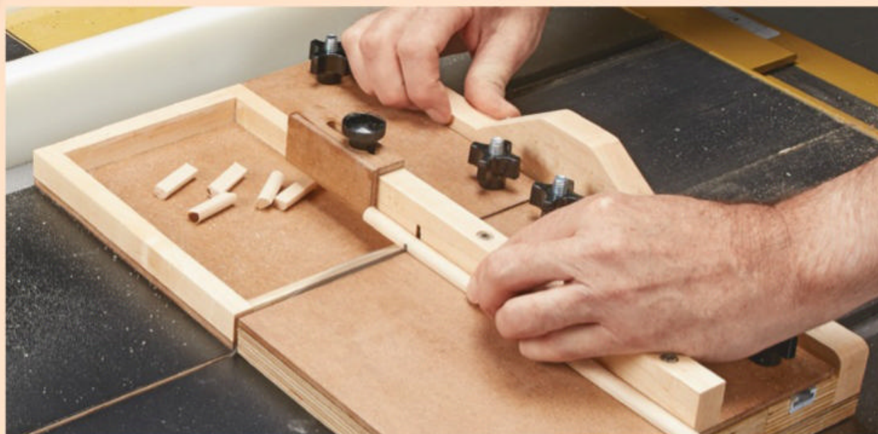
▲ A high tooth-count blade coupled with the catch tray on the sled keeps small parts from wandering away while you work. This version attaches to the T-track in the sled fence and uses T-bolts and knobs to hold it in place.
