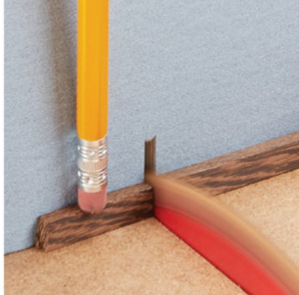
▲ A pencil eraser easily holds workpieces in place while you're making cuts. The eraser is grippy enough to give good control of the part.
