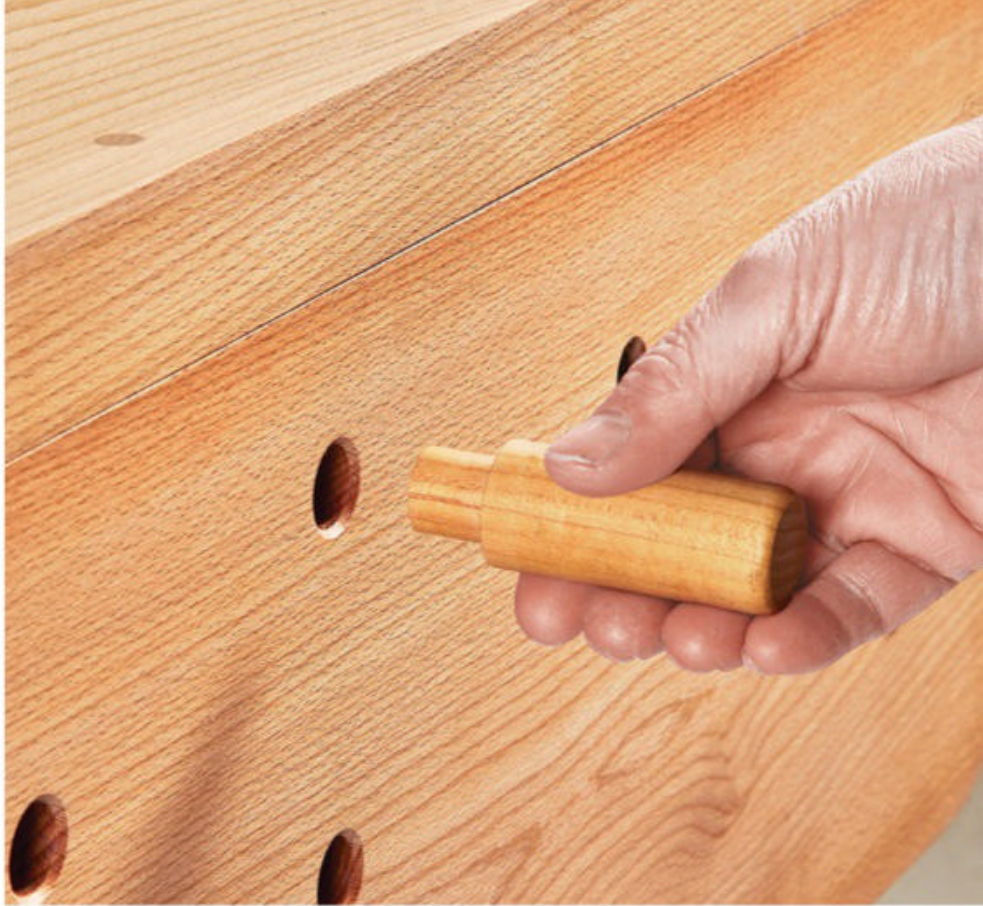
▲ The holes in the apron provide you with many ways to hold your workpieces. From jigs, holdfasts, to the simple peg you see here, they're all ready to give you a hand.
