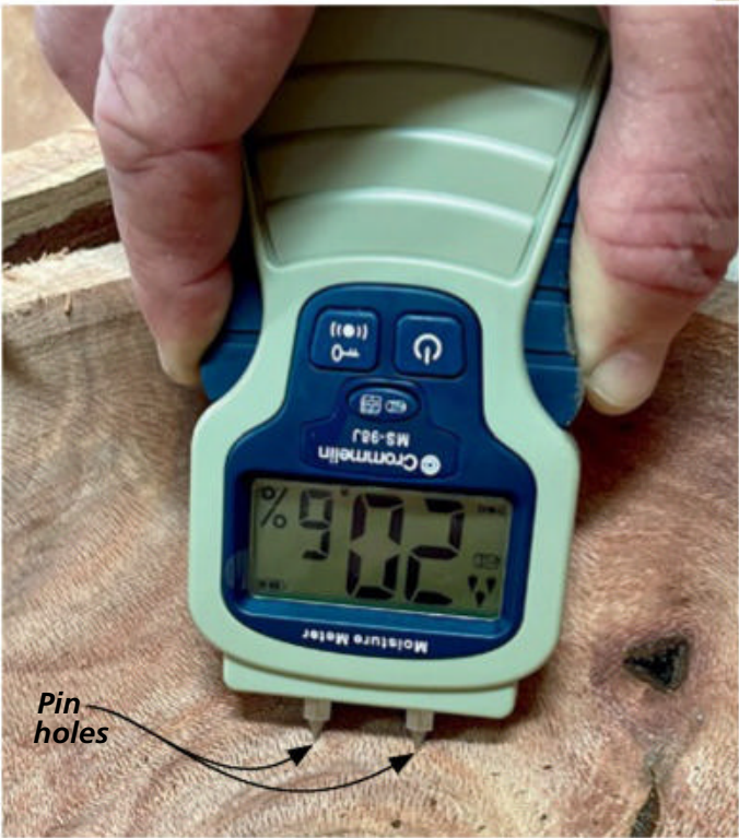
▲ Pin meters measure moisture with the use of two pins, and Crommelin claims their pin meter is accurate within two percentage points.
