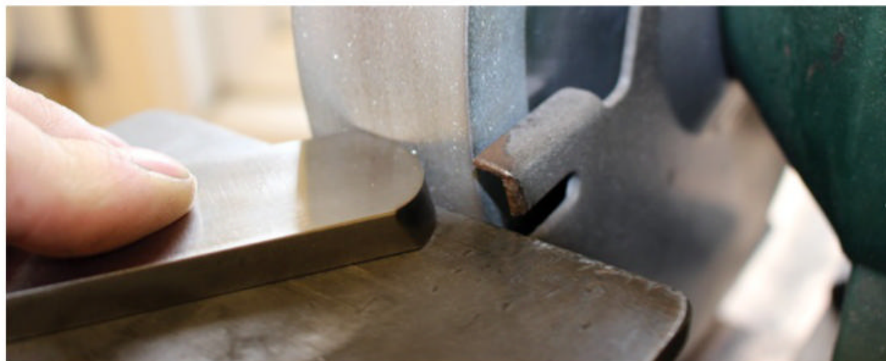
▲ Sharpening the scraper with the cutting edge downwards on the support table.
