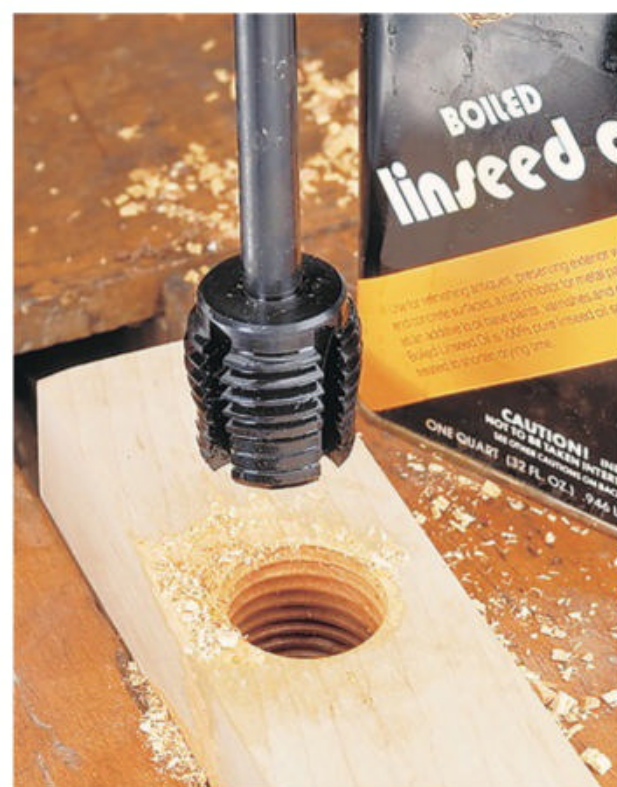
▲ A sharp tap combined with a closed-grain stock leaves crisp threads ready for a mate.
