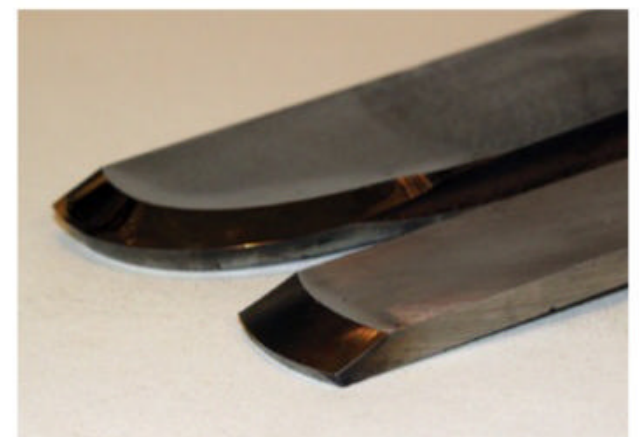
▲ Negative rake scrapers.
