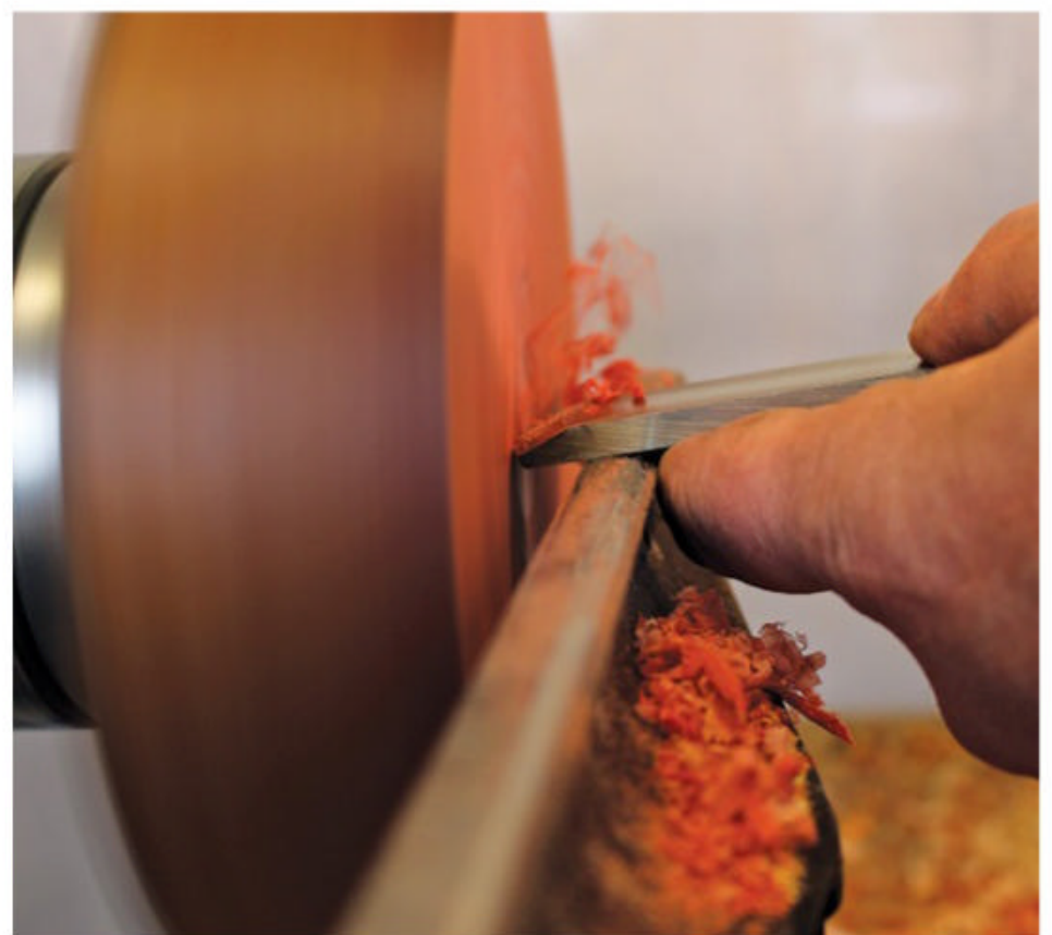
▲ Domed negative rake scraper in use.
