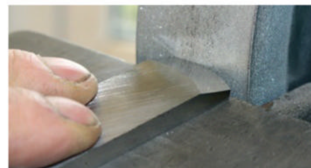
▲ Sharpening a negative rake scraper.
