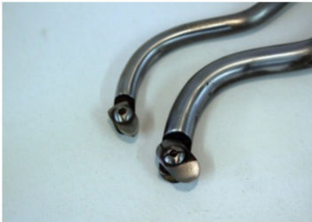
▲ Goose/swan-neck hollowing scrapers.
