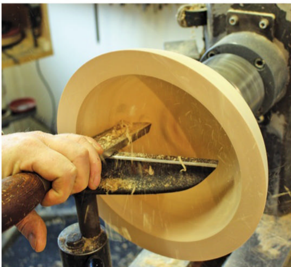
▲ Negative-rake scraper used on the inside of the bowl.
