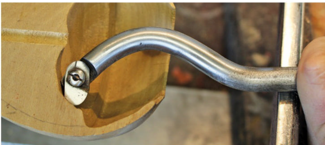
▲ Goose/swan-neck scraper allows you to hollow through restricted openings.
