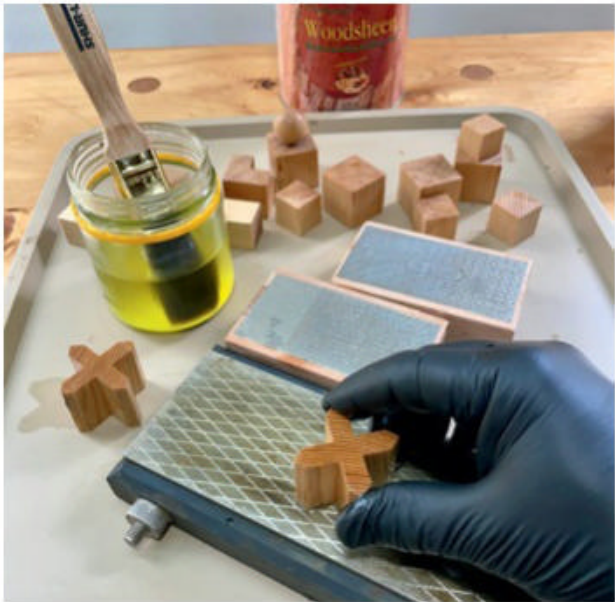
▲ Diamond plates are made perfectly flat, just right for truing and burnishing end grain.
