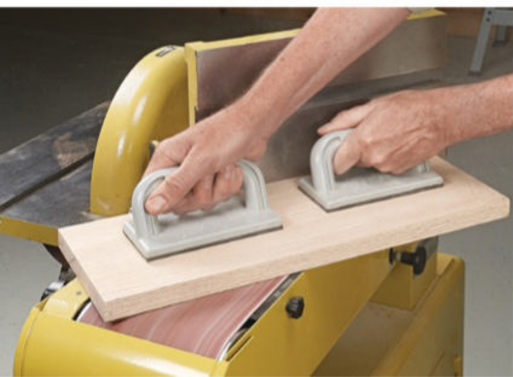
▲ The fence can pivot so it's at an angle to the belt. This allows you to put a flat face on wider boards and panels.
