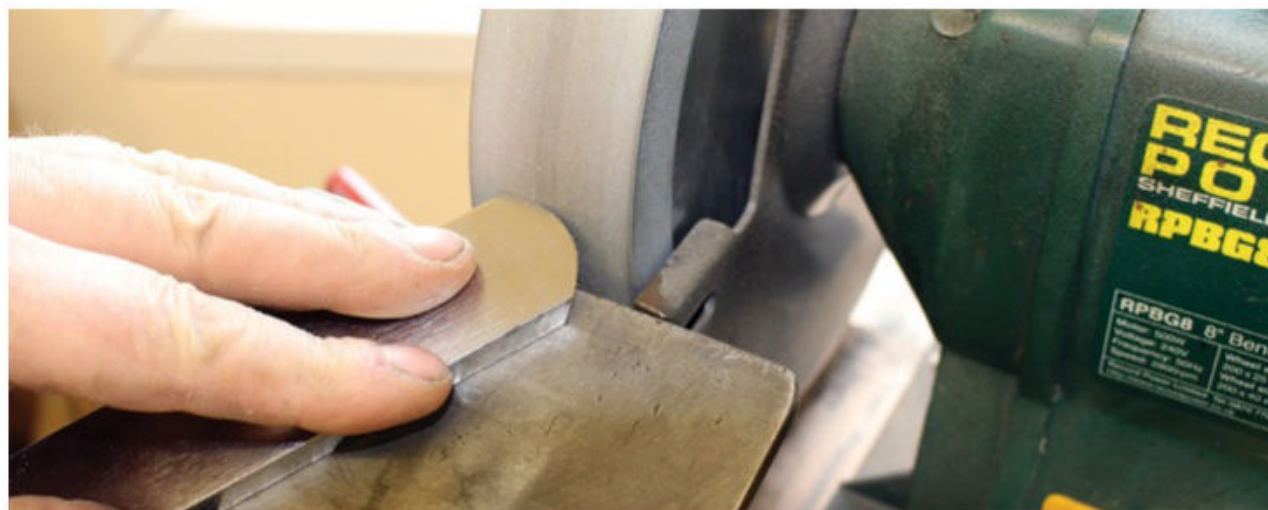
▲ The tool on a supporting table with the cutting edge uppermost to the oncoming wheel.
