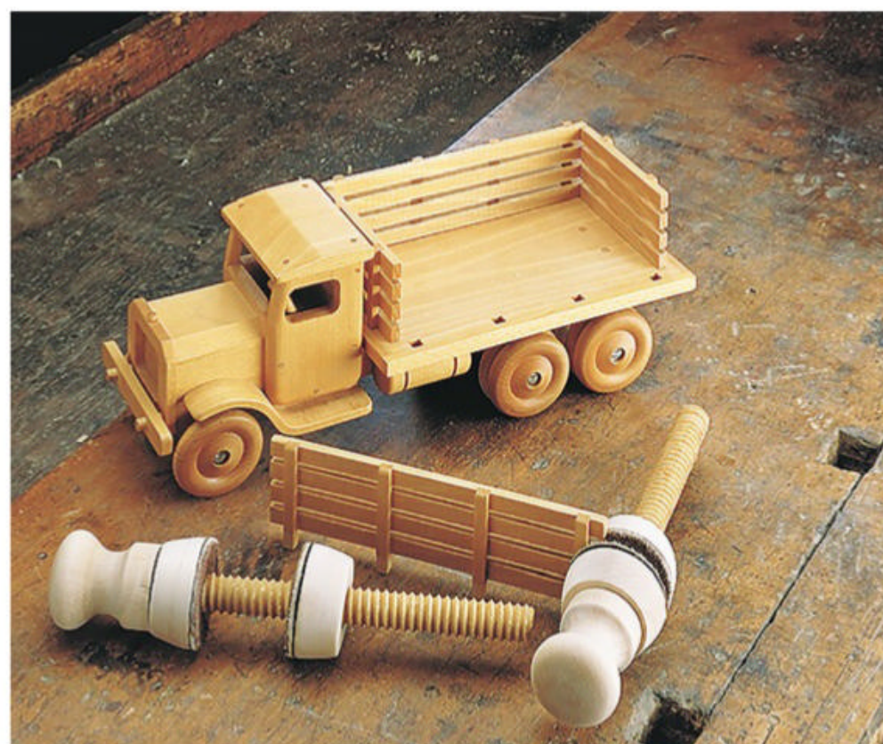
▲ Small-Piece Clamps. Cutting small wood threads are ideal for small, delicate work such as these micro clamps. Just thread a short dowel and then tap threads in the lower nut.
