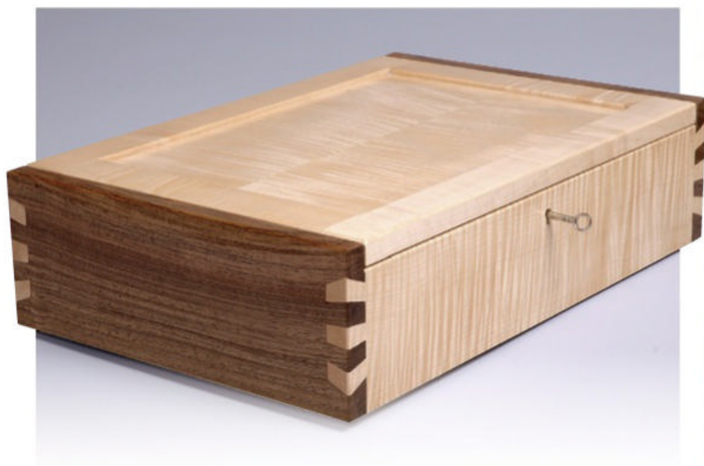
▲ Twisted Dovetails. John Bullar shows us how to make this unusual but useful joint. He takes you through the steps starting on page 36.
