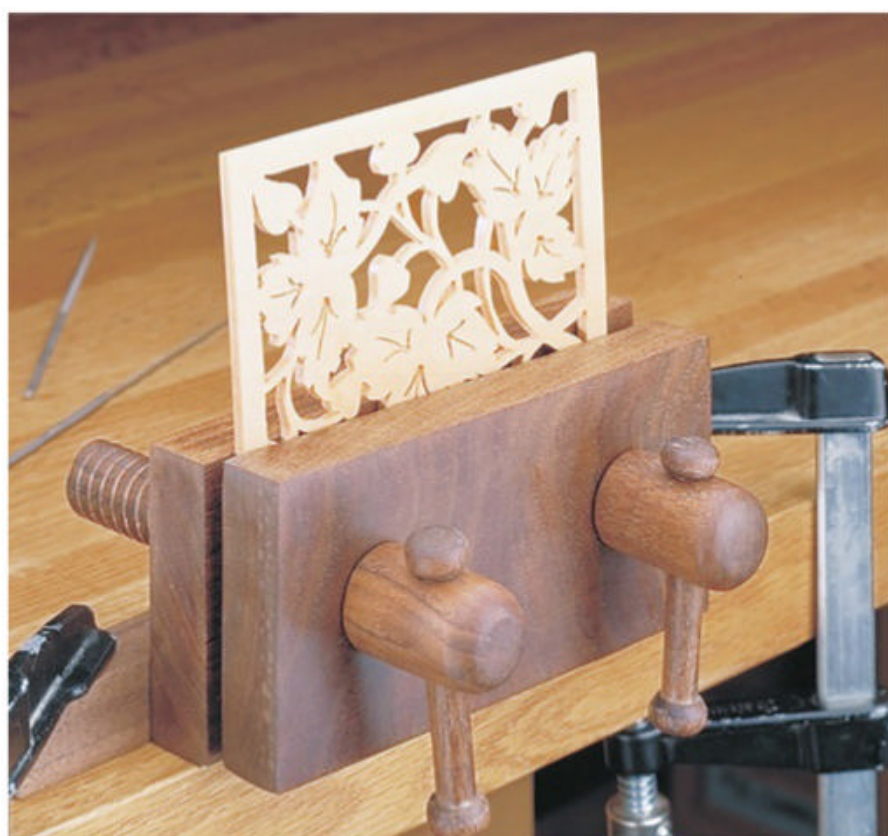
▲ Benchtop Vice. The twin wood screws on this small, benchtop vice thread into tapped holes in the back jaw. Apply a couple of oversized caps and handles for a functional benchtop vice.
