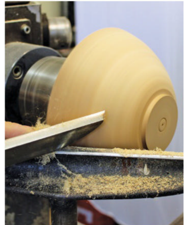
▲ Curved scraper used in shear-cutting mode.
