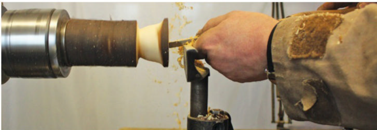
▲ Round-nosed scraper hollowing out a yew goblet.
