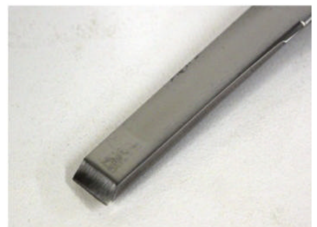
▲ Modified straight scraper.
