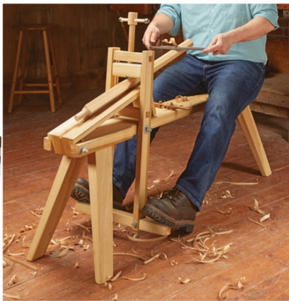
▲ Multi-Function Shavehorse. No, this isn't a woodworking rowing machine! This traditional device helps you get the most from your hand tools. Step-by-step instructions start on page 42.
