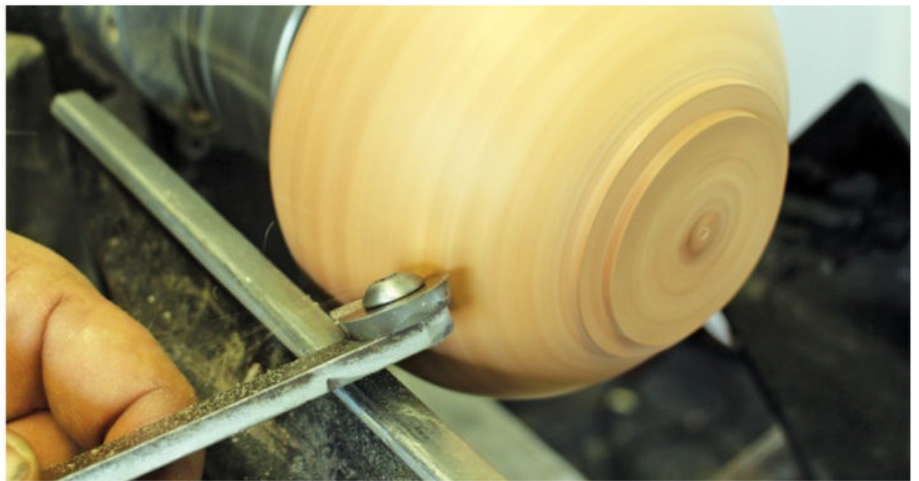
▲ Multi-head scraper used in shear-cutting mode.
