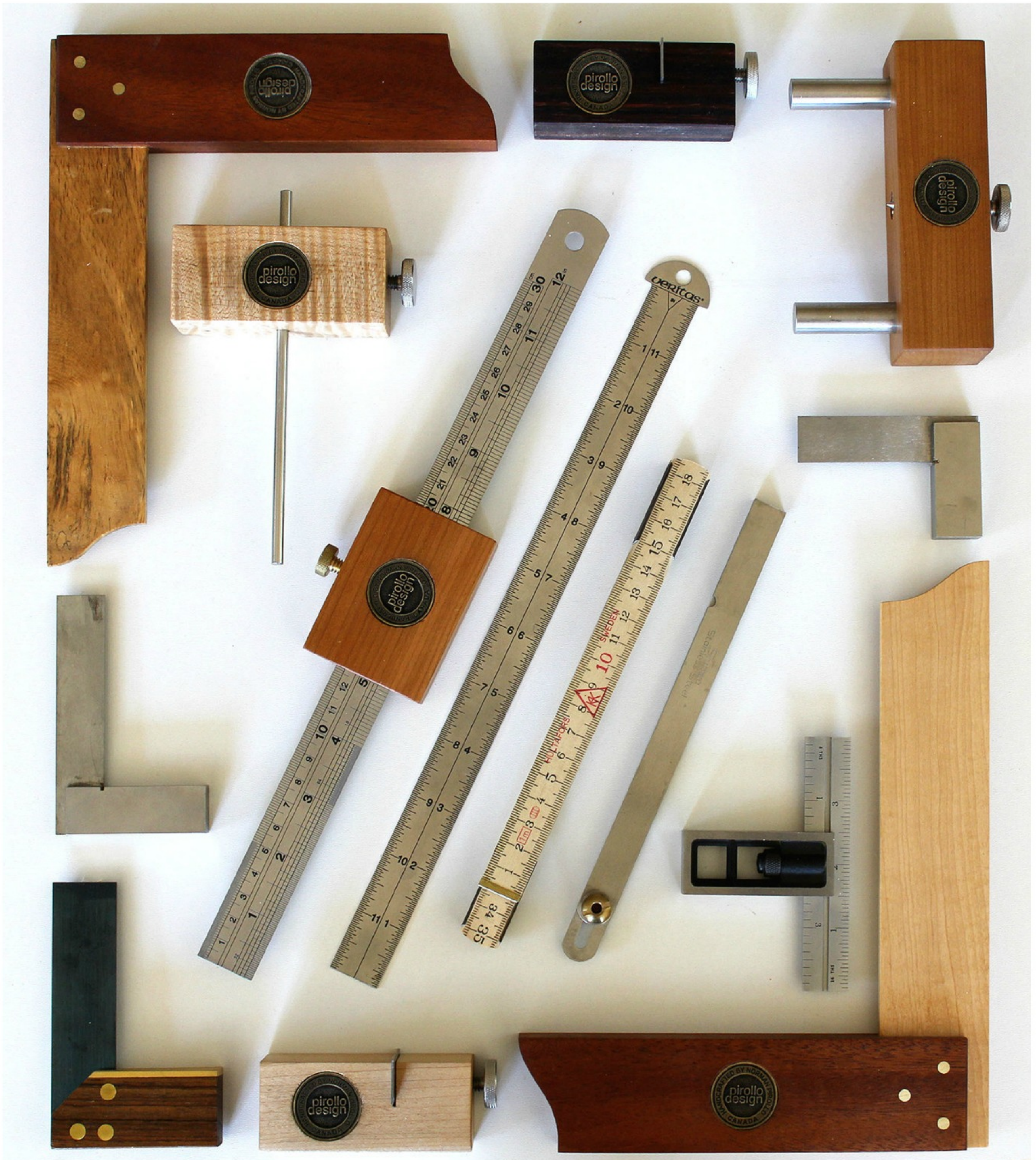
Various measuring and squaring instruments used in woodworking and furniture making. Image framed with two traditional wood try squares. Center finder tool, beading tools, various squares, depth gauge, sliding bevel gauge, and measuring instruments shown.
