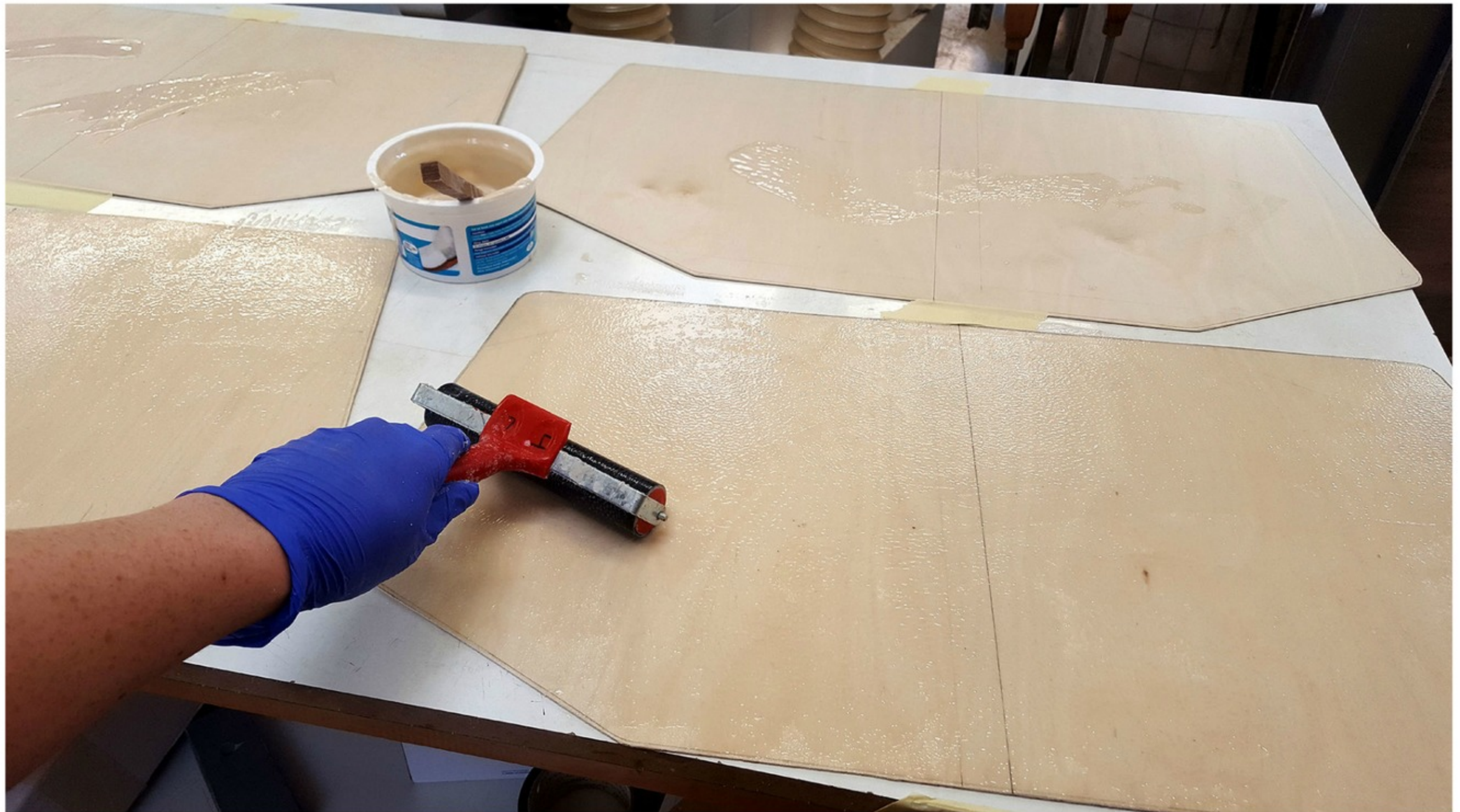
Applying glue to laminate layers using a glue roller
