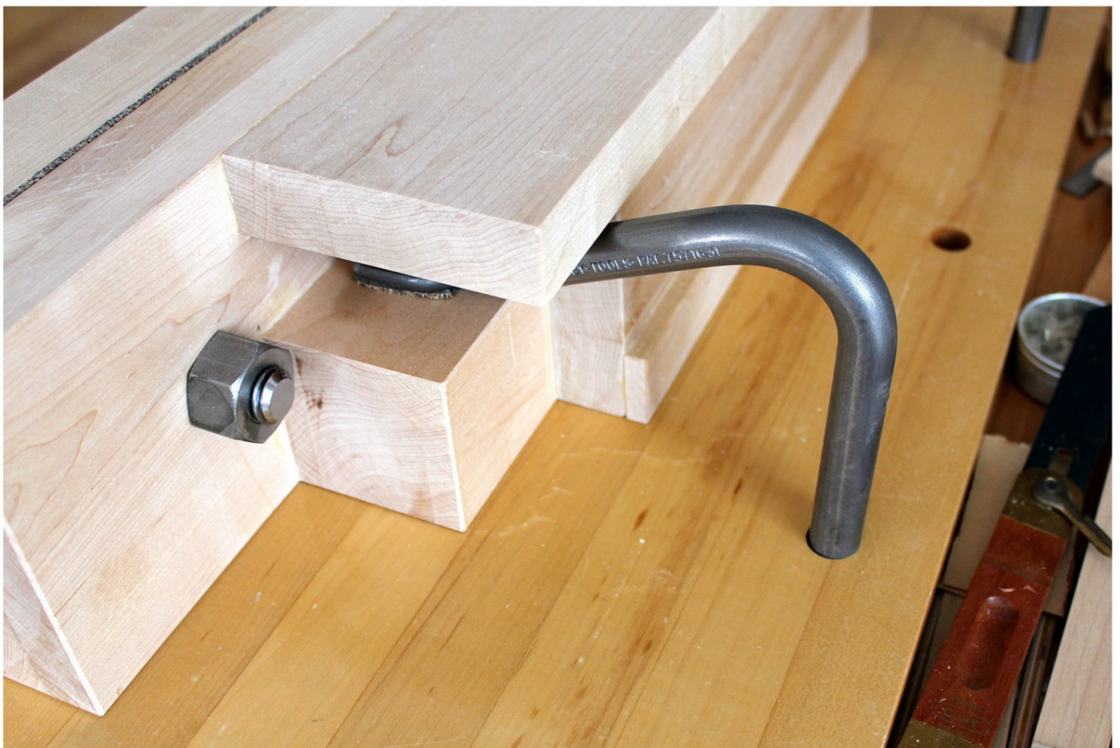
Photo of rear of Moxon vise with extra hardwood strip, table and table support
