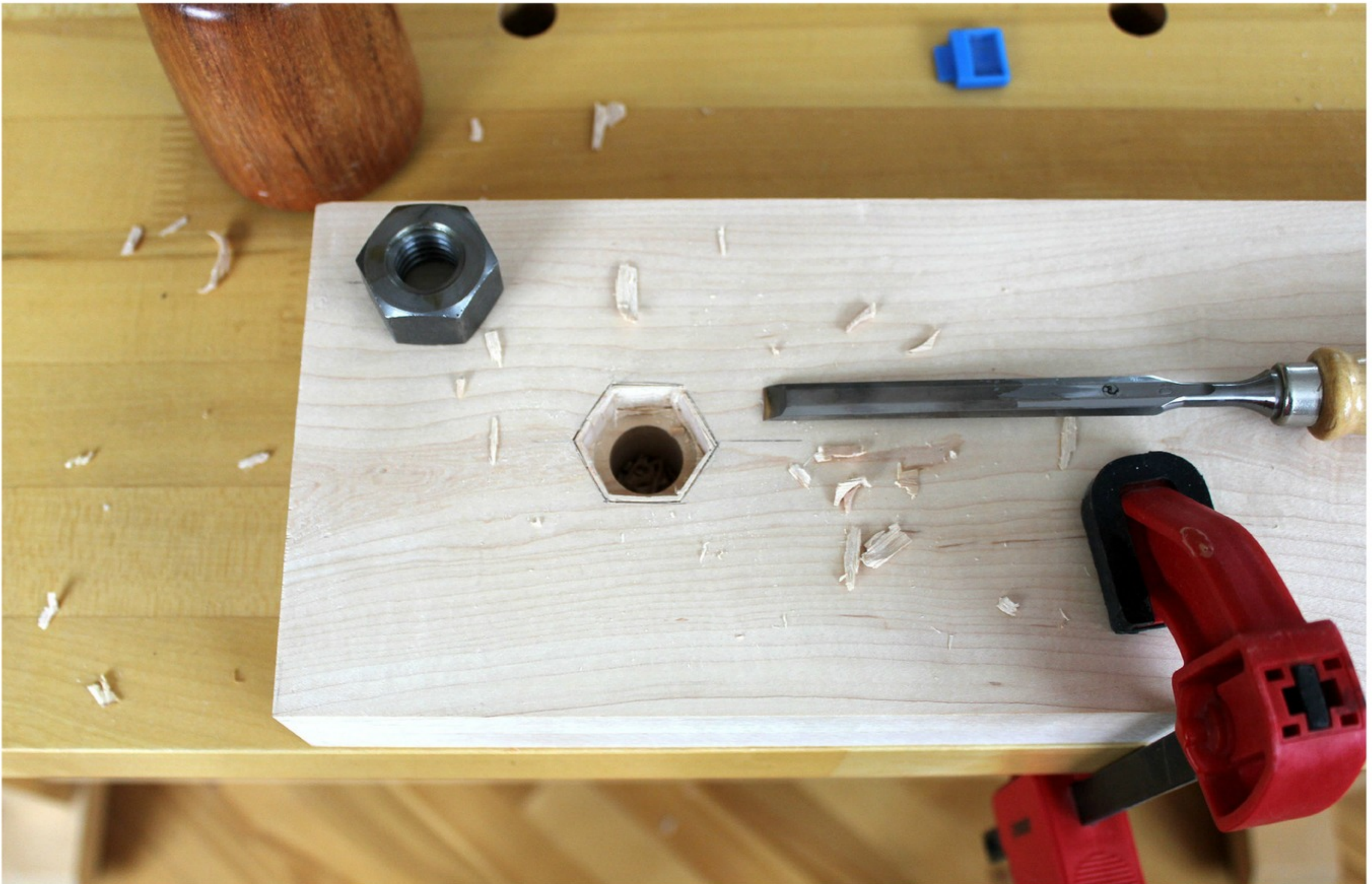
Mortise for captive six-sided nut created using bevel-edge and mortise chisels
