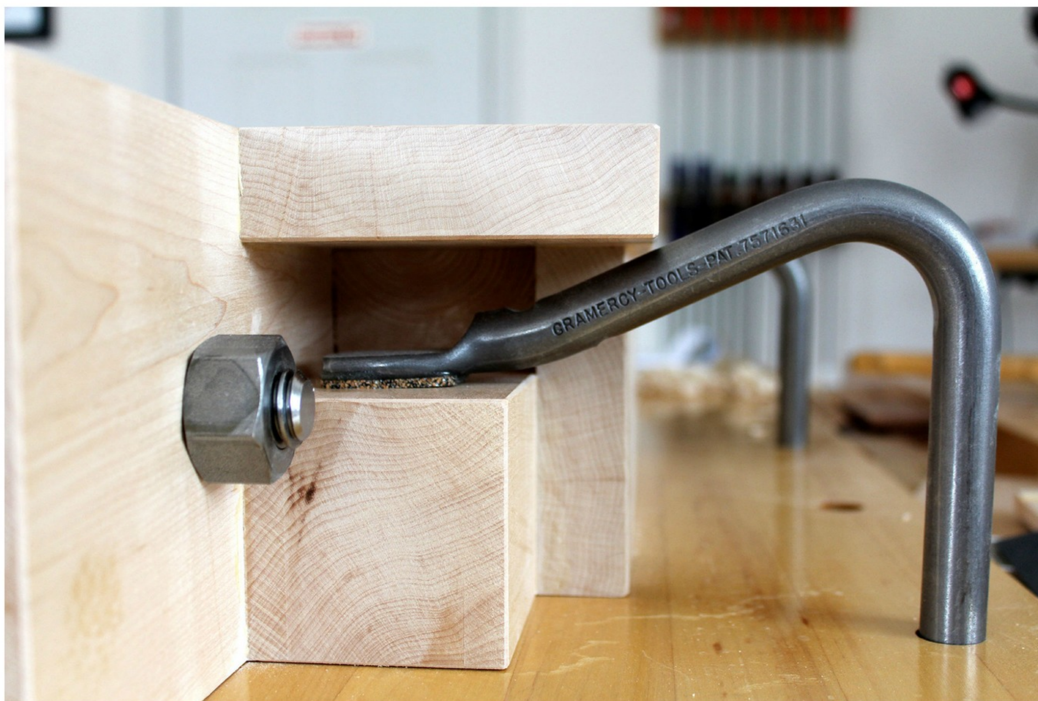
Photo of rear of Moxon vise with additional table support beneath table
