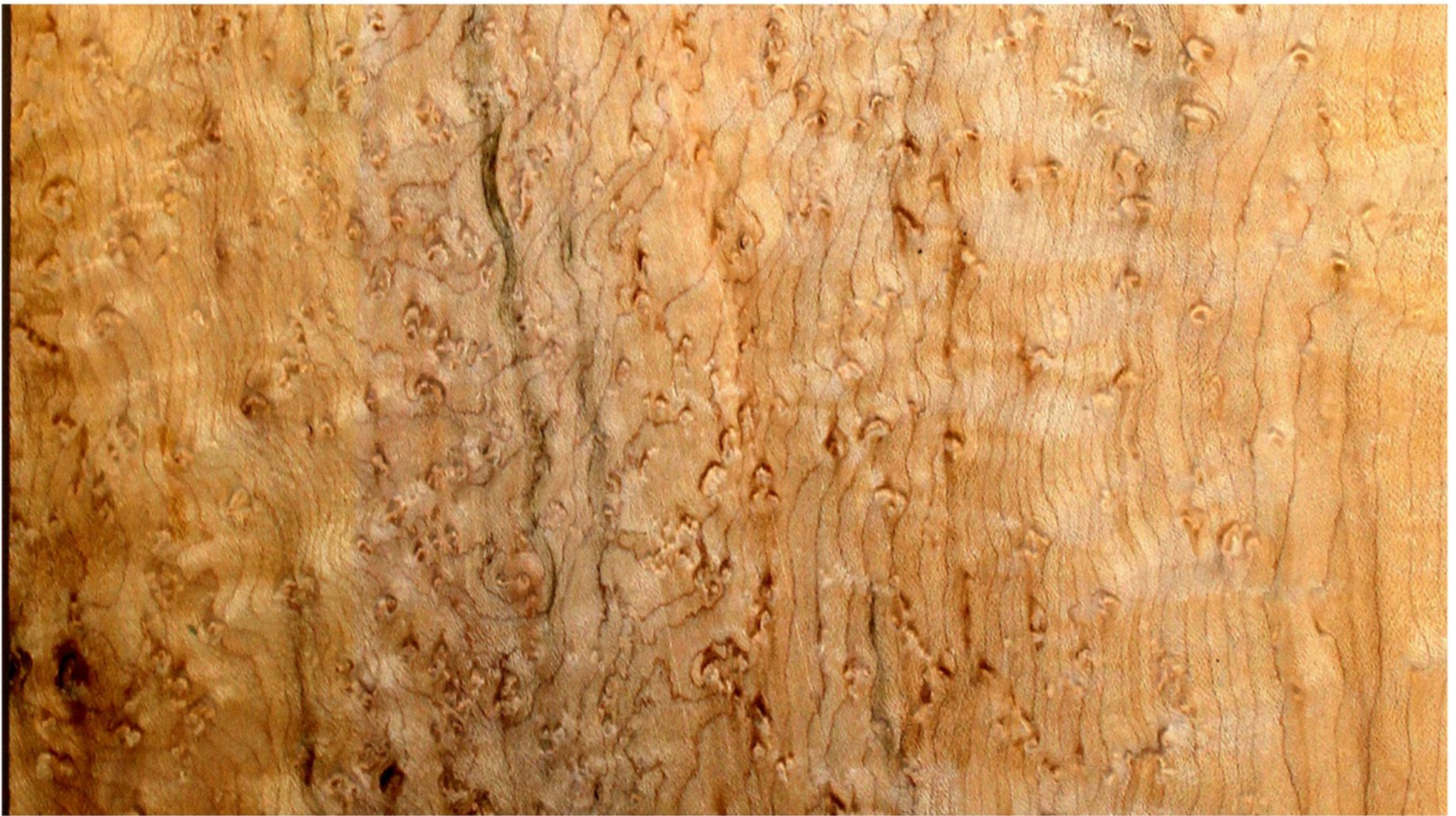
Highly-figured Bird's Eye Maple board exhibiting dense bird's eye figure
