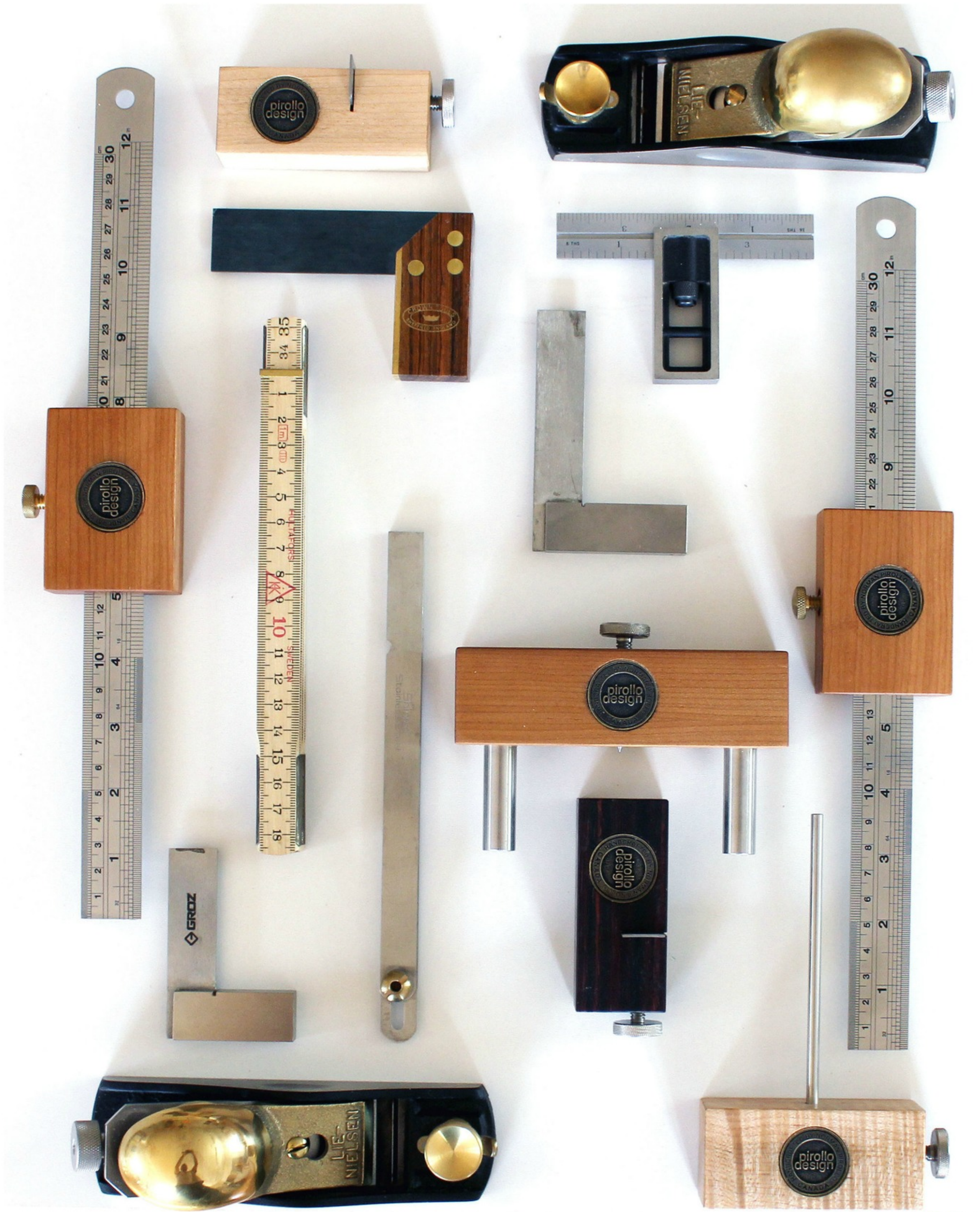
Various measuring instruments used in woodworking and furniture making. Image framed with two block planes, a low angle and standard angle. The block planes are intrinsic to hand work and very versatile in their application. Center finder tool, measuring tool, various squares, sliding bevel gauge, folding rule, beading tools, depth gauge are seen above.
