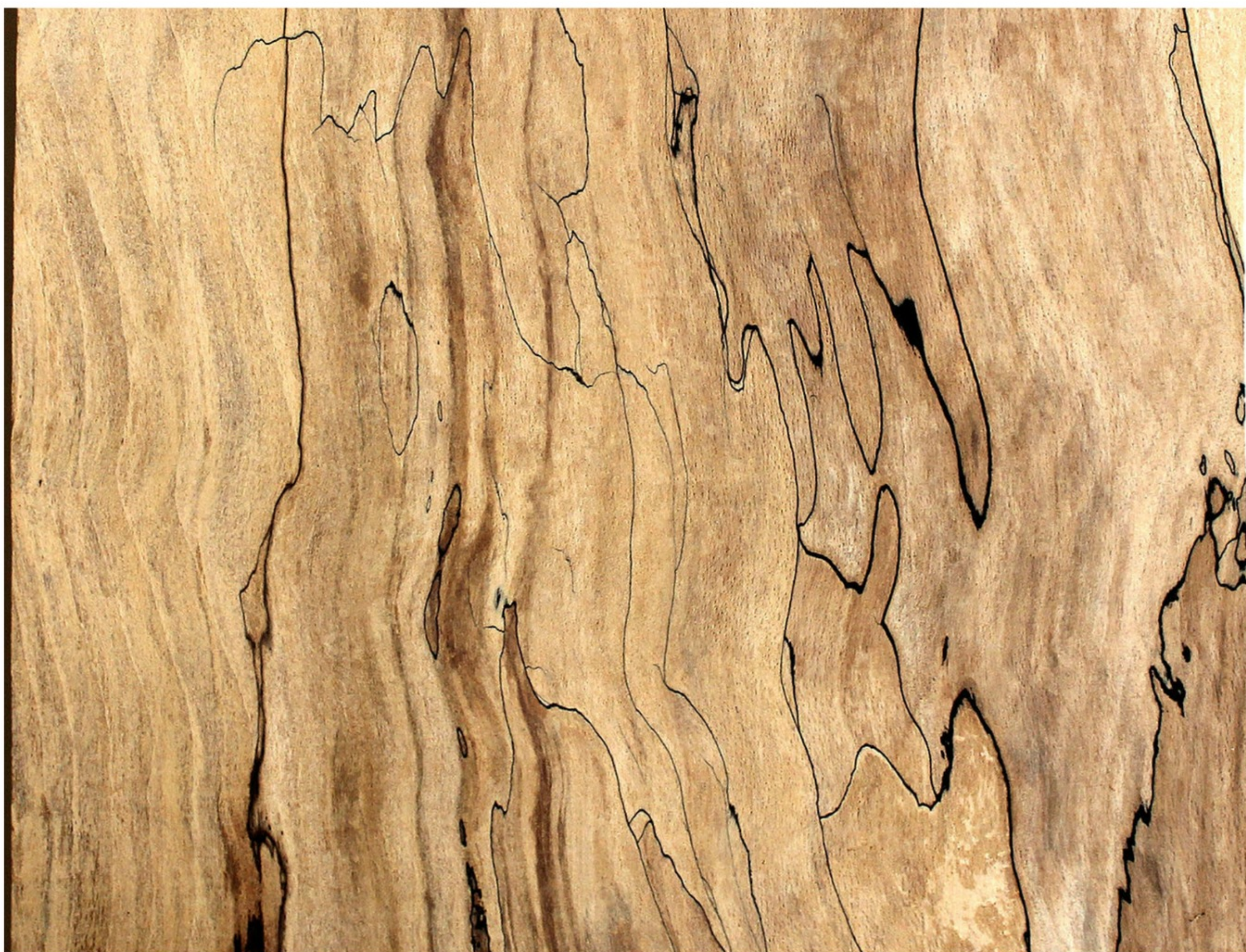
Ambrosia maple board with spalted surface and colored bug trail
