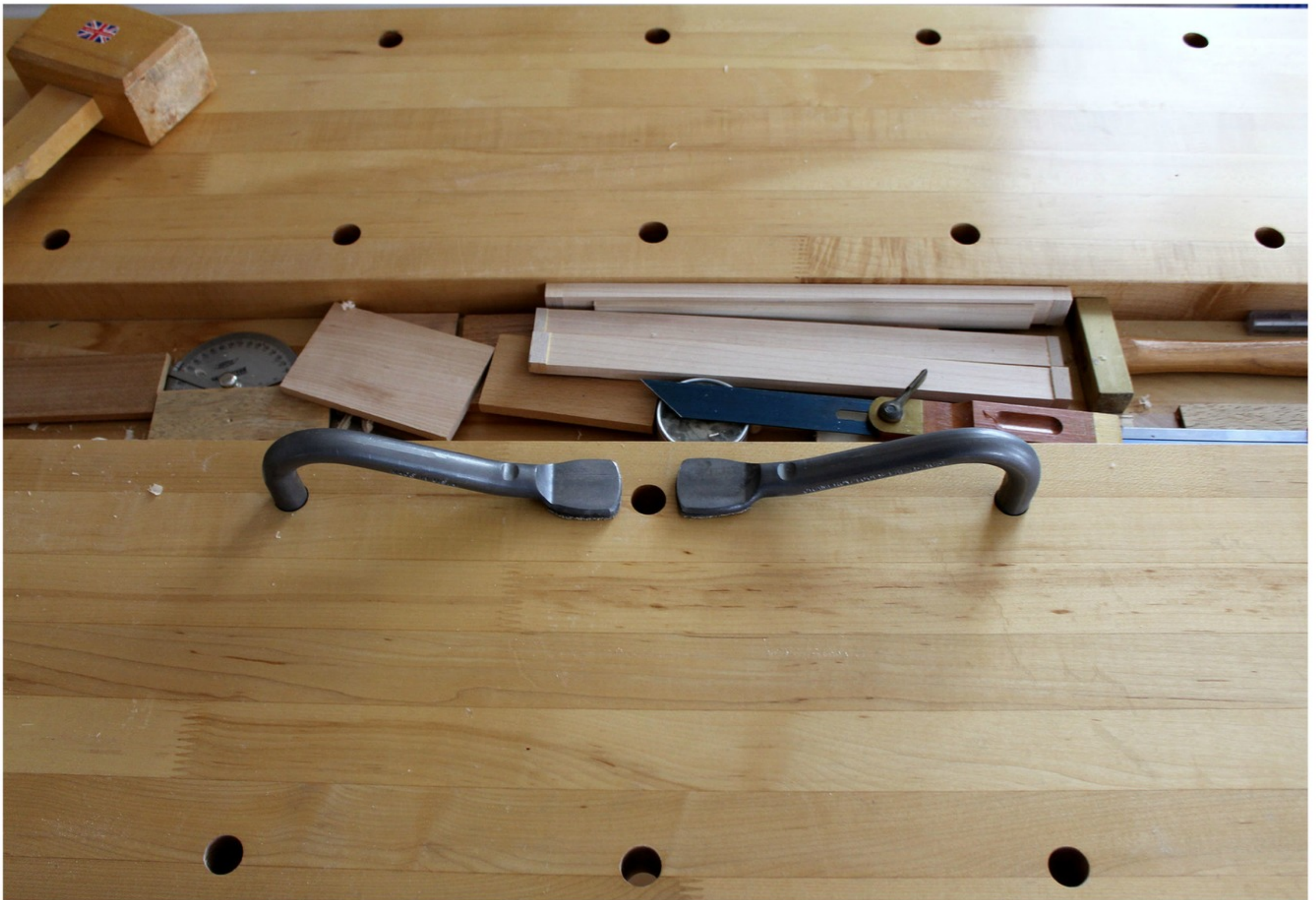
Holdfasts are inserted into dog holes of workbench top
