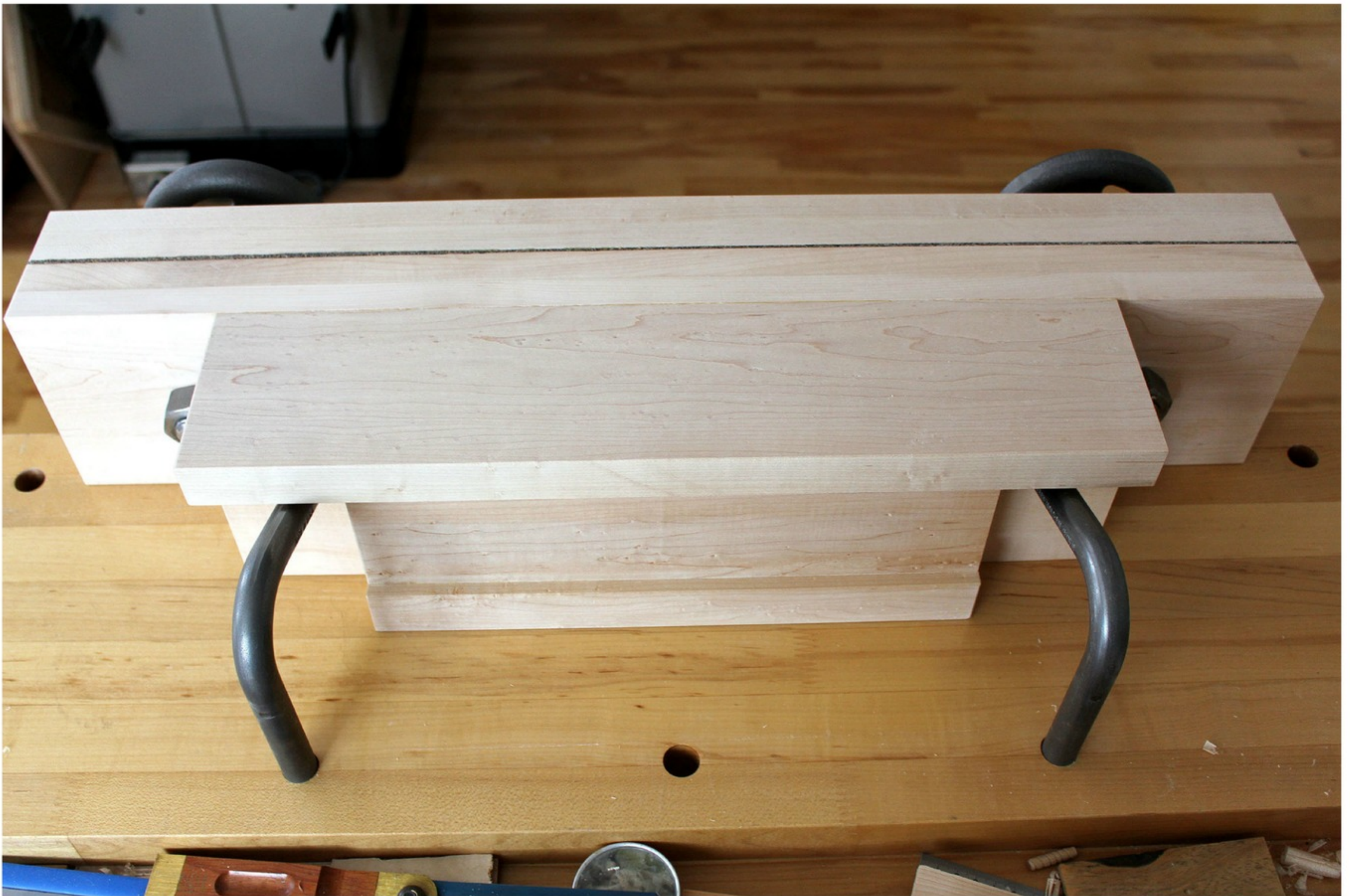
Rear view of completed Moxon vise with addition of hardwood strip to keep the vise square when placed vertically against a wall as shown below.
