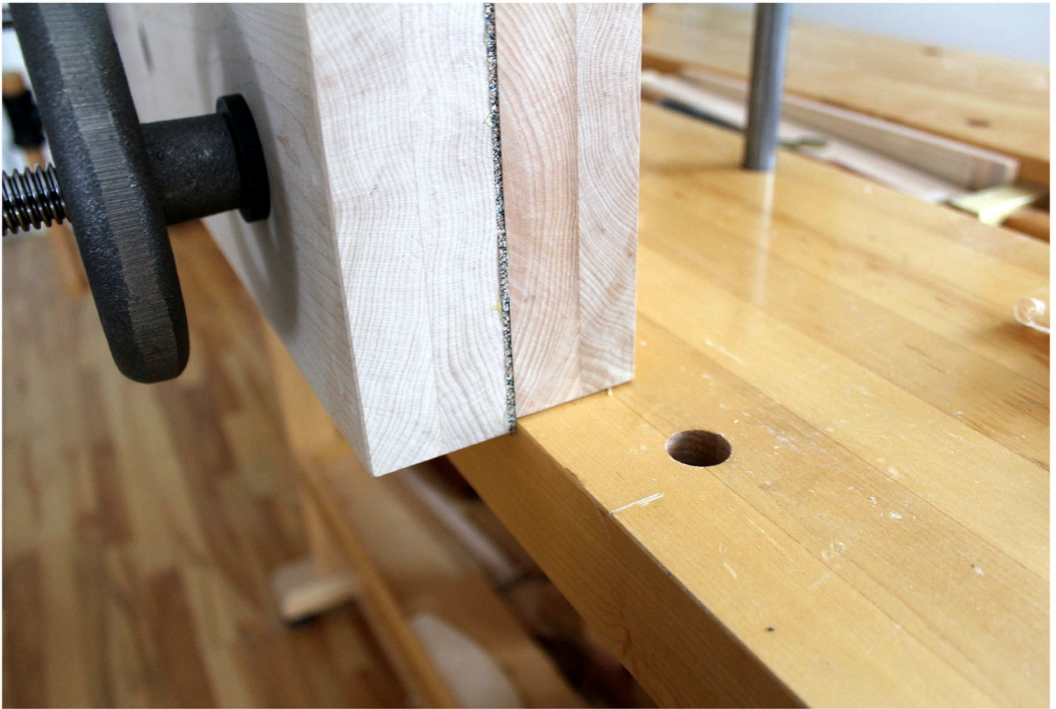
Wider front jaw sitting below workbench surface, registering closed vise to workbench top
