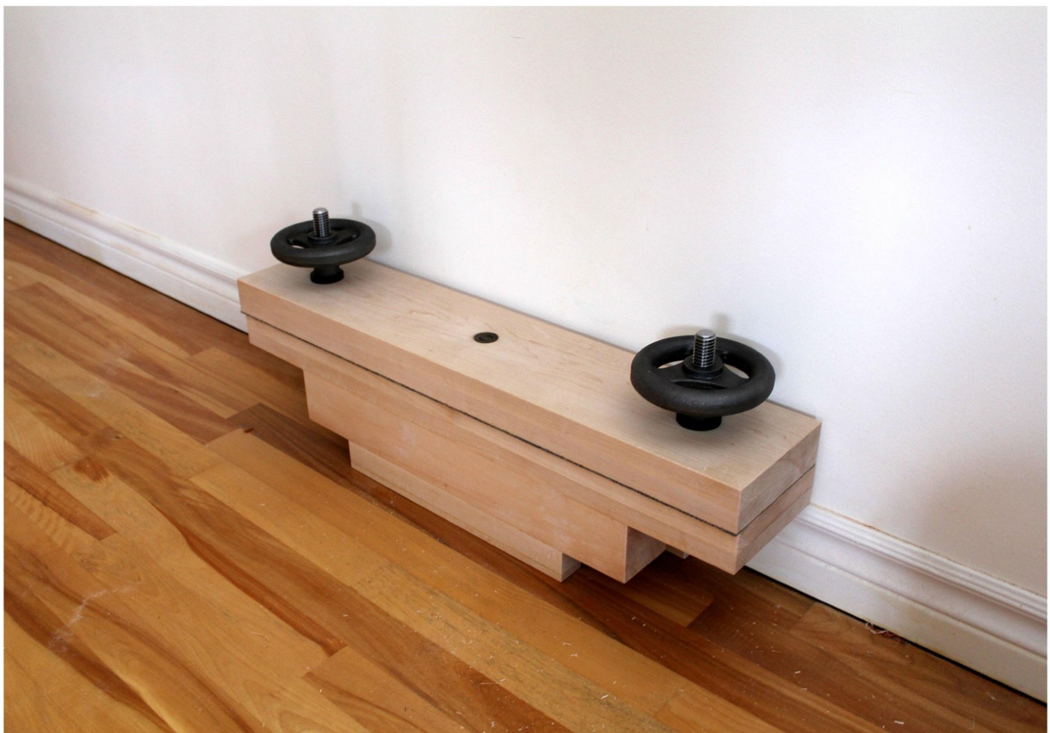
Rear view of completed Moxon vise with addition of hardwood strip to keep the vise square when placed vertically against a wall as shown below.
