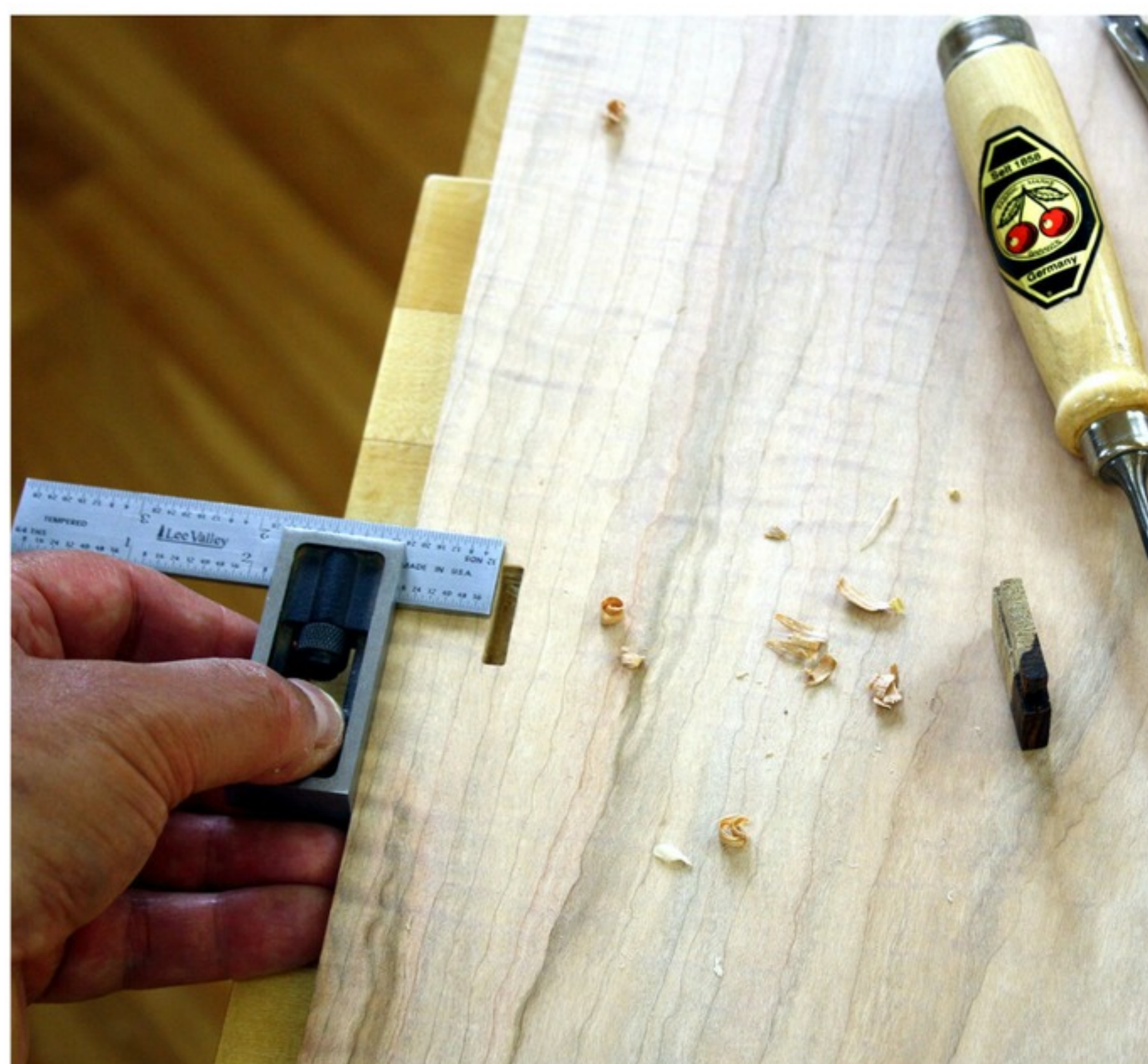
Marking & creating mortise for custom door pull
