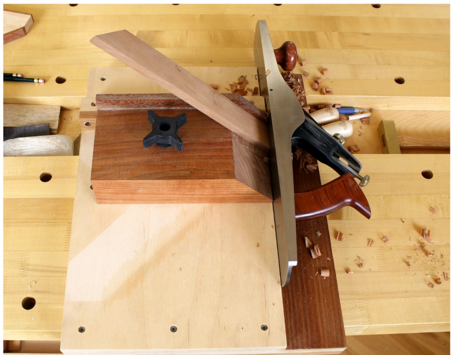
SHOOTING BOARD WITH EDGE MITER ATTACHMENT
