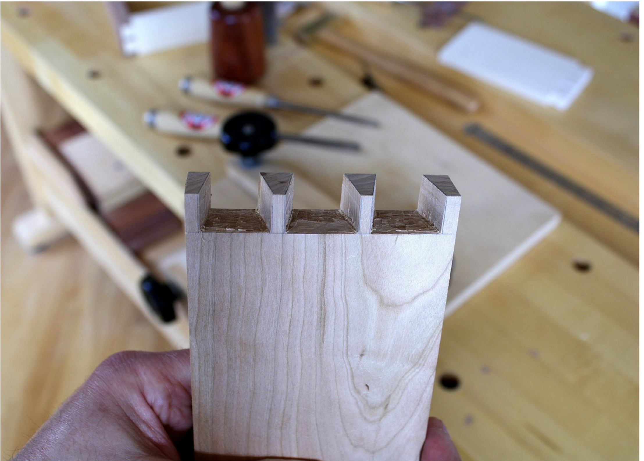
Cleaning and tuning the pins above, completed dovetail joint below
