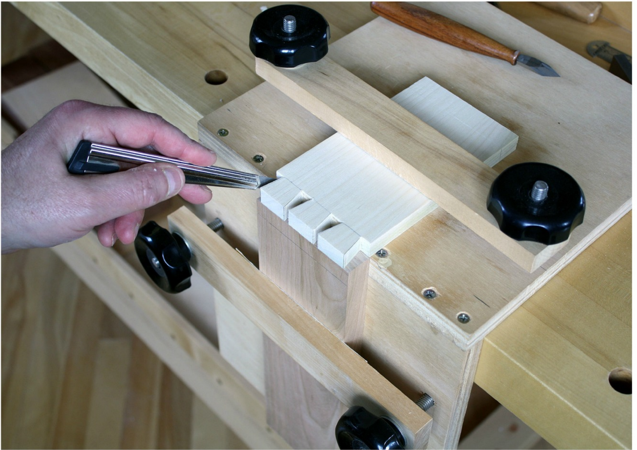
Transferring and marking the tails to the pin board above, sawing the pins below
