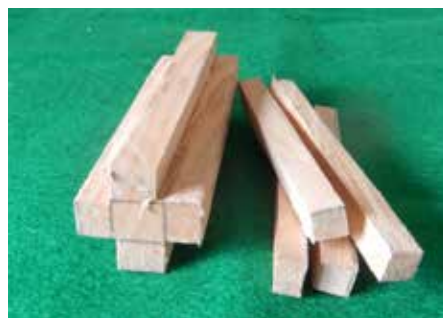
The piece of wood cut into a cross-shape. The four off-cuts (110x10x10mm) shown beside it
