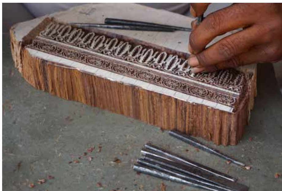
Block wood carvers in Jaipur, notice the small chisels and the fact they are carving into the end grain.
